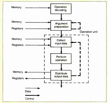
Figure A: Simplified processor flow. These several steps of machine-instruction execution may vary depending on your machine and the instruction.
