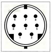
Figure 1: DIN-8 connector pin-out diagram.
