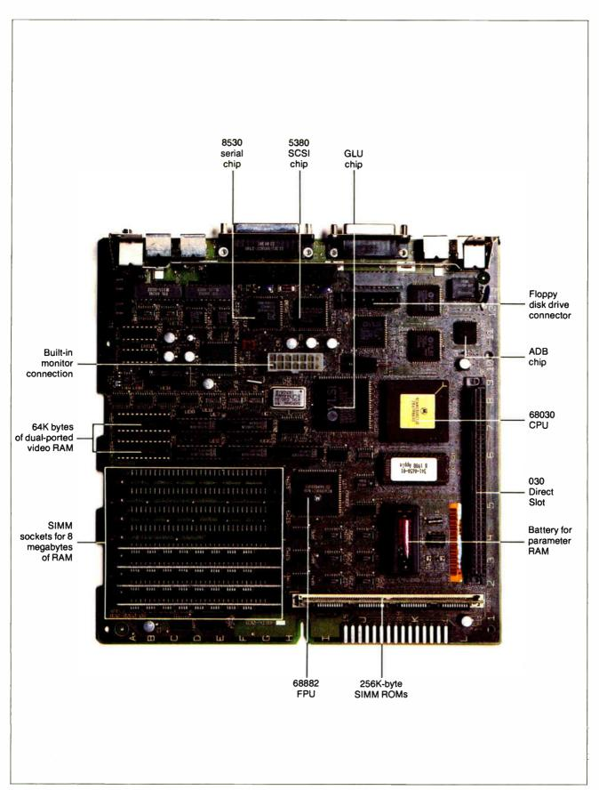
**Photo 1:** The new Mac SE/30 logic board features a 16-MHz 68030 CPU and a 68882 FPU. There's only one floppy disk drive connector on the board (the Mac SE has two). Note the SIMM-mounted ROMs and the 030 Direct Slot. Also note the 64K bytes of video RAM just above the SIMM RAM.
