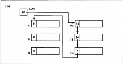
Figure 2: Once DELETE\_KEY has removed the associated key, deleting an entire record set is simply a matter of attaching the set to the available-for-reuse list.
