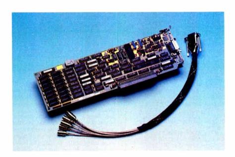
new generation of devices for the Macintosh promises to do for data input what the Laser-Writer did for output. One such product is Data Translation's QuickCapture package (\$1139), consisting of a video digitizer board (or "frame grabber") and software for the Mac II.
