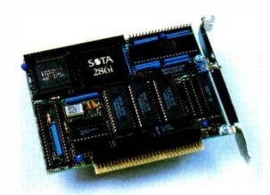
What's going on here is the 286i running the programs with no wait states on most read and write cycles.
