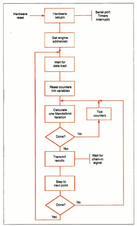
Figure 4: The flowchart for the program executed by each processor of the Mandelbrot engine.
