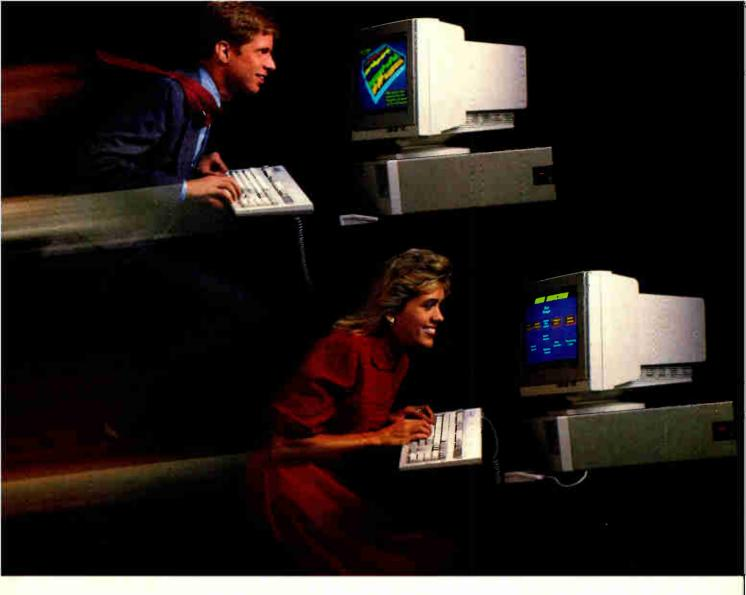
The 386/20. It's made for those who want to fly to the outer limits. With an Intel 80386 microprocessor operating at 20 MHz (with zero wait states) it'll move through the most complex applications with astounding case. And you won't have to worry about running low on memory either. It not only features 1024KB of RAM and a 1.2MB floppy disk drive, it also has a 64KB cache memory. Naturally, it comes equipped with serial/parallel/game ports and a 104-key keyboard, too.
