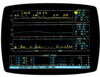
The Chromatography Data System displays data in real time.
