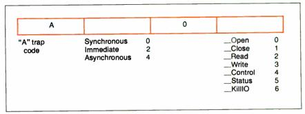
Figure 2: Device Manager trap word. Notice the seven possible traps and the three ways—synchronous (normal), immediate, or asynchronous—in which each can occur.
