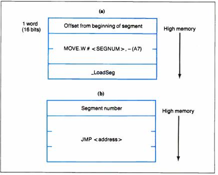
Figure 1: A Macintosh jump-table element for (a) an entry point whose segment is not currently loaded and (b) an entry point whose segment is loaded.
