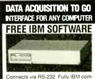
patible. Built-in BASIC. Stand alone capability. Expandable. Battery Option. Basic system: 16 ch. 12 bit A/D, 2 ch. D/A, 32 bit Digital I/O. Expansion boards available. Direct Bus units for many computers.
