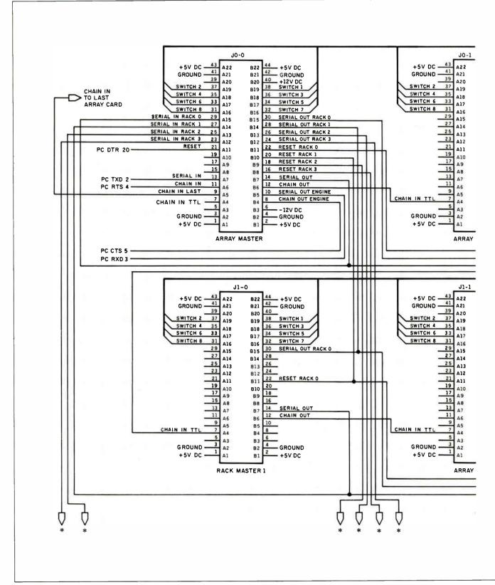
Figure 3: The complete schematic (sans buffers and support chips) for the Mandelbrot engine, detailing how the processors are chained together.
