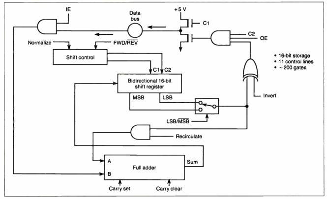
Figure 5: The Accumulator wafer type.
