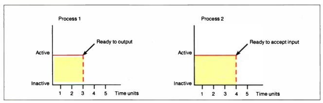
Figure 4: When process 1 must wait for one time unit before process 2 is ready to accept its data, it is said to be "blocked." Processes synchronize only when they communicate via Occam channels.
