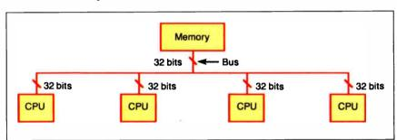
Figure 1a: A typical shared-memory multiprocessor (without contention memory cache). The bus is a common resource among all CPUs; as more CPUs are added, bus contention can lead to the von Neumann bottleneck.
