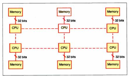
Figure 1b: A typical multicomputer system. Each node consists of a CPU and memory. Processes communicate with each other through bidirectional serial links (dotted lines).
