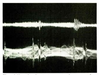
Photo 4: Normal-mode noise (top trace) and common-mode noise (bottom trace) after the insertion of an on-line UPS. The top trace contains a small amount of noise from the UPS's inverter. The bottom trace shows inverter noise superimposed over the common-mode noise present in photo 3. As you can see, the UPS has contributed to, rather than eliminated, common-mode noise.
