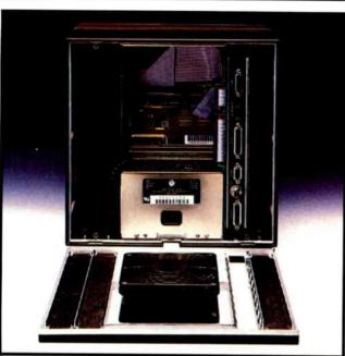
Photo 4: The inside of the cube. At top center is a bay for an additional full-height peripheral; at center is the magneto-optical drive. The power supply is at the bottom. To the right of center is the main CPU board.
