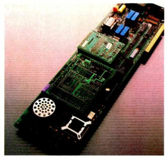
Connection Coprocessor multitasking board from Intel.
