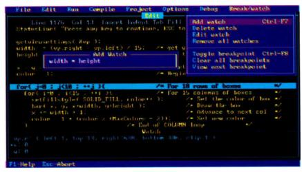
Debugging in the Turbo environment: shown here an expression is being added to the Watch window in Turbo C. The Execution Bar highlights the next line the debugger will execute.
