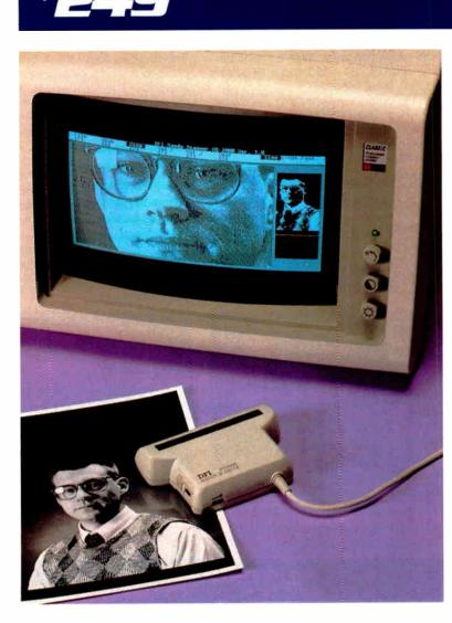
The DFI Scanner HS-3000 is a hand-held scanner designed for PC compatibles that scans images up to 4.1" wide. It's so easy to use just roll it over an image and display it on your screen it's that simple!
