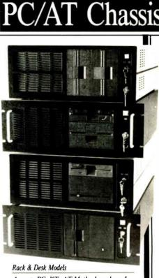
Accepts PC, XT, AT Motherboards and Passive Backplanes Doesn't Look Like IBM Rugged, Modular Construction Excellent Air Flow & Cooling Optional Card Cage Fan Designed to meet FCC 204 Watt Supply, UL Recognized 145W & 85W also available Reasonably Priced
