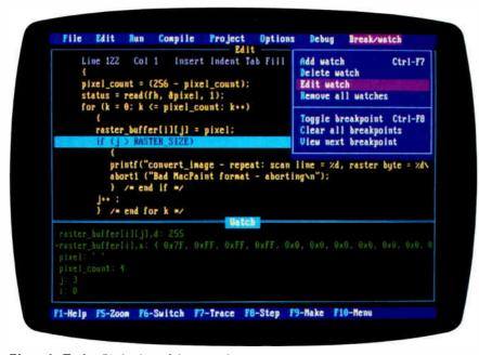
**Photo 1:** Turbo C's built-in debugging facilities highlight the statement being executed. At the bottom, you can see variables that are being "watched" and their contents. You can examine the contents of an array row, or an individual cell in the array. Also note that you can specify the output format of the displayed data.
