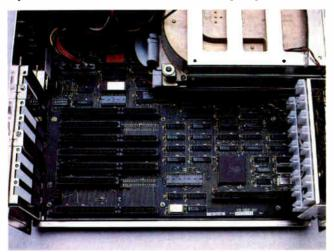
Photo 3: The popular Micronics 08-002-201 motherboard found in 6 of the 20 review machines (the Blackship 386 is shown here). the price of a chip set is far less than the price of an expansion card. All machines also include battery-backed clock chips.
