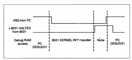
Figure 3b: A timing diagram showing the system's "gentleman's agreement" for controlling access to the debug RAM.
