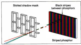
Figure 1d: Close-up of a rectangular-holed, striped-phosphor shadow-mask arrangement.
