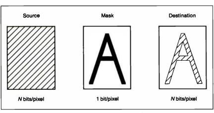
Figure 3: The three-operand PIXBLT. The third operand is a 1-bit-per-pixel array that provides a mask for pixel-by-pixel control over the destination pixels.
