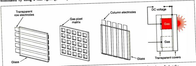
Figure 3: Gas-plasma displays use tiny pixels of gas to produce visible light. When sufficient voltage is applied at the intersection of two electrodes, the gas glows an orange-red.
