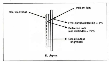
Figure 3: Unfiltered EL display reflections. An unfiltered EL display is a 75 percent-efficient mirror.
