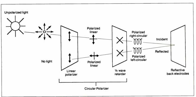
Figure 4: This diagram shows how unpolarized incident light can be controlled and its reflection eliminated by using a circular polarizer.
