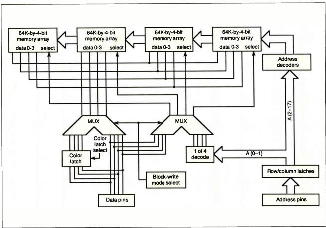
Figure 2a: TMS44C251 VRAM internals. Notice the four banks of 64K-by-4-bit memory, for a total internal width of 16 bits.
