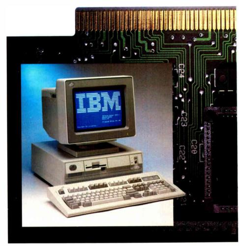
design, both companies' latest systems-IBM's PS/2 Model 70-A21 and Tandy's 5000 MC-feature a removable "processor card." Simply put, the computer's CPU components are mounted on a plugin board. Although neither company would talk about future plans, both admitted that the intent of this design is to enhance the performance of these systems at a later date by swapping the processor card.
