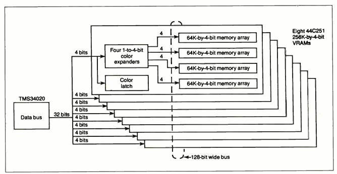
Figure 2b: An overall picture of the 44C251 and its connection to the '20. Notice how the '20 expands the 32-bit data path to 128 bits wide inside the VRAM.
