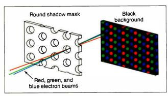
Figure 1c: Close-up of a round-holed shadow-mask and phosphor-triad arrangement.
