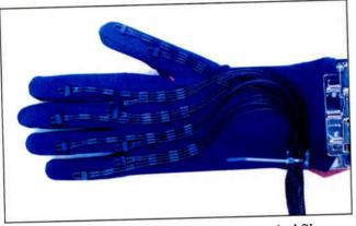
Photo 1: The DataGlove is a device that uses optical fiber sensors to measure and evaluate the range of joint movement, hyperextension, and abduction in the hand.
