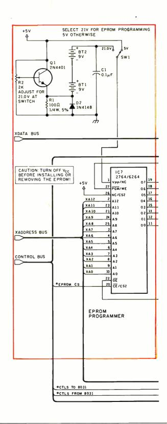
Figure 4b: The EPROM programmer subsystem and bidirectional bus buffers.
