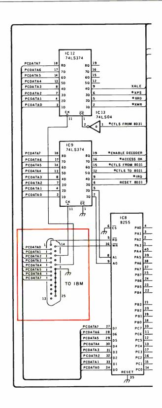
Figure 4a: The DDT-51 schematic, showing the PC interface and the debug RAM.
