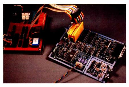
The DDT-51 is a low-cost IBM PC-based Intel 8031/8051 development system
