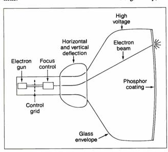
Figure 1a: Typical monochrome CRT operation. Negatively charged electrons are produced in an electron gun and are attracted to the high positive voltage at the front of the tube. The resultant electron beam is focused on and deflected across the CRT face.
