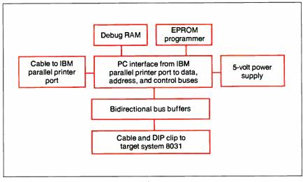
Figure 1: A block diagram of the DDT-51 development system.
