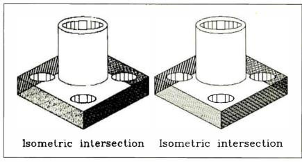
Figure 1: The image at left is an AutoCAD file that was printed on a LaserJet II and transmitted between standard fax machines. The image at right is the same file, sent between PC fax cards and output to the same printer.
