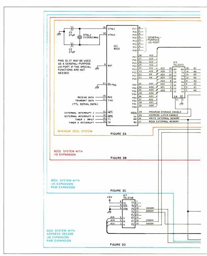
Figure 2: Growing an 8031 system. (a) A minimum configuration, (b) minimum system with I/O expansion, (c) system with I/O and RAM expansion, and (d) system with address decode logic and even more RAM and I/O.
