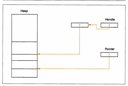
**Figure 2:** On the Mac, a pointer is a 32-bit entity that holds the address of a block of memory. A handle is a pointer to a pointer to a block. Notice that the system can relocate the upper block without altering the contents of the handle; not so with the lower block.
