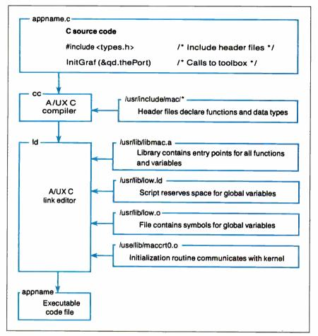
Figure 1: The steps involved in creating an A/UX application that uses the Mac ROM.
