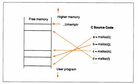
**Figure 1:** The 8088 version of BYTE Small-C handles memory allocation as an upward-growing stack tracked by the global variable \_Umemptr. Memory blocks (left) allocated by the source code (right) must be freed (using the free() function) in the reverse order to how they were allocated (i.e., the block that d points to must be released before the block that c points to). BYTE's Small-C for the Mac removes this restriction.
