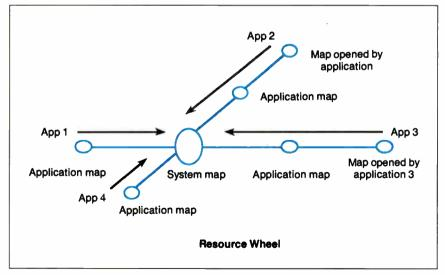
Figure 2b: A more efficient plan has been implemented using a resource wheel. The resource chain still exists for each application, but the plan adds the system heap as the hub of the wheel.
