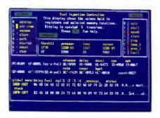
InSight Display. InSight blends analyzeremulator techniques to give you continuous, real time monitoring of key processor functions. And still services user interrupts. It displays changing register contents, I/O lines, ports, user-defined memory windows. With your own labels.
