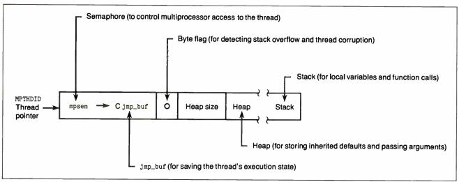
Figure 2: Internal representation of the thread data type.
