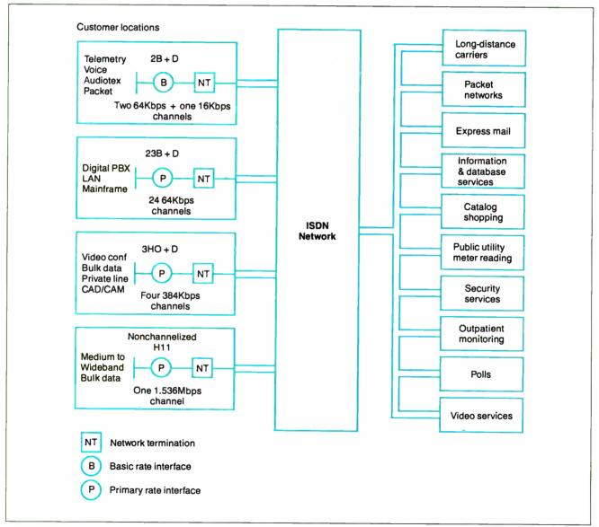
Figure 2: Many services will be available over ISDN's basic and primary rate interfaces when the technology is fully employed. Some of the potential applications are shown here.
