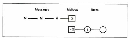
Figure 4: Mailbox "message bank." The upper diagram is of a mailbox with messages waiting for tasks (positive count); the lower diagram is of a mailbox with tasks waiting for messages (negative count).
