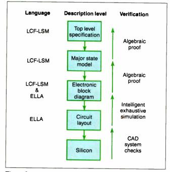
Figure 3: VIPER's hardware validation process uses a hierarchy of description levels.
