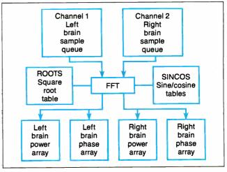
Figure 5: Main components of the FFT.
