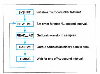
Figure 2: A flowchart for HAL's firmware program, BIO31.
