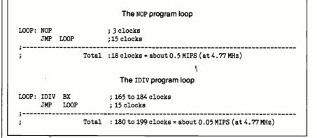
Figure 1: Why MIPS are meaningless. You could use either of these two code fragments to estimate MIPS on a machine, but their execution times differ significantly.
