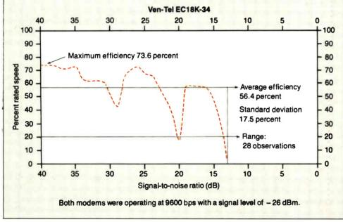
Figure 1b: The raw test results for the Ven-Tel EC18K-34 modem, a multicarrier unit, show that it operated with less efficiency but over a broader range than the Telenetics modem.
