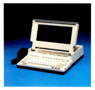
The system ROM contains the Phoenix BIOS, and the system software includes MS-DOS 3.2 and Tandy's version of GWBASIC 3.2. The system also contains a setup mode from which you can alter system parameters at any time. For example, the F7 option lets you change the system clock speed from the default 7.16 MHz to 4.77 MHz, if you should need to for program compatibility.
