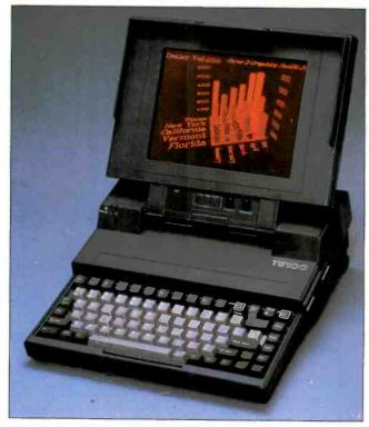
Toshiba's new portable is 80386-powered.
