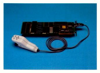
The TransImage 1000 is a product that relieves you of the burden of deciding between high functionality and low cost. The package contains three components: the TransImage scanner, the TransImage controller board, and software to make it all work. The controller board gives the scanner its power. It is centered on a Motorola 68000 processor and a series of custom logic chips.
