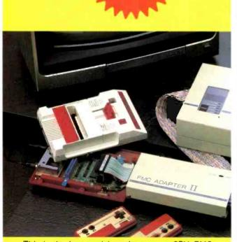
This is the key to debug the custom CPU FMC-2A03 of the FAMILY COMPUTER (Nintendo). All you need is this unit ! Then, you can debug and develop your software for the FAMICOM without much knowledge on hardware of the FAMICOM.
