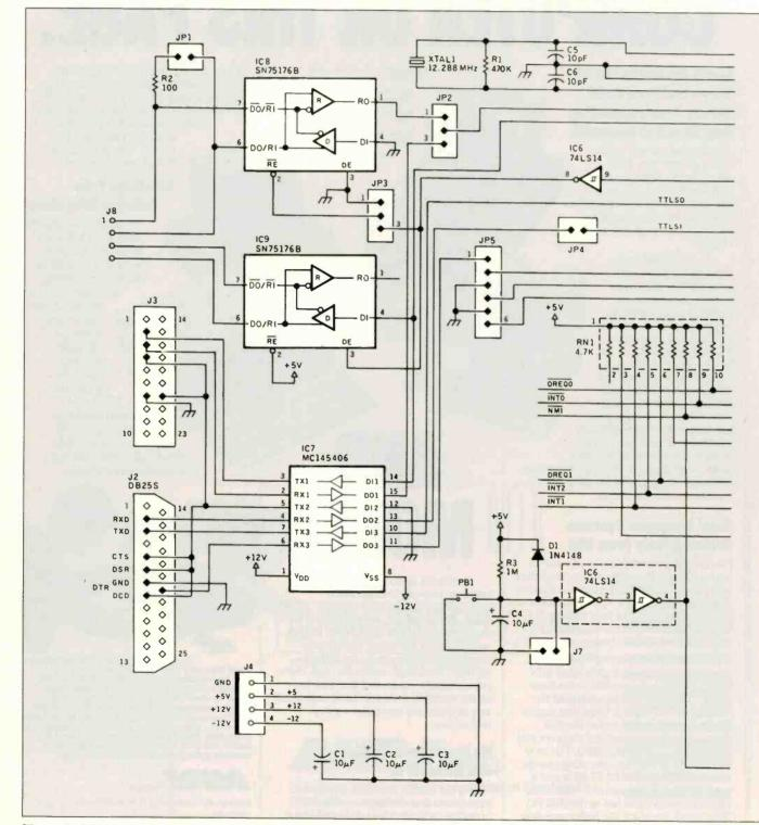
Figure 1: Schematic for the BCC180 computer/controller.
