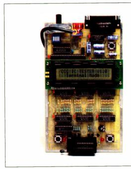
Photo 2: You can use the IC tester in stand-alone mode, provided you have attached the tester's optional LCD. The push-button switches in the upper right, lower left, and lower right control the tester's operation.
