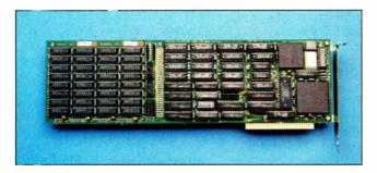
The PC-Elevator 386 is an unusual 16-megahertz 80386 addin board for the IBM PC, XT, or AT. The base unit (\$1995) comes with 1 megabyte of on-board 100-nanosecond memory, a socket for an optional 80387 coprocessor (\$795), disk caching and EMS (Expanded Memory Specification) memory management software, and a bus for attaching up to 16 megabytes of memory via optional daughtercards (\$2000 for each 4-megabyte daughtercard).
