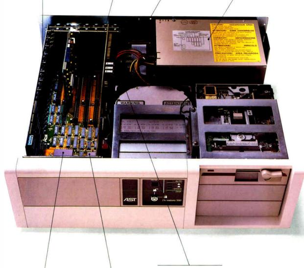
20 MHz, 80386 processor for high performance, AT-compatible desktop computing. Support for 80287 and 80387 coprocessors provides users with a choice for computation-intensive applications.
