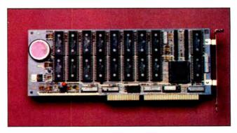
The Awesome I/O card is designed to improve the throughput, capacity, and reliability of your hard disk. Using on-board nonvolatile CMOS RAM (256K or 512K bytes, 100 nanoseconds) managed by an intelligent control unit called the Heuristic Adaptive I/O Controller, the Awesome I/O card determines and caches your most frequently used hard disk data.
