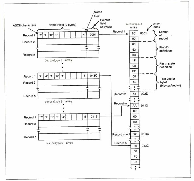
Figure 2: Illustration of the information storage in VECCPT. PAS's primary arrays.
