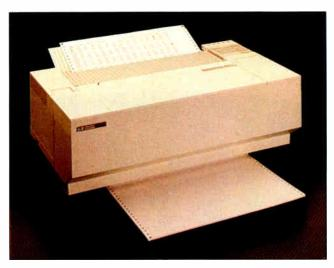
The 24-pin HP RuggedWriter prints at up to 480 cps.
