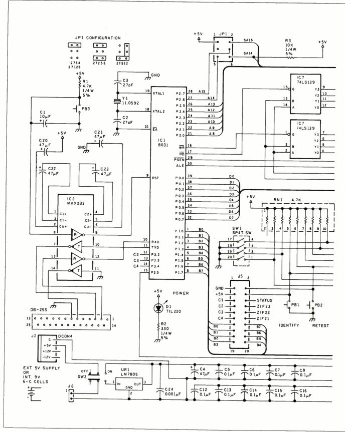
Figure 2: Schematic for the Circuit Cellar IC tester.
