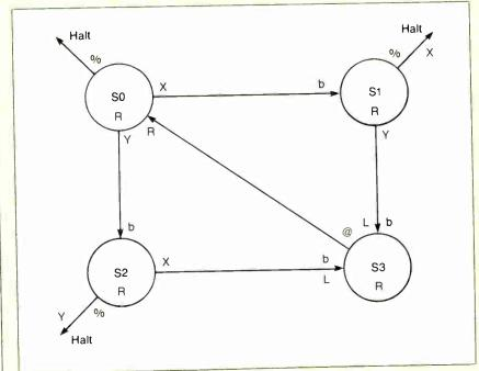
Figure A: A means of diagramming a Turing Machine, using the votetabulating TM as a base.
