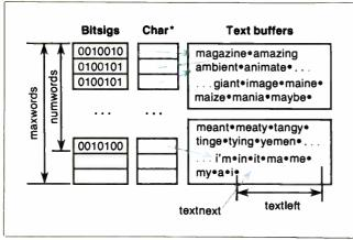
Figure 2: The "bit signature" data structure. This is a collection of fields, each holding the frequency of a given letter and an underflow bit. To simplify the algorithm (and to allow the use of arithmetic subtraction to do the subtraction of signatures), the author designed the structure so that frequency-count fields do not cross physical boundaries—longwords, in this case.
