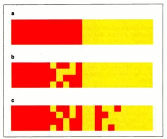
Figure 1: (a) Two adjacent blocks of color sharing a hard boundary. (b) The boundary in (a) has been softened with a yellow-filled airbrush. (Each square equals one pixel.) (c) In this case, the hard boundary in (a) has been softened by smudging (i.e., by swapping pixels).
