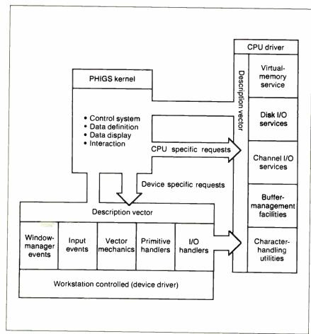
Figure 4: Figaro's CPU and device intelligence.
