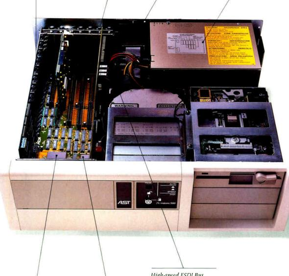
20 MHz, 80386 processor for high performance, AT-compatible desktop computing. Support for 80287 and 80387 coprocessors provides users with a choice for computationintensive applications.
