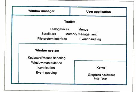
Figure 1: Window-system architecture. A window system provides a high-level interface between the application and the hardware.
