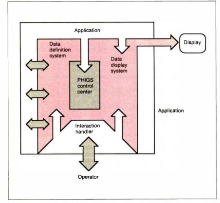
Figure 1: A block diagram of the PHIGS subsystem.
