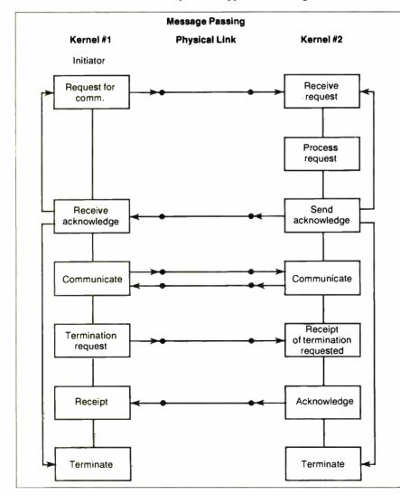
Figure 2: A model of the flow of the message-passing process.
