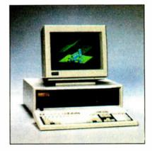
disk with less than 20-ms access time. The system comes with a 1.2-megabyte 54-inch floppy disk drive, and a 1.4megabyte 31/2-inch floppy disk drive is available as an option. Also available is a 135-megabyte internal tape drive that uses DC-600 tape cartridges.
