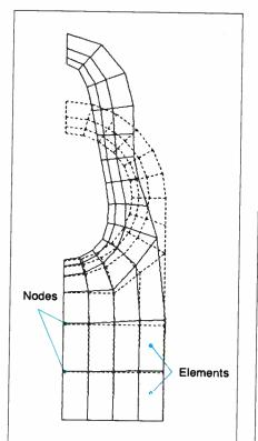
Figure 1: A half-symmetry finiteelement model of a steel lifting lug, used for lifting pressure vessels and other heavy objects, generated in MSC/pal 2.
