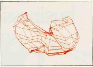
Figure 7: The matrix begins to define a two-dimensional surface as the number of points increases. Here, the number of defined points is 50.
