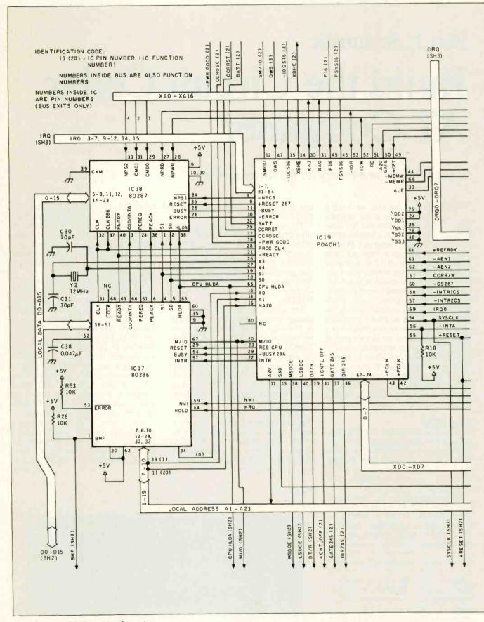
Figure 1: The CCAT circuit schematic.
