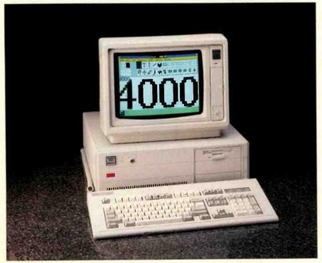
its standard configuration a 1.44-megabyte 31/2-inch floppy disk drive. Tandy happily points out that other types of disk drives-such as a 51/4-inch floppy-are available as options. The keyboard departs from the XT style used by the 3000 and looks very similar to the latest PC AT keyboard, complete with 12 function keys arranged horizontally, and LED indicators.
