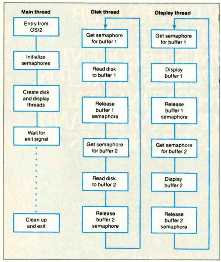
Figure 2: A sketch of program logic for the DUMP example program. Separate subprocesses (threads) are used to perform the disk file reads, and the formatting and display. Two semaphores provide mutual exclusion on the I/O buffers. The main thread simply waits until the other two threads are done, unless a critical error or other external event activates it in the meantime.
