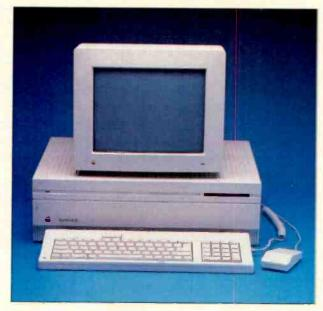
cess, as opposed to the 16-bit data path and 24-bit bus on the other Macintosh systems. The combination of doubled clock rate and doubled data path give roughly a fourfold increase in performance over the Mac Plus.
