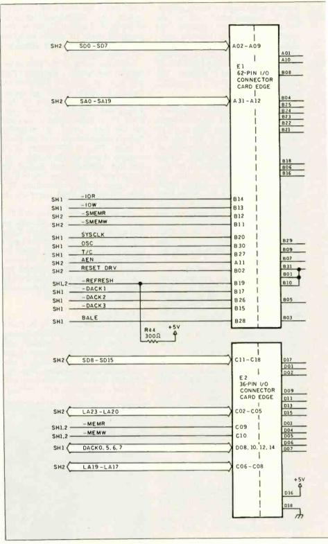
Figure 2: Edge-connector pin-outs for the CCAT.
