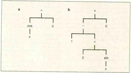
**Figure 1:** A diagram showing how the position list for an unknown is generated. (a) In the equation  $\cos x = 0$ , the position list for x is [1,1]. (b) In the equation  $I - 2 \sin x = 0$ , the position list for x is [1,2,2,1].
