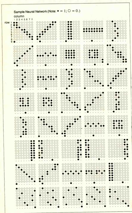
Figure 1: The original patterns for a sample neural network designed to illustrate the associative memory property. (Note:  $\bullet = 1$ ;  $\bigcirc = 0$ .)
