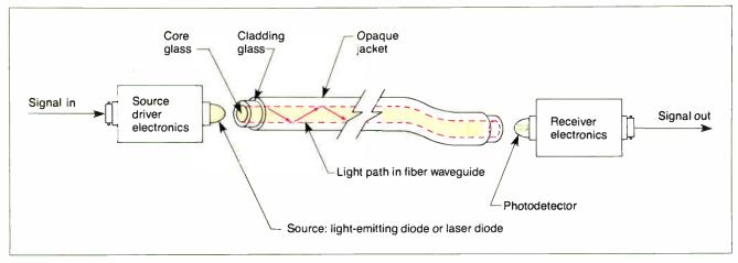
Figure 6: Basic optical-fiber communications link.
