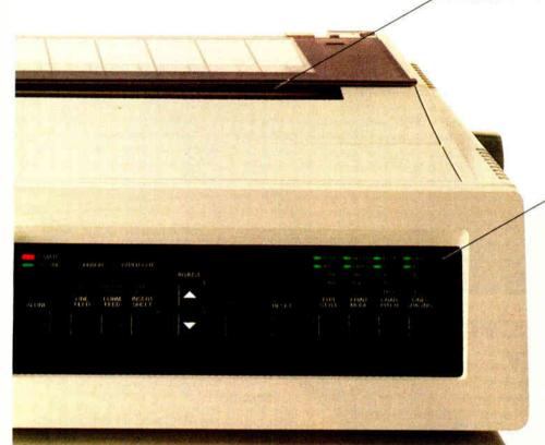
You also get conveniences that many other printers are lacking. Like control of everything from the front panel, the feature menu, or from software — without using DIP switches.
