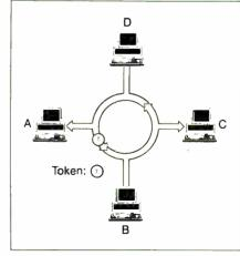
Figure 5: On a token-ring network, the "token" packet controls network access.
