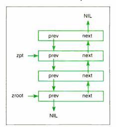
Figure 1: Typical stack structure.
