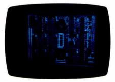
Photo 5c: The missing IC stands out.
