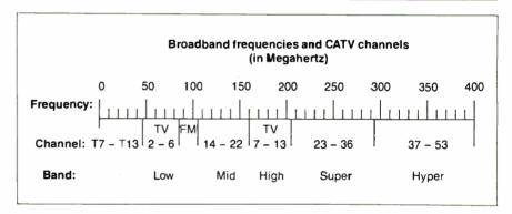
Figure 4: Spectrum of frequencies allocated for broadband transmission.
