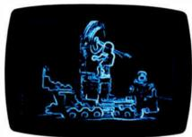
**Photo 8:** Edge detection with ImageWise. The image in (a) is processed through Edge, Multiply, and Thresh to produce (b).
