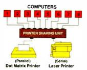
Our 4 or 8 port Printer Sharing Units work automatically with up to 256K buffering. No cable switching or knobs to turn. Software changes are usually unnecessary since they use standard Ready/Busy or XON/XOFF handshaking.
