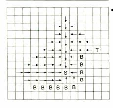
◆ Figure 3i: The flag array after the completion of the search phase. The home cell for step 11 is just to the left of the target (T) cell.
