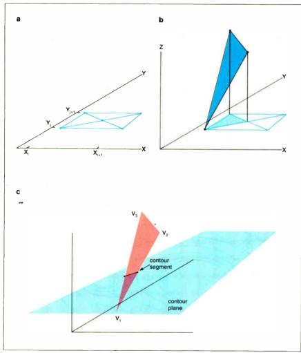
Figure 2: The data points are analyzed in groups of four contiguous points. These rectangles are divided into triangles (a). The centerpoint C's coordinates are interpolated, giving three triangles in three-dimensional space (b shows one of them). The intersection of these triangles with the contour plane determines the location of the contour segments (c).
