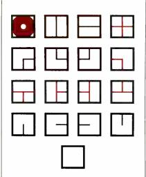
Figure 2: All of the possible cell contents for the basic Lee's Algorithm. Component leads are normally soldered to pads (the circular conductor, also called vias); most traces will start and end at a pad. Pads may be used to connect traces on two different layers.
