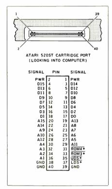
Figure 1: The Atari cartridge port and signals.
