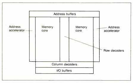
Figure 1: A floorplan for a RAM chip.
