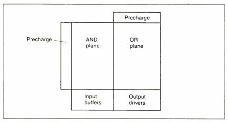
Figure 2: The organization of a programmable logic array chip.
