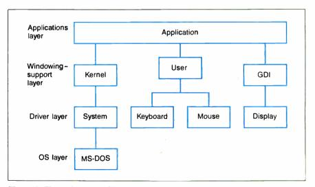
Figure 1: The architecture of Windows as seen from an application.
