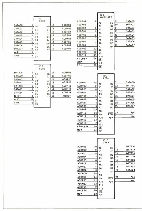
Figure 5: A CADcompiler schematic with each device shown separately, along with the signal names listed next to their corresponding pins.
