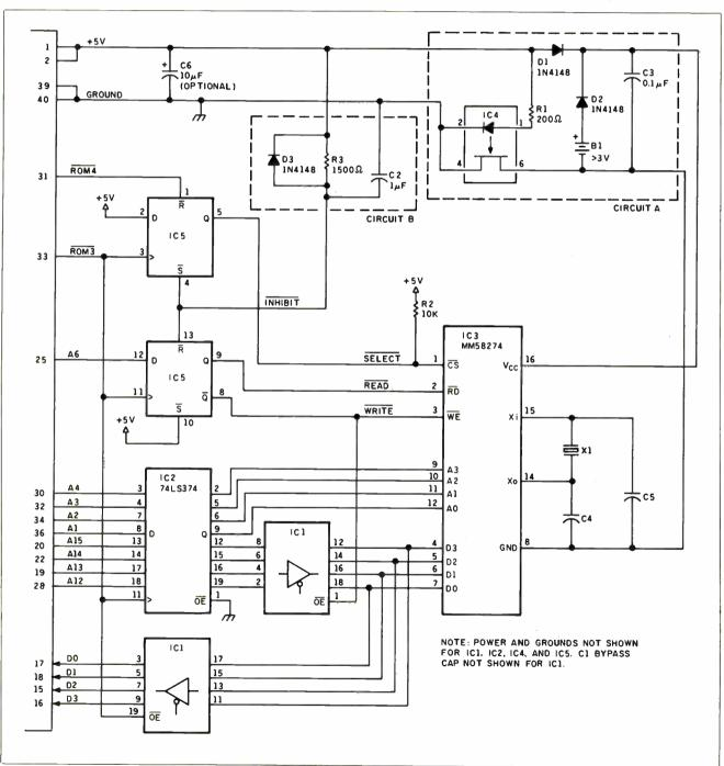
Figure 4: The clock/calendar circuit.
