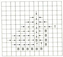
Figure 3h: The search wavefront continues to expand and is now within one cell of finding the target.
