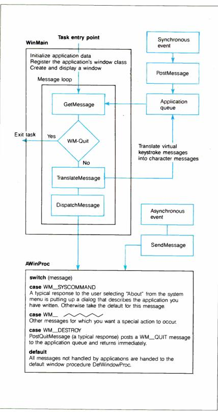
Figure 2: Every Windows application must have a WinMain procedure which serves as the entry point to the task. WinMain sets the stage for the application and then supervises the removal of messages from the application queue and the distribution of messages among the application's windows. PostMessage returns without waiting for the corresponding window to process the message; SendMessage doesn't return until the message has been processed.
