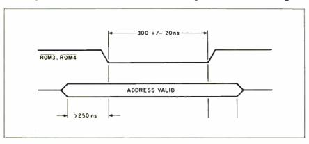
Figure 2: Cartridge-port address timing.
