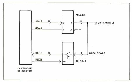
Figure 3: A simple circuit for data separation on the cartridge port.
