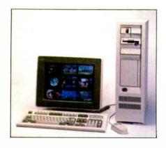
The PS/2 Model 80: IBM's first 80386-based computer.
