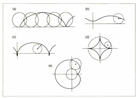
Figure 1: A variety of curves produced by rolling a circle along another curve: (a) simple cycloid; (b) curtate cycloid; (c) prolute cycloid; (d) hypocycloid of four cusps, or astroid; (e) epicycloid of one cusp, or cardioid.
