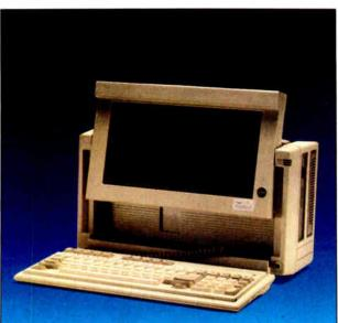
The Portable III's 80286 microprocessor is user-switchable between 12 and 8 MHz. The computer can also use an optional 8-MHz 80287 math coprocessor. It has 640K bytes of RAM on its main board and comes in three configurations: the Model 1 (\$3999), which includes a 1.2-megabyte floppy
