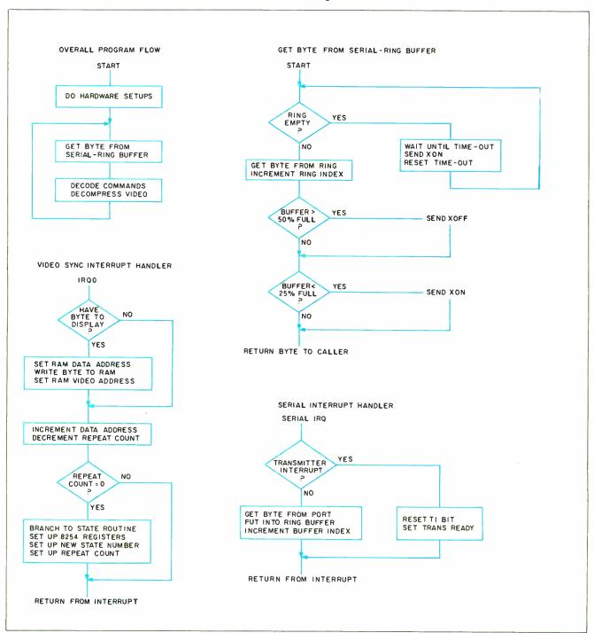
Figure 7: Flowchart for the ImageWise display/receiver system's software.
