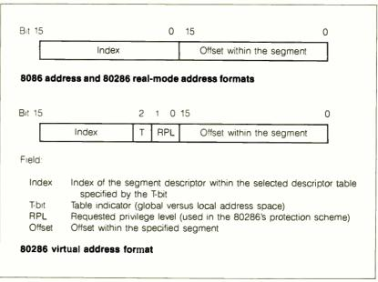
Figure A: The placement of the T-bit and the permission bits within the address/segment word on the Intel 80286.
