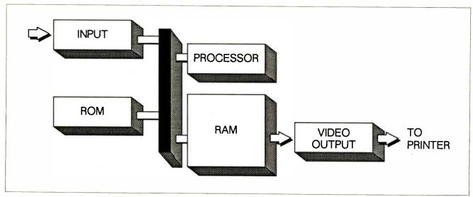
Figure 4: A simple raster-image processor.
