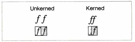
Figure 2: Unkerned italicized f's, shown on the left, each occupy an inviolate rectangle. Kerned letters, on the right, overhang each other, complicating the bitmapping algorithms.
