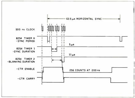
Figure 6: Timing pulses generated by the display/receiver's 8254 PIT.
