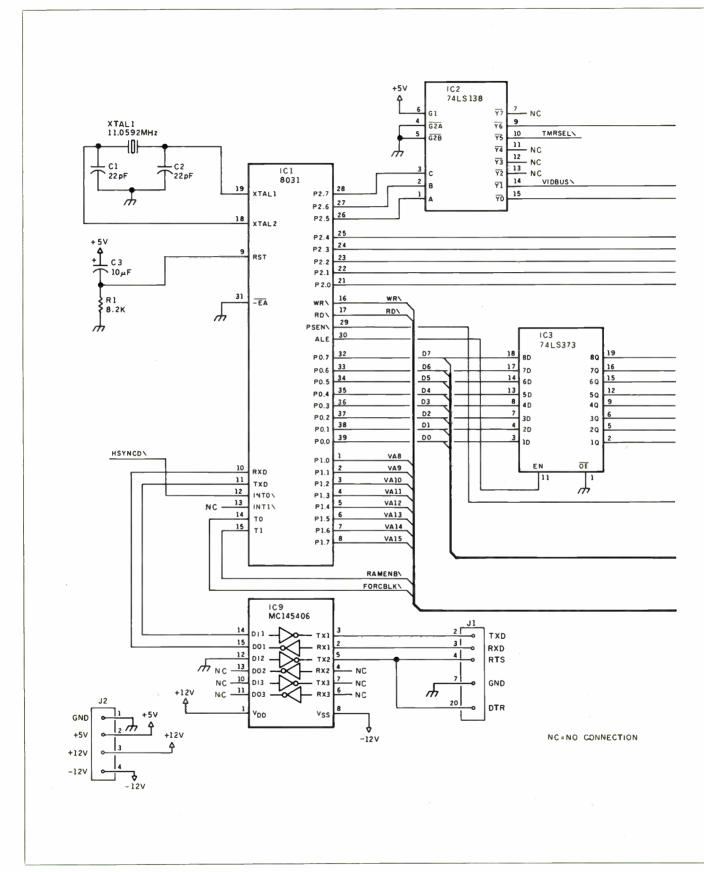
Figure 5: Schematic diagram of the ImageWise display/receiver hardware.
