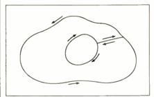
Of course, this is just a computerized mechanization of the old surveyor's areafinding tool, the planimeter. The technique is a limiting case of the method for finding the area of a triangle, which appears in many analytic geometry texts.
