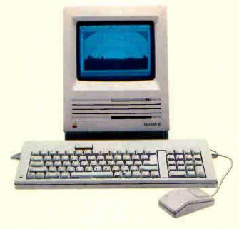
an extra 3½-inch floppy disk drive. Both hardware options are available from Apple for the Mac SE. Last but not least, a single 96-pin slot using a Eurocard type C connector is mounted on the side of the Mac SE's motherboard (see photo A). This connector makes unbuffered processor signals and power available to vendor cards that can be plugged into the slot. The card must lie parallel to the motherboard in the cramped space at the bottom of the Mac SE.
