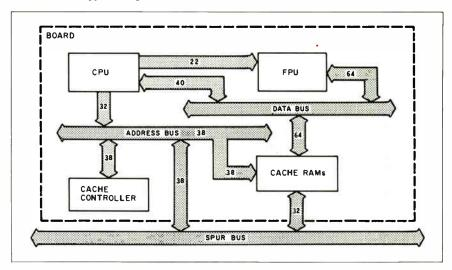
Figure 2: The SPUR processor-board block diagram.
