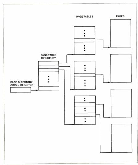
Figure 10: Virtual-to-real address translation proceeds quickly under the twolevel system that moves from a 1024-entry page-table directory to one-page tables to the pages themselves.
