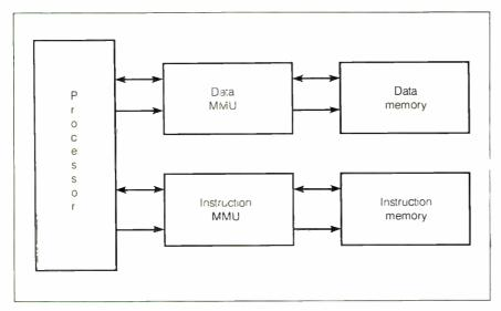
Figure 2: The Harvard-architecture method of linking a processor to memory.
