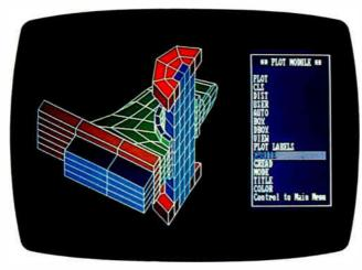
PCTRAN Plus helps create finite-element models.
