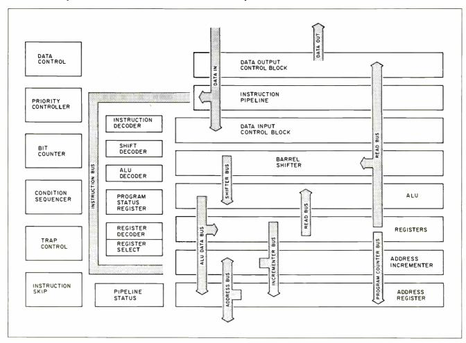
Figure 4: The ARM block-and-position diagram.
