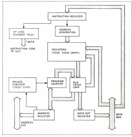
Figure 3: The AMD RISC-system block diagram.
