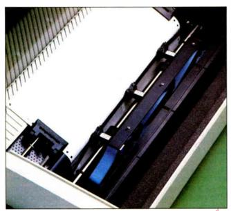
Photo 1: Output Technology's OT-700e uses a three-head design to achieve a maximum speed of 700 cps. The three heads give the greatest advantage for printing on wide forms because all three heads are used. On 8-inch forms, only two of the print heads are used.
