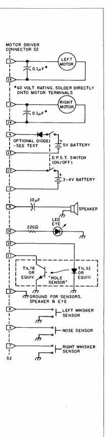
Figure 2: Schematic diagram of the robot base.
