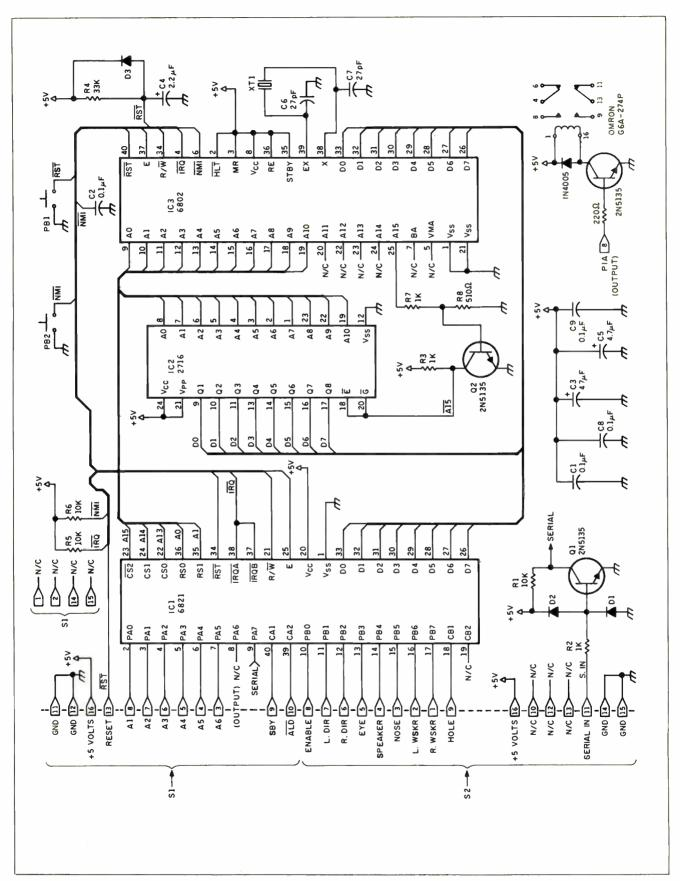
Figure 1: Schematic diagram of BERT's on-board computer.
