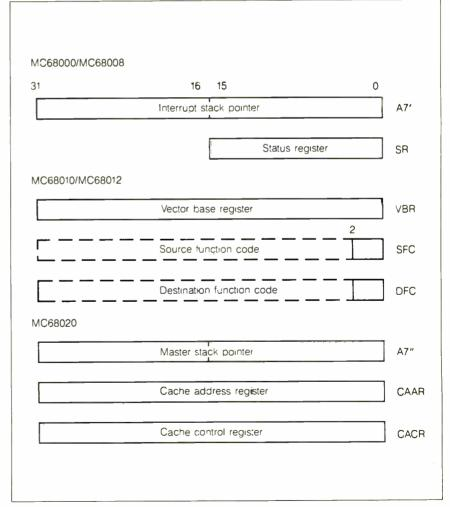
Figure 4: The additional registers in the supervisory programming model.
