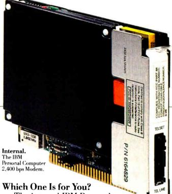
The internal IBM Personal Computer 2.400 bps Modem is designed to occupy a half slot in the IBM PC, XT, AT and 3270 PC.
