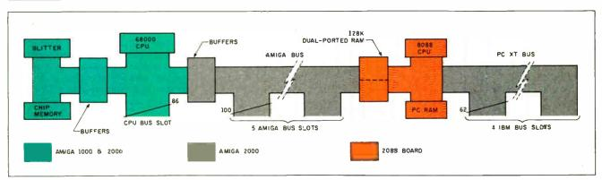
Figure 2: A simplified block diagram of the Amiga 2000 with the Amiga 2088 board installed. The CPU bus slot, Amiga bus slots, and PC bus slots can operate without interfering with the blitter chip.
