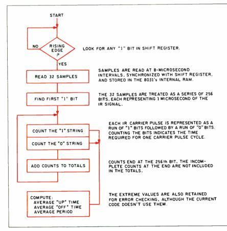
Figure 2: Carrier-frequency measurement flowchart.
