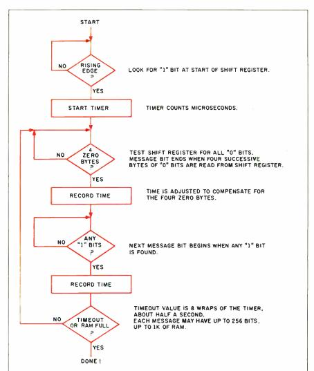
Figure 3: Signal-capture flowchart.
