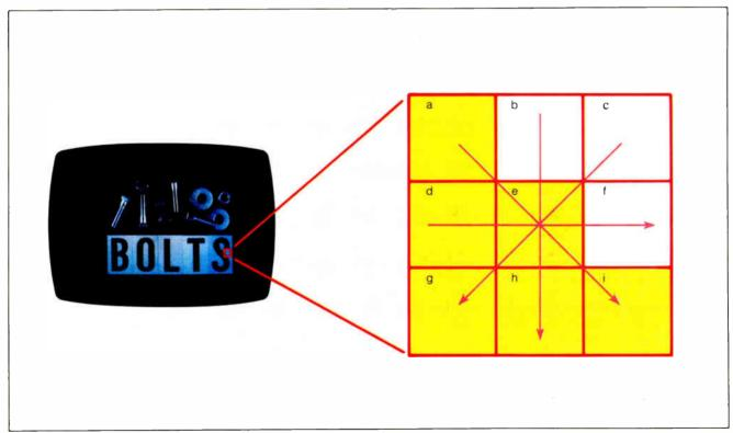
Figure 1: The Sobel algorithm for image processing breaks arrays of pixels into 3 by 3 subarrays.
