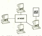
The PC Station is the only terminal of its kind with dual-host capability, which allows it to be connected to a mainframe host and an AT host simultaneously.
