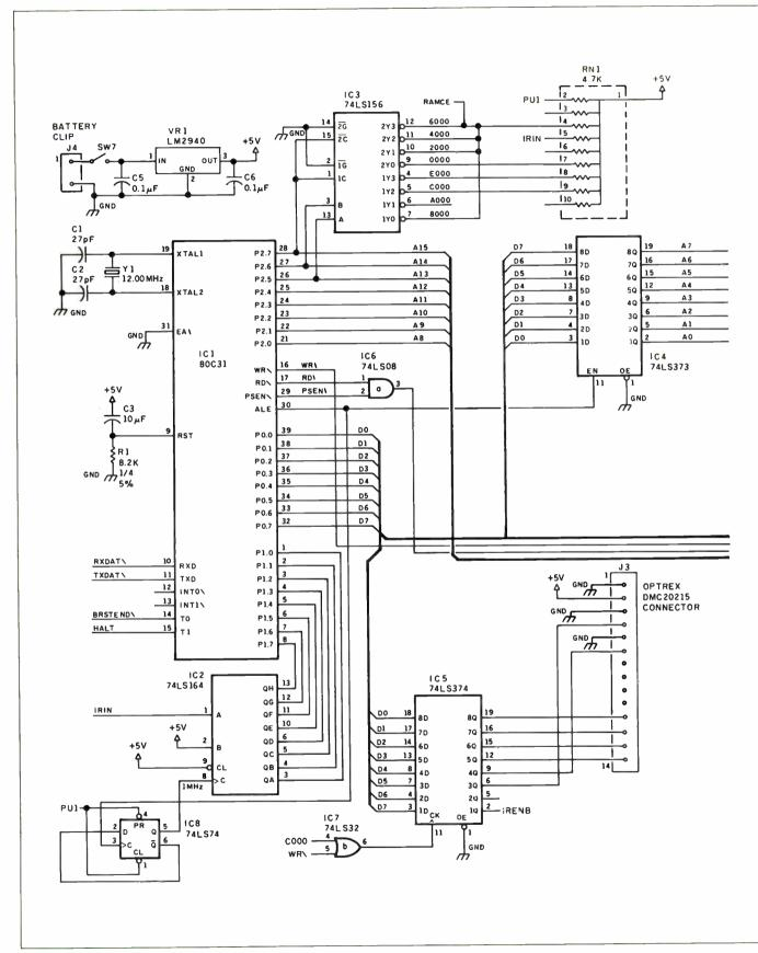
Figure 1: Master Controller schematic diagram.
