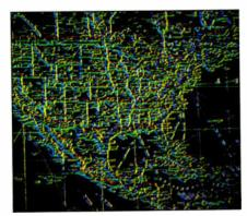
Photo 13: The result of a Sobel operation on a map of the United States. Edge orientation is represented by color, and edge strength by color intensity. (Photo courtesy of Imaging Technology Inc.)
