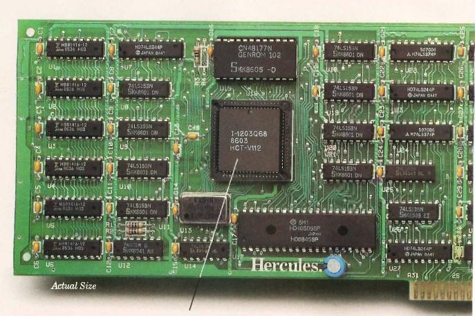
The heart of the Graphics Card Plus: the V112 microchip, Hercules' next generation video processor that makes the RamFont mode possible.
