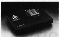
For economy. The single-socket SAILOR-1 EPROM programmer is small, portable, and fast. Dual sockets on the SAILOR-2 allow mini-gang and mini-set programming. Macros for totally automated operation!
