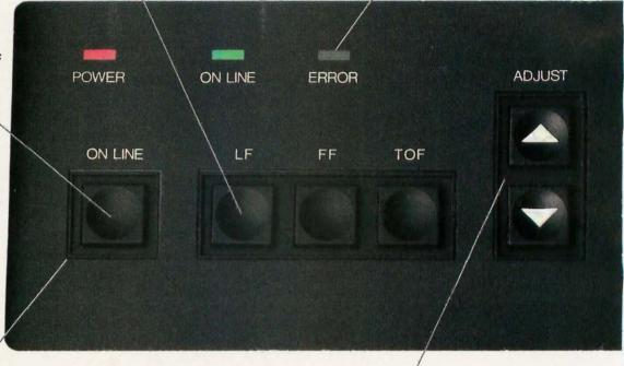
12 pushbuttons to control printing functions.
