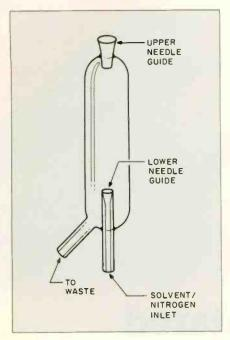
Figure 2: Self-cleaning syringe washer.
