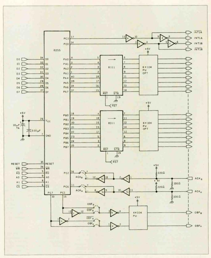
Figure 11: 16-bit buffered parallel output circuit.
