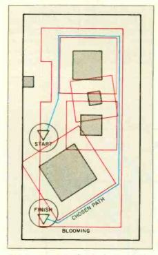
Figure 4: A Magellan-level navigation by HERMIES, showing the original spatial map, the blooming of obstacle diameters by HERMIES (red), and the selected path (blue).
