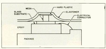
Figure 4: The major components of a single-element tactile sensor that measures force normal to its surface. By permission of Transensory Devices Inc., Fremont, California.
