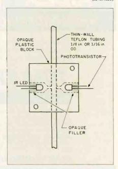
Figure 8: Liquid-presence detector.
