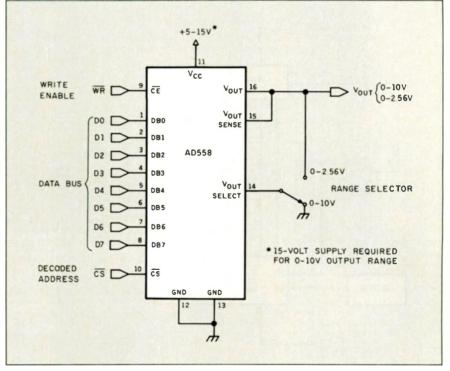
Figure 3: A block diagram outlining a typical connection of the AD558 8-bit multipluina D/A converter.
