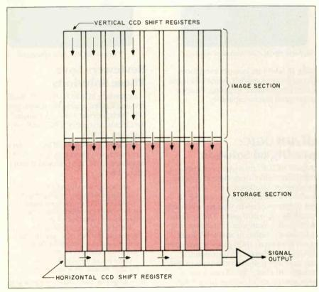
Figure 6: A diagram of a frame transfer CCD.
