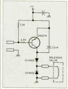
Figure 10: Valve-driver power booster circuit.
