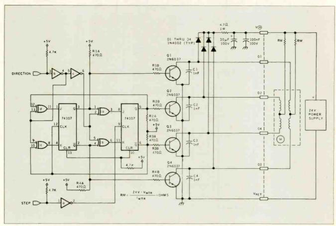
Figure 4: Stepper-motor drive circuit.
