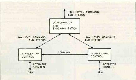
Figure 3: Simplified dual-arm control hierarchy showing low-level and high-level functions.
