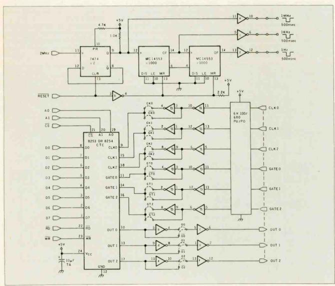
Figure 5: Real-time clock (CTC) circuit
