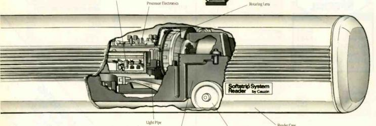
One Softstrip data strip, typically 5/8" x 91/2", can contain up to 5,500 bytes of information. (For example, you could fit this entire ad on two strips.)
