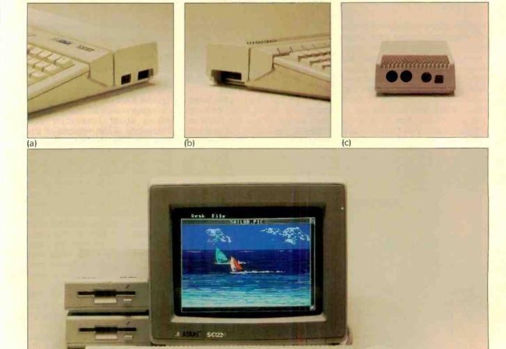
Photo 1: The Atari 520ST, shown here with the color monitor and two single-sided double-density disk drives. (a) On the right side of the keyboard unit are two joystick/mouse ports. (b) On the left is the 128K-byte ROM cartridge port. (c) The rear of the disk drives has specific ports for 1/0 in and 1/0 out.
