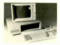
Limited time special offer: 640KB CPU. Floppy Controller, Keyboard, Parallel Port, Serial Port, Game Port, Clock, two 360 KB Disk Drives ..... all for \$799
