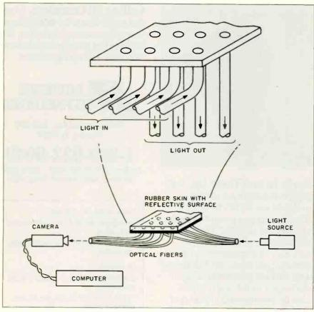
Figure 2: A tactile sensor based on the use of fiber optics, designed by John L. Schneiter and Thomas B. Sheridan. Reprinted from Robotics and Computer-Integrated Manufacturing. Courtesy of Pergamon Press.
