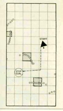
Figure 5: A Columbus-level navigation by HERMIES. Obstacles are drawn into the figure but were not available to the robot. The small circles represent the obstacle locations as they appeared on sonar
