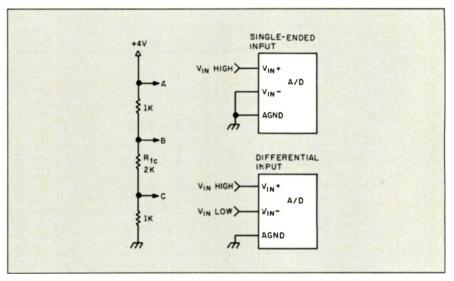
Figure 7: Comparison of single-ended versus differential input connections.
