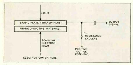
Figure 3: A diagram of a vidicon tube sensor.
