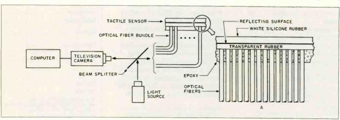
Figure 3: A fiber-optic-based tactile sensor that uses each fiber as both emitter and receiver. Reprinted from Robotics and Computer-Integrated Manufacturing. Courtesy of Pergamon Press.
