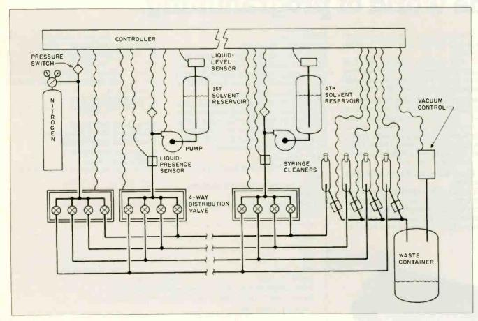
Figure 3: Syringe-cleaner subsystem.
