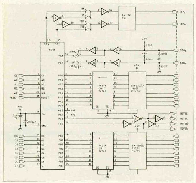
Figure 9: 16-bit buffered parallel input circuit.
