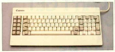
Photo 1: Keyboard of the Canon A-200 computer. It is identical to the IBM PC keyboard.
