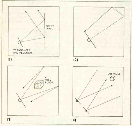
Figure A: Sonar problems. (1) Specular reflection, (2) false distance readings caused by reflection. (3) absorbancy, and (4) beam focusing.
