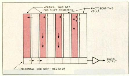
Figure 5: A diagram of an interline transfer CCD.
