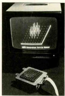
Photo 1: LTS-100 sensor with display of tactile impression. Used with permission of Lord Corporation, Erie, Pennsylvania.
