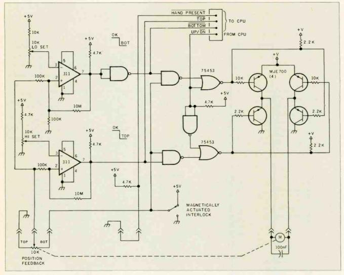
Figure 12: Parked syringe hand drive circuit.
