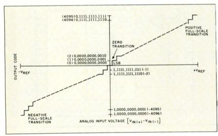
Figure 6: ADC1205 output characteristics.
