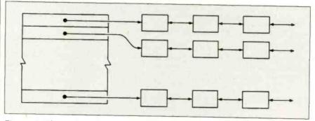
Figure 5: The structure of the symbol table: an array of pointers to doubly linked lists of symbol-table entries.
