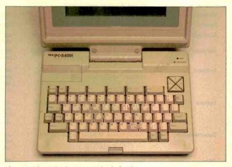
Photo 6: The NEC PC-8401A 68-key keyboard.
