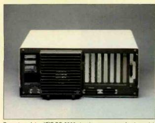
Rear view of the AT&T PC 6300 showing connectors for the serial port, parallel port, keyboard, and monitor. Note the oversize cooling fan, protective shroud, and connector access slots for the seven expansion boards.
