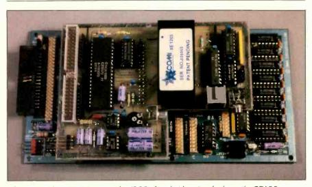
Photo 3: The COMMI80 modem/SCSI board rides piggyback on the SB180 single-board computer. connecting via the SB180's expansion 1/O connector.
