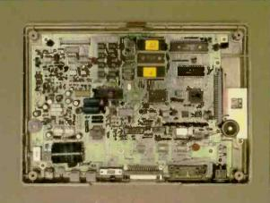
The NEC PC-8401A's internal circuitry.
