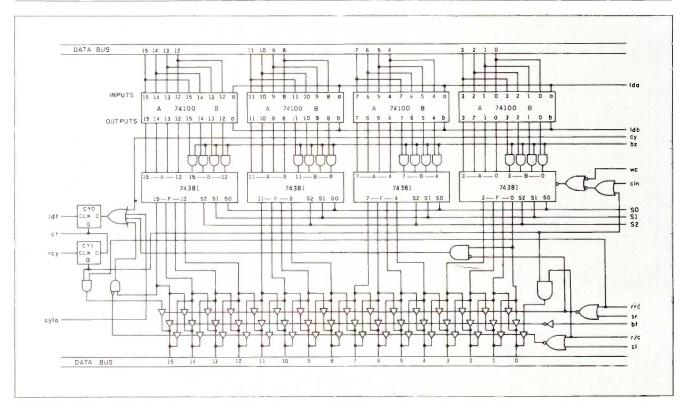
Figure 7: EGO's ALU. Note the bank of tristate drivers near the bottom used to perform shift and rotate instructions.
