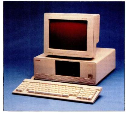
Photo I: Overall view of the Ericsson PC showing the system unit, the keyboard, and the monitor.
