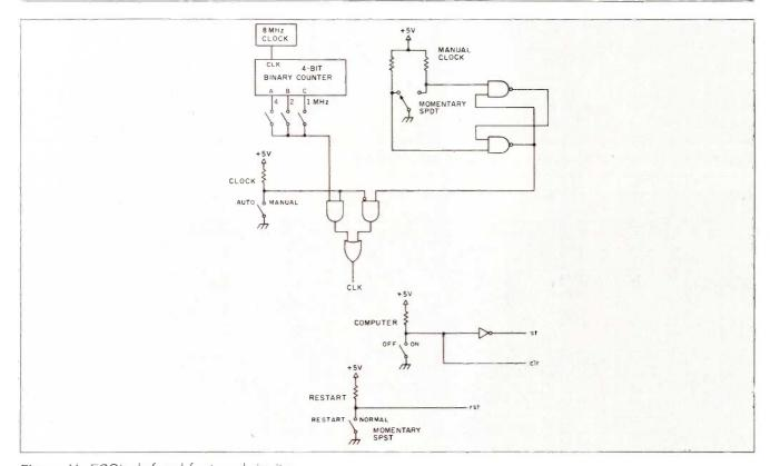
Figure 11: EGO's clock and front-panel circuitry.
