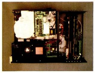
Inside the Stearns. The slots, fan, floppy-disk drive, and hard-disk drive are evident.
