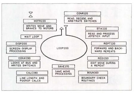
Figure 2: A software flow-of-control diagram for Skycam's main software loop. The text above the double line in each box is a FORTH word whose function appears below the line.
