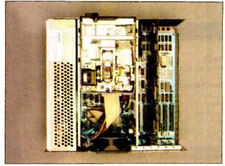
Top view of the main unit with the cover removed to show expansion slots and internal hardware.
