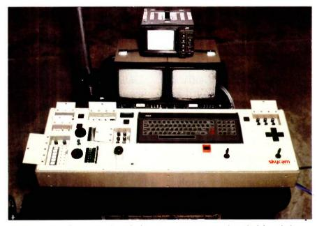
Photo 2: The Skycam console with the camera operator's panel at the left and the pilot's jousticks on the right.
