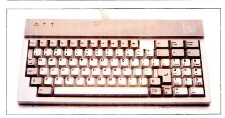
Photo 3: Keyboard for the STM Personal Computer. Note the enlarged return key and the special function keys on top of the alphanumeric keys.
