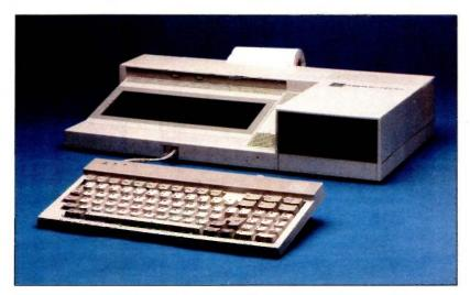
Photo 1: The STM Personal Computer with two 5¼-inch floppy-disk drives and an 80-character by 25-line LCD with electroluminescent backlighting.
