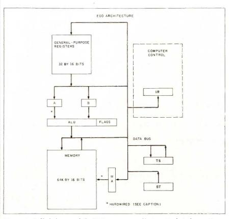
Figure 1: A block diagram of the EGO processor's architecture. Hard-wired connections indicate signals that are never "turned off." For example, the output of the A register is always sent to the ALU, but the output of the B register can be disconnected from the input of the ALU for those instructions requiring only one operand (shifts and rotates).
