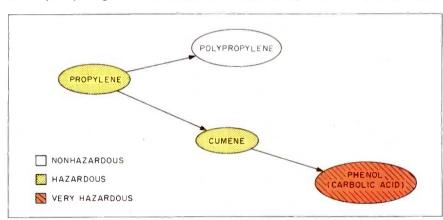
Figure 1: The propylene-phenol production chain.
