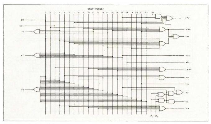
Figure 4: Another portion of the EGO sequencer circuit.
