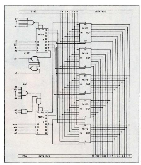
Figure 12: EGO's I/O interface circuitry.
