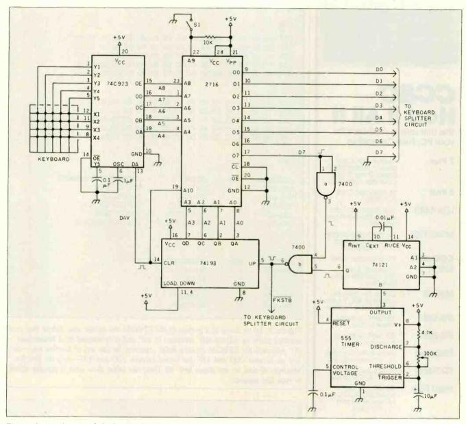
Figure 2: A schematic of the function-key-generator circuit.
