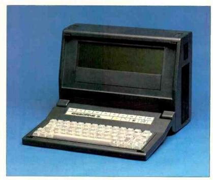
Photo 1: The Osborne 3 with an 80-character by 16-line liquid-crystal display and two 51/4-inch floppy-disk drives.
