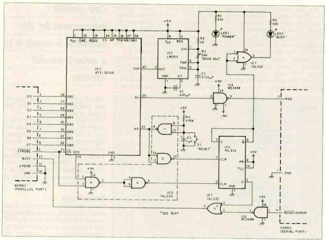
Figure 1: A schematic for the parallel-to-serial adapter. The UART (ICI) converts the 8 bits coming in at the parallel port
