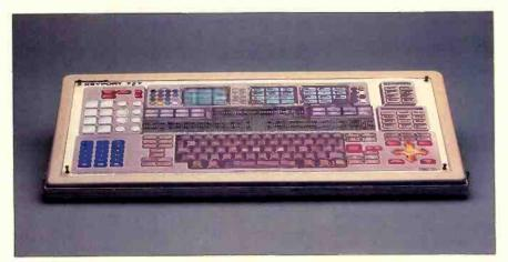
Photo 1: The Keyport 717 with the BASIC programmer's overlay.
