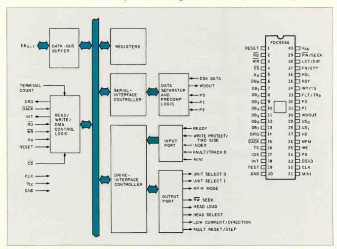
Figure 3: Block diagram and pin-out of SMC's 9266.
