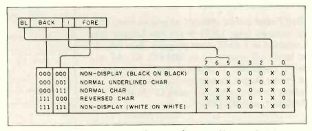
Figure 6: The translation of the monochrome attributes. In addition to the IBM PC attributes, the APC III supports additional features like overlining and vertical bars.
