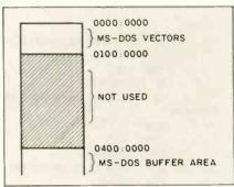
Figure 1: The patch program makes use of undefined interrupt locations and stores an attribute-translation subroutine at address 0010:0000 (all addresses in the figures are in hexadecimal notation).
