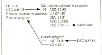
counter with the value 8, which is actually an unconditional jump to memory location 9 (since the program counter is automatically incremented at the end of every instruction). I can use any register as an index register. The simplicity gained by my instruction set resulted in a few strange-looking instructions. I have not yet found a use for some of the data instructions.
