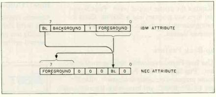
Figure 5: The translation of the color attributes. Note that the APC III cannot make use of the background color or the intensity flag.
