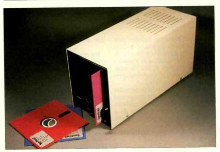
Photo 4: The enclosure from photo 3 is shown with the cover on. The only additional hardware necessary to use the system is a serial terminal.
