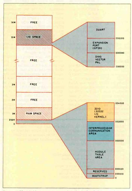
Figure 1: The DSI-32's memory map. 3210 is the 1/0 kernel that resides between locations 3000 and 4000. All addresses are in hexadecimal.
