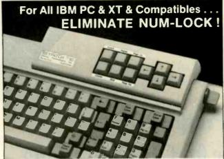
KEYPATCHT -10 - A full travel mini-keyboard. Plugs between keyboard connector and CPU. Automatically activates NUM-LOCK placing your IBM™ keyboard into the number pad mode while KEYPATCH™ -10 provides separate cursor and screen control functions without the use of the NUM-LOCK key. Saves time — eliminates errors. KEYPATCH™ -10 requires no software. A must for spread sheets; word processing; graphics; etc.
