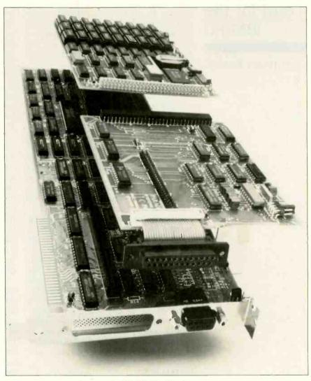
Photo 1: Modular Graphics Card from Paradise Sustems fits into any full-size slot in an IBM PC or compatible. The connector at the bottom right of the photo mates with a cable from a monochrome TTL monitor. Also shown are two of Paradise's optional addon modules; at the top is a combination RAM/clock card, and below that, a serial adapter card.
