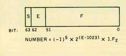
Figure A: IEEE standard for 64-bit floating-point number. The S bit indicates the number's sign—0 is positive and 1 is negative. The E or exponent field is in excess-1023 form (subtract 1023 from the value in the E field to get the actual exponent). The F field holds the fractional portion of the number.
