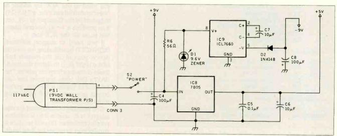
Figure 2: The power-supply adapter for the parallel-to-serial converter of figure 1.
