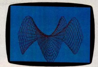
**Photo 3:** The plot of z = x \* y \* (x \* x - y \* y) / (x \* x + y \* y). The border has been eliminated and cross-hatching added in this plot. Using red on blue instead of the default colors requires only the use of the estimate-scales selection instead of the auto-graph routine.
