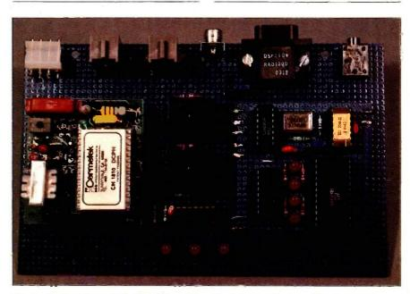
**Photo 3:** Prototype of the Touch-Tone Interactive Message System. The connectors from left to right are the power supply, answering-machine connector, telephone-line input. Microvox speech-synthesizer output, parallel 1/O interface to computer, and the answering-machine earphone output.
