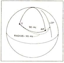
Figure C: In this case 90-H0 is greater than 90-Hc. Your actual position lies on an arc (LOP) of a circle of center 0 and radius 90-H0.
