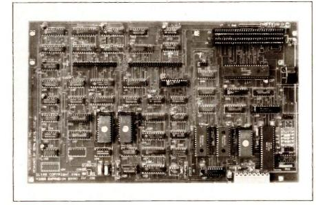
Photo 3: The video expansion board supports an IBM-compatible 80 by 24 monochrome display, 640 by 200 bit-mapped graphics, and has two IBM PC slots and a connector for an IBM replacement keyboard.
