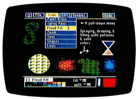
**Photo 2**: Dazzle Draw at work. Note the pull-down menu. Active selections are in blue, inactive ones in gray; a menu selection is yellow when it is about to be activated by the cursor; the Undo box is red when an action can be undone. The colored areas were made using both solid colors and patterns with the Paint Brush, Spray Paint, Flood Fill, and Shapes tools. The area at the bottom is the "control panel" for the current tool, Flood Fill.
