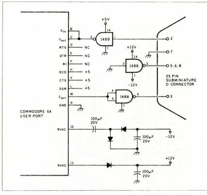
Figure 3: A schematic of the RS-232C interface.
