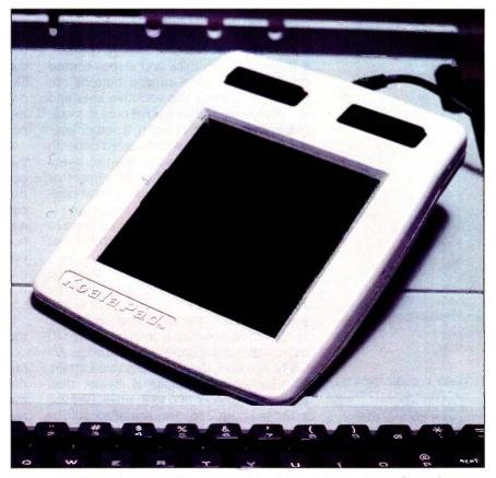
**Photo 1**: The KoalaPad provides a method for entry of data or for making selections from the screen using touch rather than the keyboard.
