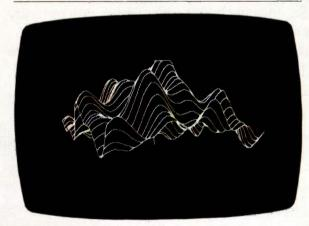
**Photo 7:**  $Z = \cos(x + y) * \cos(3 * x - y) + \cos(x - y)$ \*  $\sin(x + 3 * y) + 5 * \exp((-x * x - y * y) / 8)$ . The clipped peak in the back of the plot illustrates the kind of problem that can arise from auto-graphing complex functions. You can eliminate this by adjusting the scaling factors after viewing the plot.
