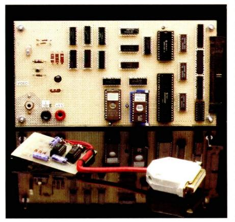
Photo I: The 80-column board and the RS-232C interface board.
