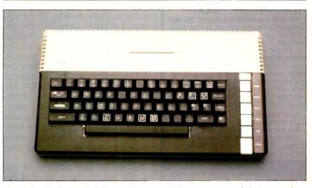
Photo 2: The keyboard of the 800XL. Note the better placement of the inverse-video key in the lower right corner.
