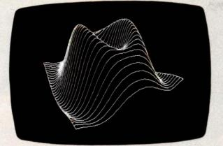
**Photo 2:** The plot generated by sin (x \* x + 2 \* y \* y) \* exp(-x \* x - y \* y)after rotating -5 degrees around the y-axis and changing the x and y scales. The colors are the default high-resolution colors.
