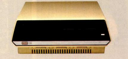
The Altos 586 system unit, showing a single floppy-disk drive.
