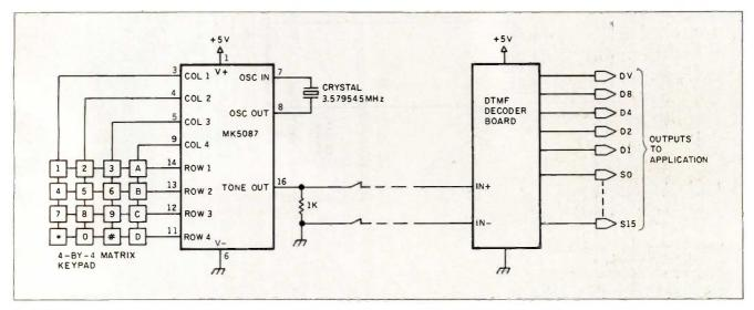
Figure 5: DTMF encoder/decoder remote-control circuit.
