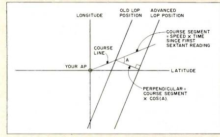
Figure E: Advancing or retiring the LOP is done by moving the line along a perpendicular to itself, a distance equal to the course segment  $X \cos(a)$ . The course segment equals your speed multiplied by the time elapsed since the last sextant reading.
