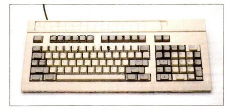
Photo 4: The APC III keyboard. Note the 12 unlabeled programmable function keys and the template for recording the functions.
