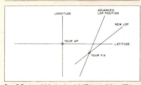
Figure F: The point at which the advanced, or retired, LOP intersects with the new LOP is your new fix. The point of intersection can be solved using analytic geometry and by solving a set of two simultaneous equations in two unknowns.
