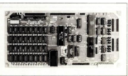
Photo 2: The Slicer expansion board has an additional 256K dynamic RAM, a realtime clock/calender with battery backup, a parallel port, and four serial ports.
