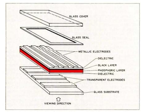
**Figure 3**: Cross-section of an ACTFEL display panel. The phosphoric layer glows in response to voltage applied through the matrix of electrodes. Substituting other materials for the manganese dopant changes the color of light given off.
