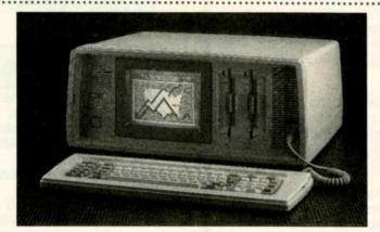
The Sanyo's screen accommodates 80 by 25 characters in regular mode and 40 by 25 characters in double-sized mode. The machine has 16-color graphics capabilities with 640- by 200-pixel resolution in color mode. In black-andwhite mode, resolution is 320 by 200 pixels. Bundled software for the MBC 775 includes EasyWriter 2. EasyMailer. EasyPlanner. and EasyFiler. Its operating system is MS-DOS 2.11, and it also features GW-BASIC.
