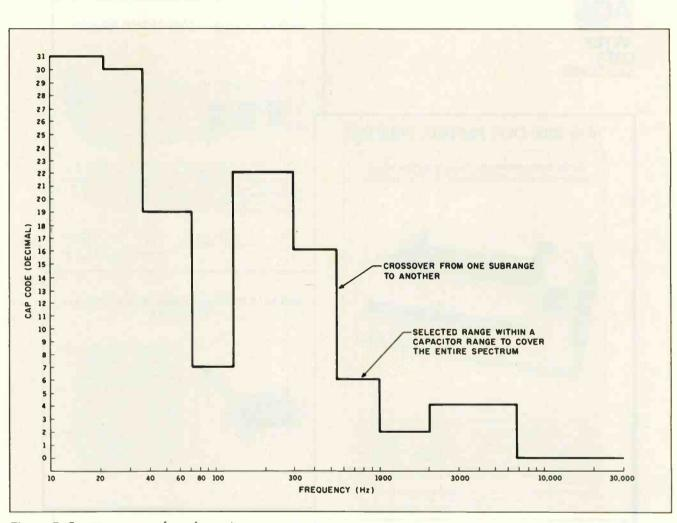
Figure 7: Spectrum coverage by each capacitor range.
