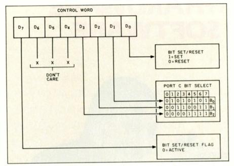
Figure 5: Setting the port C bits of the 8255A using the control word.
