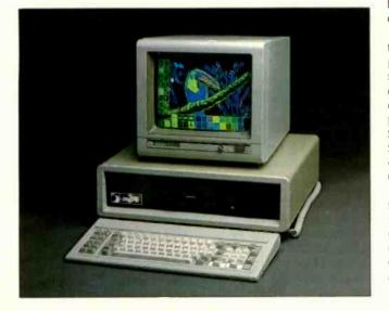
IBM PC rate of 4.77 MHz. Seequa says another function of the 16-bit hardware bus is to produce a flickerfree image for the Cobra's color-graphics display.
