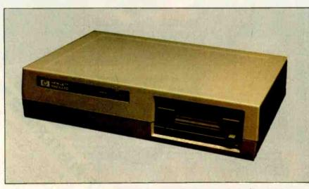
Photo 5: The HP 9114 portable disk drive contains a  $3\frac{1}{2}$ -inch, double-sided Sony disk drive capable of storing over 680K bytes of data. Also included is a lead-acid battery and interface electronics.
