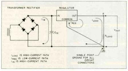
Figure 10: The proper power-supply layout
