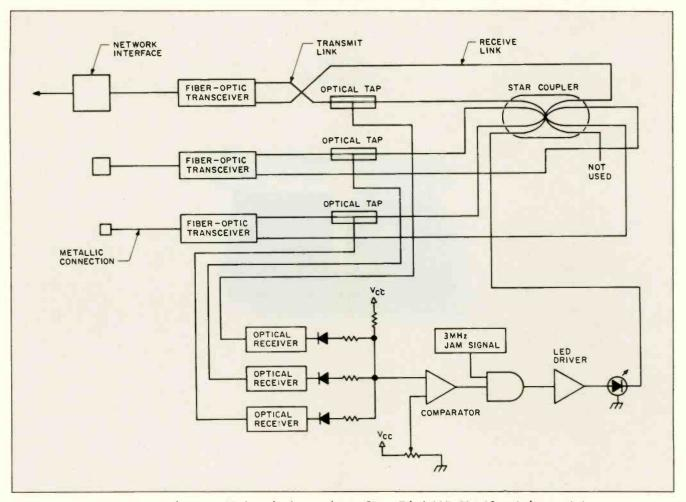
Figure 4: Ungermann-Bass's Fiber Optic Net/One local network uses Siecor FiberLAN's Net 10 optical transmission system, a cabling setup similar to IBM's in that a star-like formation of cables is used to connect devices on the network with centralized wiring locations. A passive star coupler lets data-bearing light propagate throughout the network for Ethernet compatibility.
