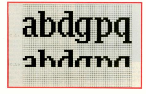
forms on most computer terminals usually provides a single size of a single style of coarse-resolution dotmatrix letters. Character-generator technology usually does not let the user modify the fonts because the character images are contained in hardware or firmware.
