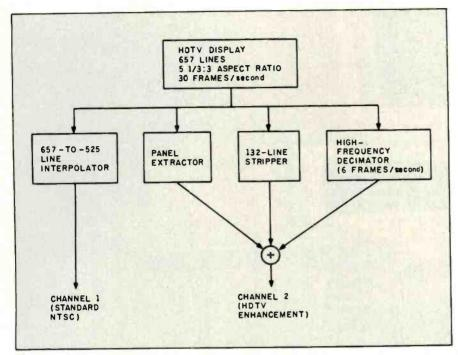
Figure 6: A block diagram of two-channel decomposition.
