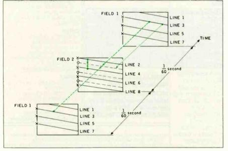
Figure 2: The sequential-scan conversion process. X indicates a transmitted line; O indicates a locally interpolated line. The solid green line indicates line average (motion), green dashes indicate picture average (still), green dots indicate field insertion (still).
