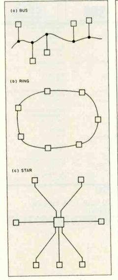
Figure 1: The bus, ring, and star topologies (or connection configurations) shown in their idealized forms.
