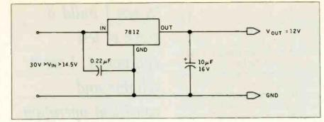
Figure 5: A typical +12-V fixed-voltage output regulator.
