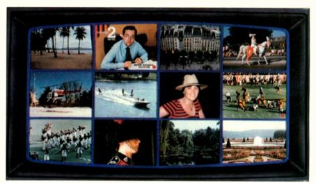
Photo 2: An example of multiple-picture-in-picture display using the  $5\frac{1}{3}$ :3 aspect ratio CRT The red dots in the two corners of the small windows indicate high-definition television display availability.
