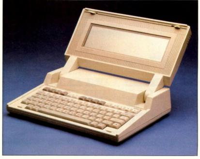
Photo 1: The HP 110 Portable Computer.
