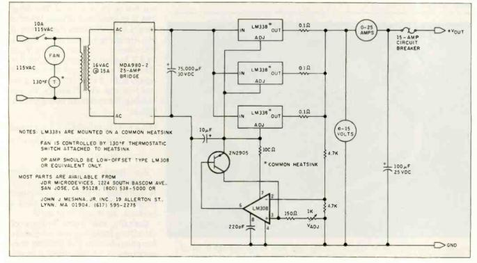
Figure 8: A 12- to 13.2-V 15-A power supply that uses readily available components.
