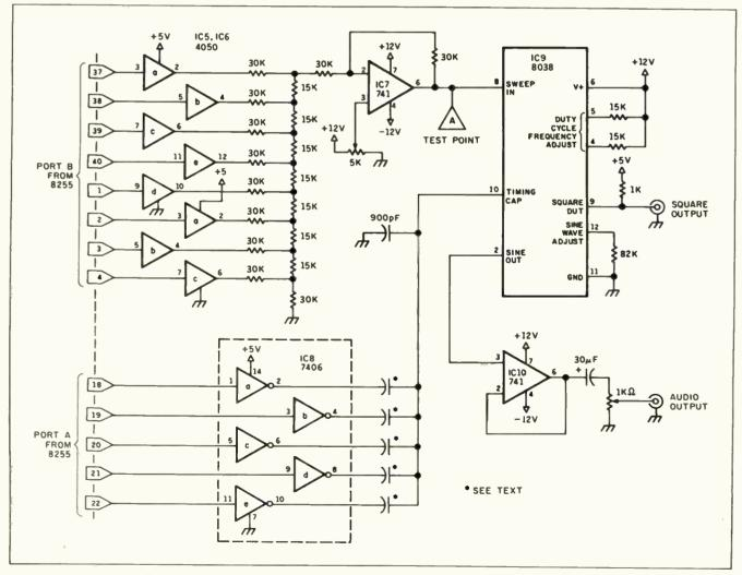
Figure 3: Voltage-controlled oscillator and driver circuitry.
