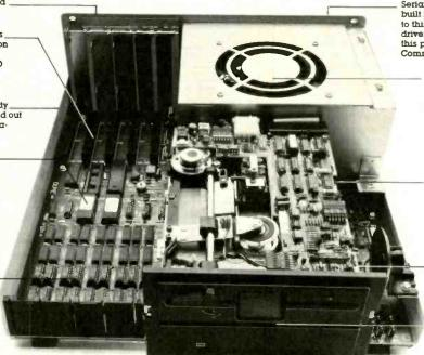
Serial (RS-232) communications port built in. Console I/O may be redirected to this port by switch setting. Menudriven DOS utility (set up) to configure this port or redirect printer I/O to it. Communications program included
