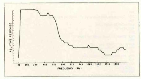
Figure 12: Frequency response with full bass on.
