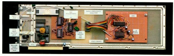
Photo 1: Audio-frequency analyzer board.
