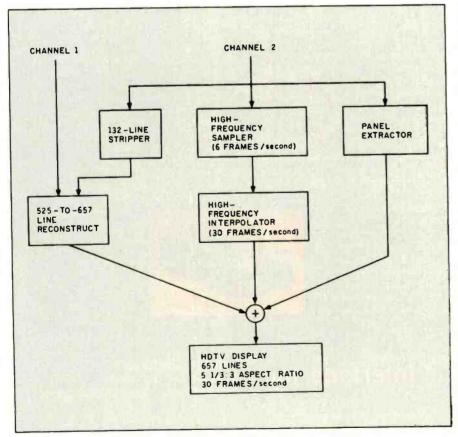
Figure 7: A block diagram of two-channel reconstruction.
