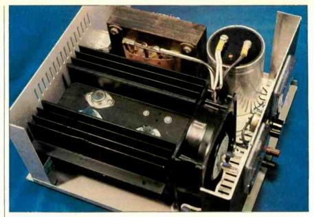
**Photo 3:** The completed power supply has little extra internal space. You'll notice that the filter capacitor has two sets of connecting wires to conform to the layout guidelines I've described. While the heatsink is sized properly for ambient air installations. I have added a fan to compensate for the insulating effect of the enclosure. To limit noise, the fan is controlled by a 130°F thermostat attached to the heatsink. The thermostat turns on the fan only when necessary.
