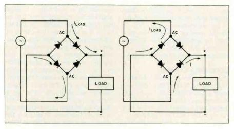
Figure 2: The current flow through a full-wave bridge. Two diodes are conducting current at any one time. They present a voltage drop of 1 V each.
