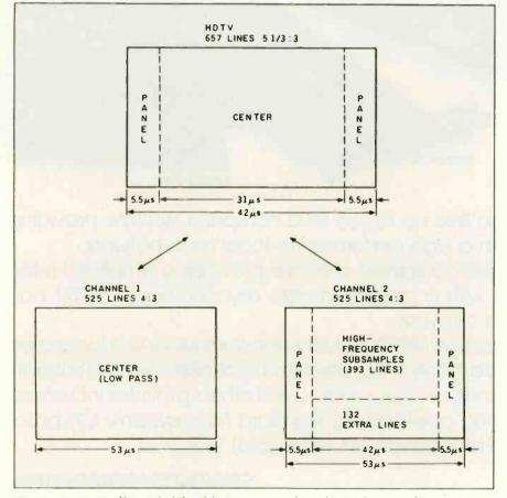
Figure 5: A possible method for delivering a two-channel NTSC-compatible high-definition television transmission.
