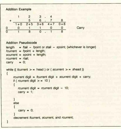
Figure 2: Addition algorithm example and pseudocode.
