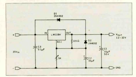
Figure 6: A typical variable-voltage three-terminal regulator.
