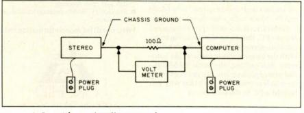
Figure 6: Potential ground problem test configuration.
