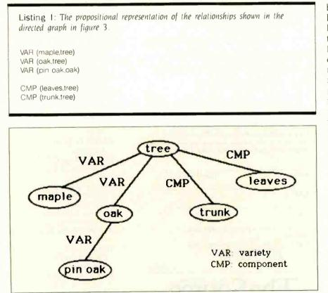
Figure 3: A notation used in knowledge representation known as the directed graph. The nodes (ellipses) stand for concepts while the arcs (the connections between the nodes) indicate the relationships between those concepts.
