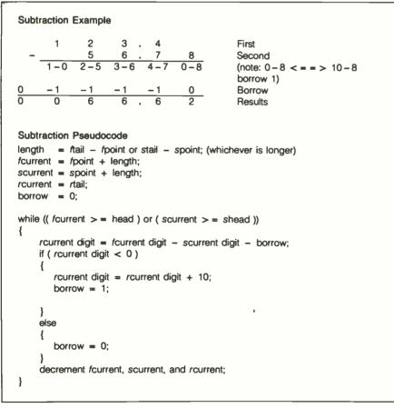
Figure 3: Subtraction algorithm example and pseudocode.
