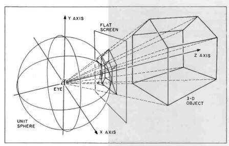
Figure 1: True perspective and drafting perspective both depend on the intersection of a vector by a surface at some distance from the eye. Because the sphere is curved it presents a more natural view.
