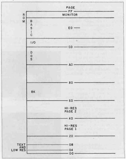
Figure 2: The y-axis paper scale used to label the Apple 11+ memory-location display.
