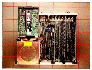
The inside of the Leading Edge. The disk drives are at the upper left (front) of the machine.
