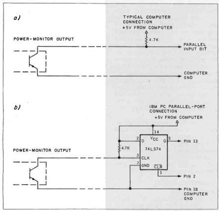
Figure 3: The connection between the computer and the power monitor: (a) shows the usual connecting circuit; (b) shows the circuit needed to connect the monitor to an IBM PC.
