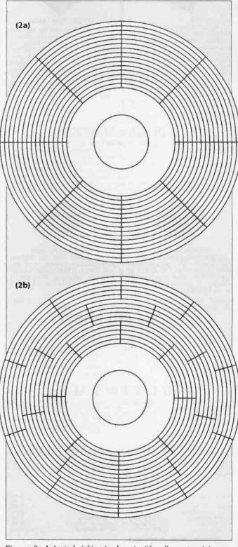
Figure 2: A typical eight-sector layout with radius sectors (a). Sector layout traditionally focused on the pie cut. Newer methods involving fixed-bit-cell sectors (b) enable a disk to hold up to 40 percent more data.
