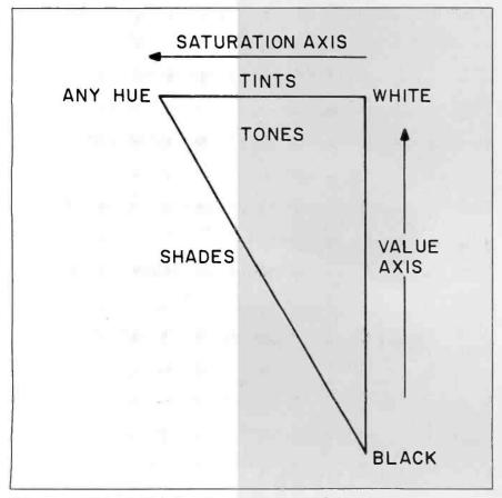
Figure 5: Cross section of the HSV hexcone showing tint, shade, and tone.
