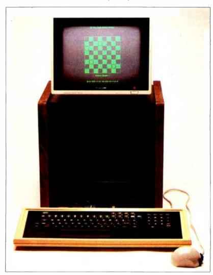
Photo 1: The Lilith Personal Computer. The four components of a Lilith are the system unit. the video display, the keyboard, and the mouse.
