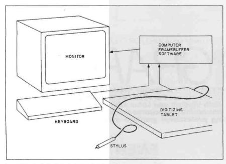
Figure 6: Tools for the selection and mixing of color, as in a paint system.
