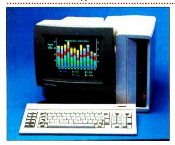
TeleVideo's color version of its IBM PC-compatible computer. the TeleColor PC. Model TS 1605C. comes with word-processing. spreadsheet. and database-management applications software and Microsoft's GW-BASIC. It's built around Intel's 5-MHz 8088 microprocessor and runs under TeleVideo's TeleDOS operating system. which is compatible with MS-DOS 2.11.
