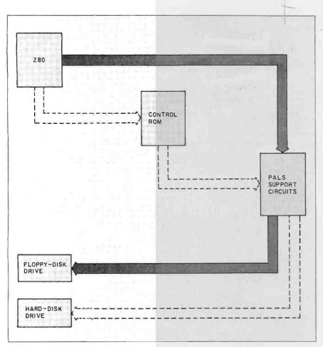
Figure 2: Central to its bid for higher speeds is the MD-11's controller, which, among other things, reduces the number of memory transfers required to deliver the data to its destination.
