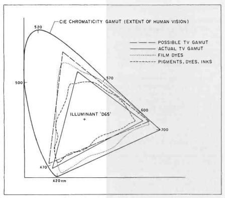
Figure 1: A diagram indicating the color spaces, or "ranges," of human vision. television. photographic film. and print media.
