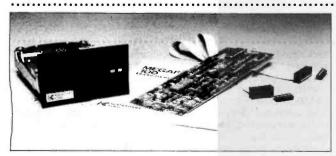
The Megaflight 100 is a 10-megabyte IBM PC and PC-compatible hard-disk drive that sells for \$895. It uses PC-DOS 2.0 or 2.1 software drivers, which gives it full compatibility with most IBM PC and PC XT software, Including Lotus 1-2-3 and MicroPro WordStar.
