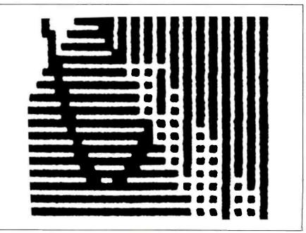
Figure 3: The film positive used to create the silk screen retains the irregularities of the dot-matrix printout from which it was enlarged.
