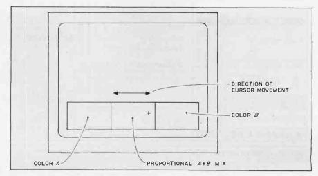
Figure 8: Using the system's Mix option to mix two colors on the monitor.
