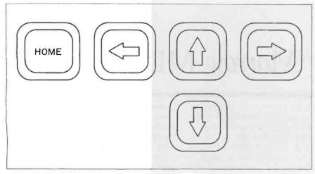
Figure 1: Morrow arranged the cursor-control keys in what might be termed an inverted-modified diamond and placed them at the upper right of the keyboard with Help to the left of Home and Erase to the right of Right cursor.
