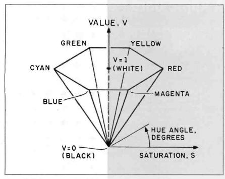
Figure 4: A hexcone representing the hue. saturation, and value (HSV) color model.
