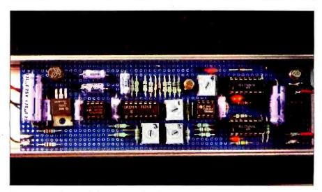
Photo 6: A close-up of the power-monitor electronics.
