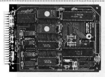
connector brings out the four parallel ports. TTL and RS-232C serial data, and a +5-V ground.
