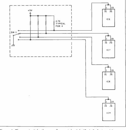
Figure 1: The new circuit for the manually operated switch. ICs 1, 2, 3, 4, and 5 are replaced by the circuit in the dashed box.
