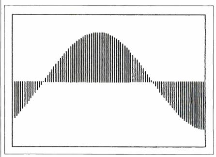
Figure Ic: A sense of solidity is added to the sine wave by plotting lines from the x-axis to the curve.
