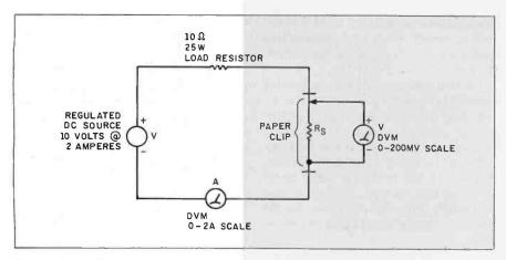
Figure 2: Calibrating the paper clip.
