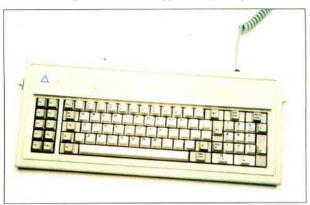
Photo 2: The keyboard of the Leading Edge. Note that the key layout is identical to that of the IBM PC's keyboard.
