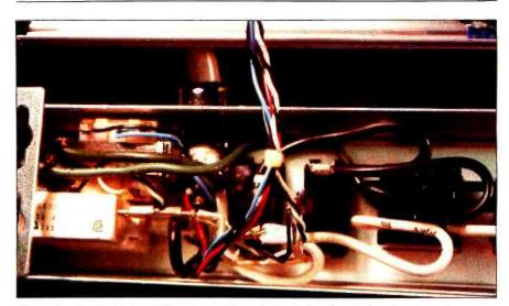
Photo 5: A 12.6-V AC. 300-mA transformer is inserted and secured within the case next to the circuit breaker. Its output is also connected to the power-monitor electronics.
