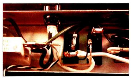
Photo 4: The wire from the hot side of the breaker (black wire) to the switch is replaced with the paper clip sensing resistor. Notice how it is bent to fit the enclosure. It is insulated with heat-shrink tubing. The sensing wires (#22 black-and-white) are connected to the power-monitor electronics.
