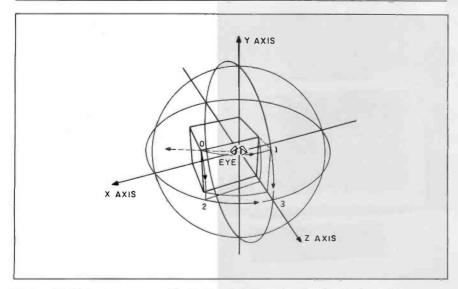
Figure 2: The vector represented by the dotted line can be aligned with the positive z-axis in either of two ways. The noncommutativity of matrix multiplication assures that the two cases require different amounts of yaw and pitch rotation.
