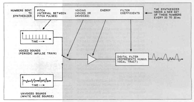
Figure 1: A linear predictive coding (LPC) model of the human voice.
