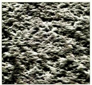
Photo 1: An electron microscope view of a normal disk area at 1330x.
