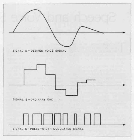
Figure 2: Two alternate forms of synthesizer output that can be used to reproduce signal A: D/A converter (signal B), in which an amplitude proportional to the voice signal at some time is held constant until the next sampling time, and pulse-width modulation (signal C), in which the pulse width is proportional to the voice signal at the sampling time. When sent through a low-pass filter, both signals get smoothed into the desired voice signal.
