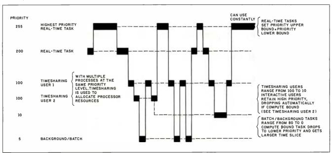
Figure A: An example of task scheduling by the UNOS operating system.
