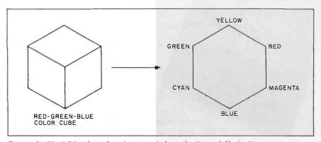
Figure 3: The RGB color cube, when viewed along the diagonal black-white axis appears as a hexagon, with primary colors (red. green, and blue) and secondary colors (cyan, magenta, and yellow) situated at the vertices.
