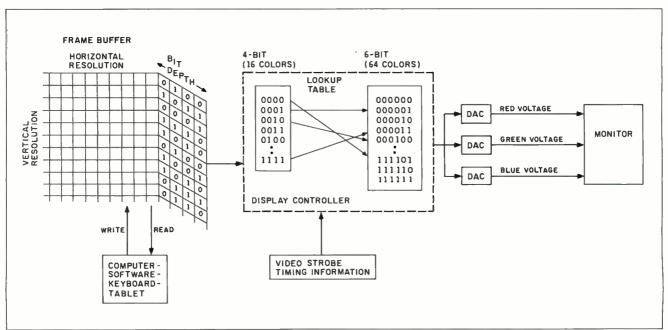
Figure 10: Basic graphics hardware architecture.
