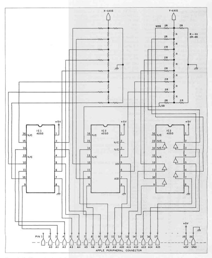
Figure 3: The D/A converter schematic diagram.
