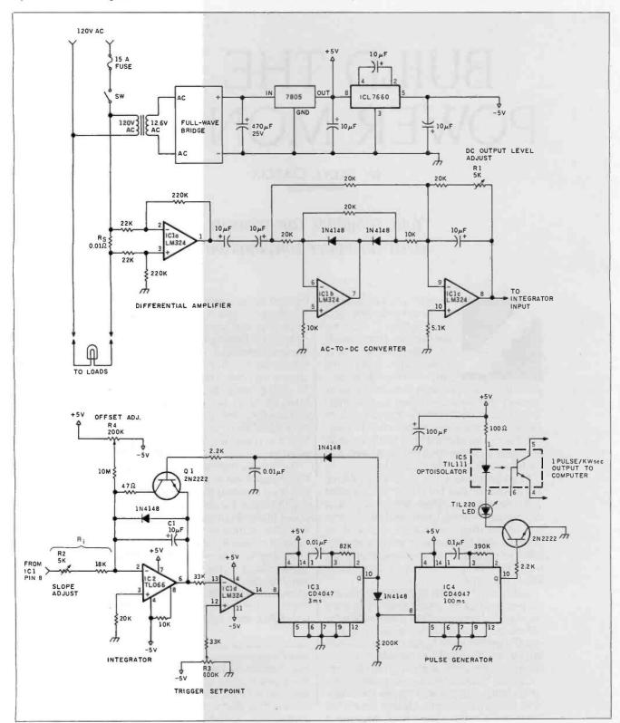
Figure 1: A schematic diagram of the Circuit Cellar AC power monitor.
