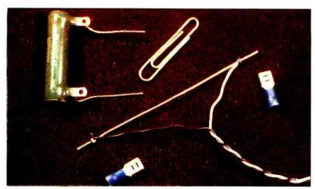
Photo 1: A 0.01-ohm sensing resistor is created from a jumbo paper clip. A load resistor combined with a regulated DC power source is used to calibrate the sensing resistor. Two wires are attached at the 0.01-ohm resistance points.
