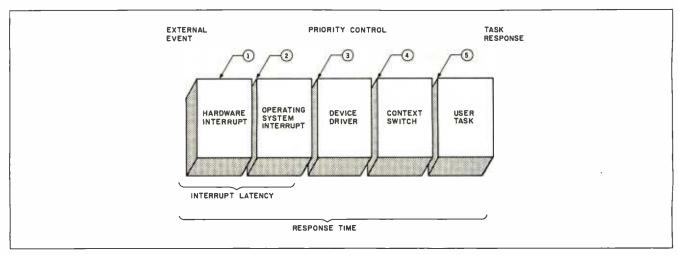
Figure B: The components of delay in a computer as it attempts to respond to a real-time event.
