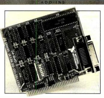
rather than as a driver. The operating system manages the GPIB as one of its system resources. The handler can control more than one GPIB-PC simultaneously. which lets you place a variety of devices on separate GPIB's to meet special needs.
