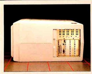
Sliding panel on right side covers serial port, video connectors, and three blank expansion slots.
