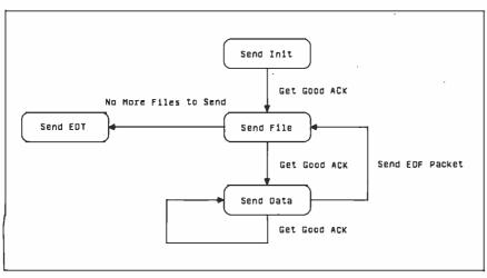
Figure 2: A simple state diagram for Kermit sending files.
