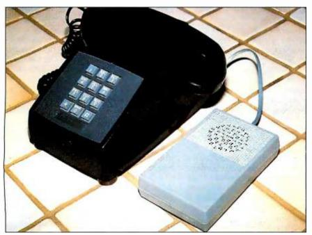
Photo 1: Whimsi-Bell attaches to the tip and ring wires in parallel with your phone.
