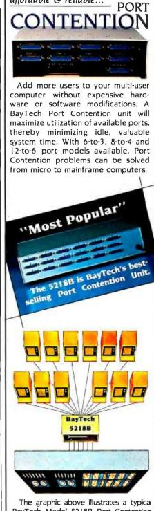
BayTech Model 5218B Port Contention application. By adding a single 5218B unit. a 6-port multi-user computer gains six additional users, thereby doubling accessibility to the computer.
