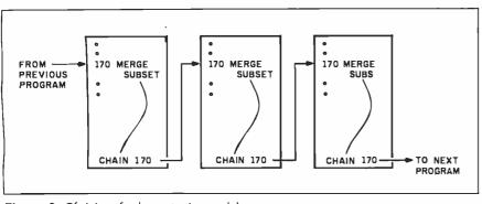
Figure 2: Chaining the demonstration modules.
