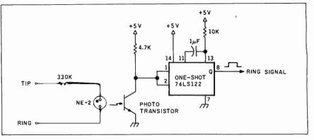
Figure 1: A simple ring-detector circuit.
