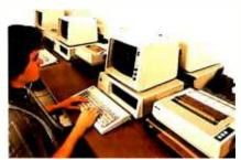
And now with Quadnet, you don't have to compromise your system to fit our system. Instead, you can easily link as few as two, or as many as 255 IBM PC's together in a hardwired network. And you can configure them almost any way you want. They can work independently of each other or share resources and peripherais.
