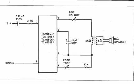
Figure 3: A typical ring detector using the TI ring-detector chip.
