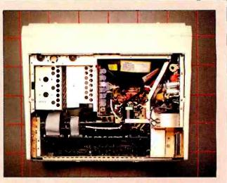
Top view reveals fixed disk (upper left), with floppy disk to its right. Power supply is at right, expansion slots at bottom.
