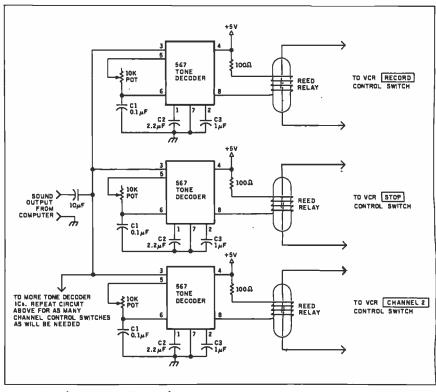
Figure 2: The computer-VCR interface circuit.
