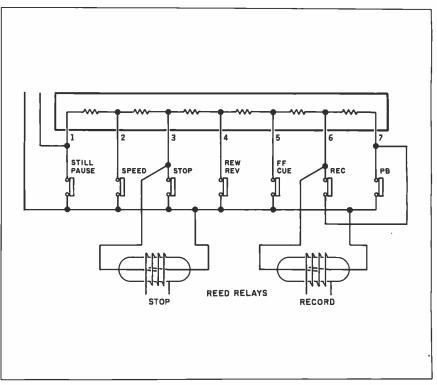
Figure I: An example of external switch connection.
