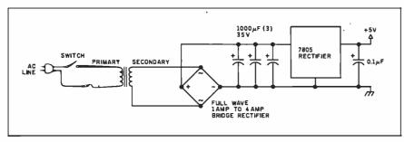
Figure 3: The regulated power-supply circuit.
