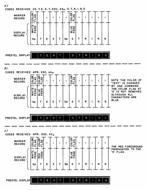
**Figure 4:** A diagram showing the immediate effect of a serial attribute and the need for attribute-marker flags. The notation 4/4 is the equivalent of 44 hexadecimal.
