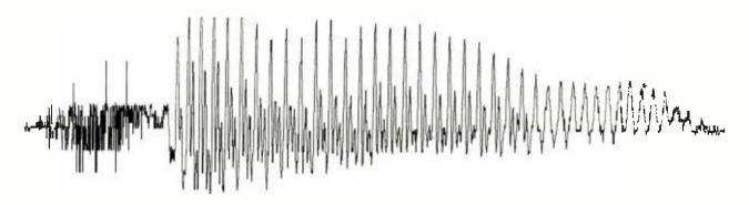
**Figure 3a:** The waveform for my utterance of the word "two" with no filtration. Corresponding to a plot of the function V(t) over time, where V(t) is the voltage of the incoming analog audio signal, it graphically depicts the sound-pressure variation at the microphone, over a 400-ms (millisecond) period while the word "two" is being spoken. This graph was produced on an Epson MX-70 dot-matrix printer and then reduced to about one third its original size.
