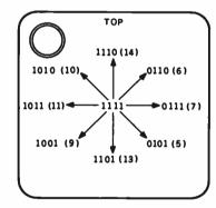
**Figure 2b:** Joystick positions and their corresponding digital codes (decimal value in parentheses).
