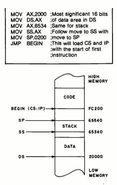
**Figure 2:** This is an example of segmentregister initialization. The SP register should be loaded directly after the SS register to make sure that the stack is pointed to correctly.
