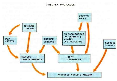
**Figure 4:** A genealogical chart of the different videotex protocols. Prestel, the British videotex protocol, was first introduced around 1976. Later systems are either based on Prestel or have added significantly enhanced graphics capabilities. The CEPT (Conference of European Posts and Telephones) standard is based predominantly on Prestel. Although the various protocols are fairly incompatible, they are being merged into a world videotex standard.
