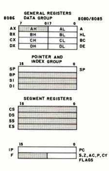
**Figure 4:** Shown is the 8080/8085 register subset of the 8086. The nonshaded registers are those used by conversion programs when converting programs from the 8080 to the 8086.
