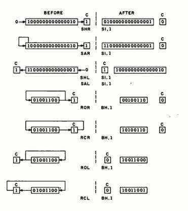
Figure 7: The shift and rotation instructions work on bytes or words. The two forms of shifts and rotations are single-bit, as shown, and a variable-bit form.
