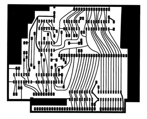
Figure 2: Layout of etched circuit board. When exposing the board, place this artwork face up on the copper-clad side.
