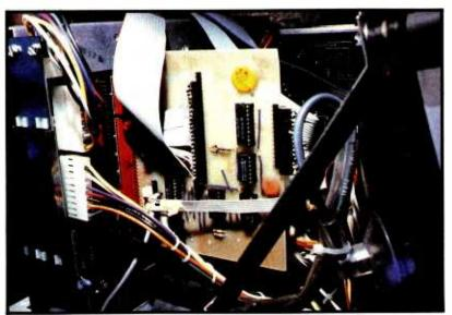
**Photo 1:** The installed interface showing cable placement. Note that the cable connectors of P1 and P2 do not connect to all the pins on the interface board because they were wired for an earlier version. Yours should fit in exact correspondence.
