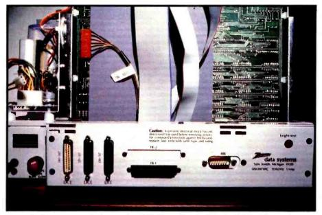
**Photo 4:** The rear panel of an updated H-89, as fitted with parallel port bus connector (leftmost) and parallel printer output (small rightmost). Male D connectors have been used here but female ones would be better protected from accidental shorts.
