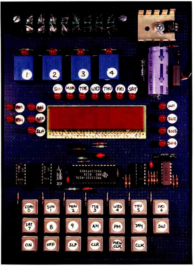
**Photo 1**: Prototype of the Circuit Cellar RTC-4 real-time controller, a unit suitable for switching low-current external devices on and off according to immediate commands or stored time-lapse event settings.
