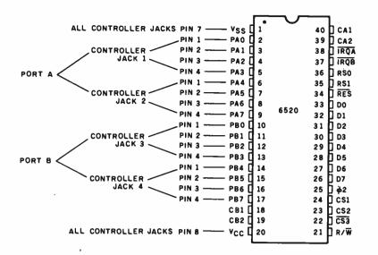
**Figure 1:** The peripheral interface adapter. Pins 2 through 17 connect indirectly through a 220-ohm resistor to the controller jack pins shown. These pins can be used as input or output.
