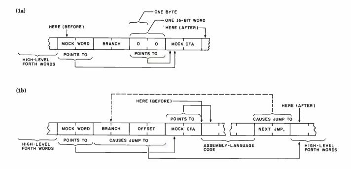
**Figure 1:** Operation of the FORTH words ASM < and FORTH <. In 1a and 1b, the condition of the dictionary is shown after the words ASM < and FORTH <, respectively, have executed. The words HERE (BEFORE) and HERE (AFTER) show the positions of the dictionary pointer before and after the given word has executed. See listing 4 and the text for details.
