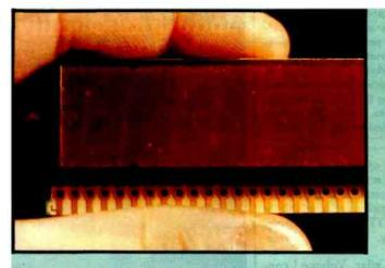
**Photo 3a:** This typical National Semiconductor 4-digit LED display (which I believe to be one of the NSB7400 series) is most frequently used in digital clocks. It consists of three parts: a plastic circuit board with LEDs bonded to the circuit traces, a plastic reflective digit form, and a red lens cover.
