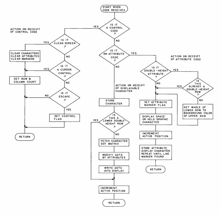
Figure 3: A flowchart of the Prestel decoding process. Each code received causes one pass through the flowchart.
