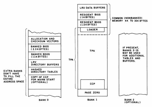
**Figure 2:** The CP/M Plus banked-memory organization. Up to 16 banks can be supported, although only two are required for operation of the banked version. Bank 0 contains the bulk of the BDOS and BIOS as well as all the extra buffers. Bank 1 is used to run programs and contains a small part of the BIOS and BDOS in common memory. The block of common memory must be at least 4K bytes long and must reside at the top of the address space.
