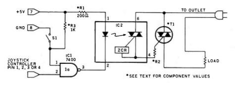
**Figure 4**: This solid-state relay isolates a computer from up to 7500 V, produces no EMI when switching, runs quietly because it has no moving parts, and connects directly to an Atari 400/800.
