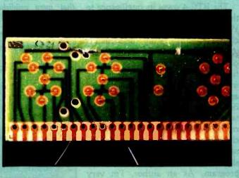
**Photo 3d:** Finally, I drilled holes and soldered wires to the individual digit connections.
