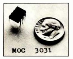
**Photo 1:** The MOC3031 is the heart and brains of the solid-state relay described in the text. Don't let its small size fool you; it can protect a computer from voltage spikes up to 7500 V. It costs about \$2 from any Motorola distributor.
