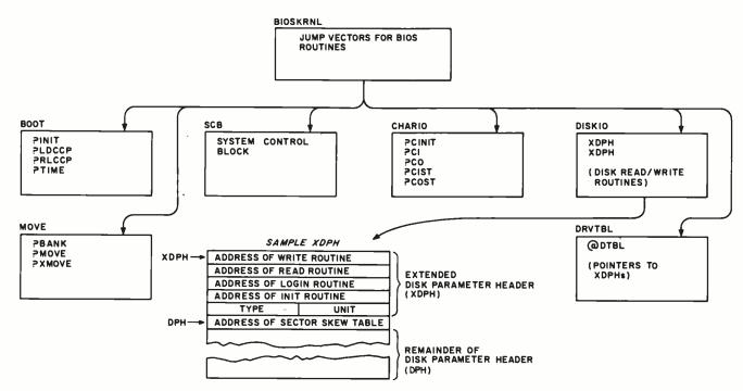
**Figure 4:** The linkable modular BIOS can be broken into several easy-to-maintain segments, as shown here, allowing a manufacturer to supply a disk I/O module with its disk-controller board without having to worry about making the rest of the BIOS compatible. In the same way, character I/O devices can be separated into modules to simplify system integration. Furthermore, breaking the BIOS into logical sections makes it easier to maintain and modify.
