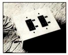
**Photo 2:** The chassis of the four-channel SSR prototype the author built contains a control cable, which plugs into any Atari 400/800 controller jack and a power cord.
