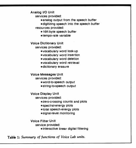
cation functions to investigate the structure and content of digitized speech. Furthermore, the program units are designed so that they can not only serve Voice Lab but also provide synthesized-speech output from virtually any program running under the p-System. They allow my computer to speak with a limited vocabulary and provide a set of tools for investigating computer speechgeneration and recognition.
