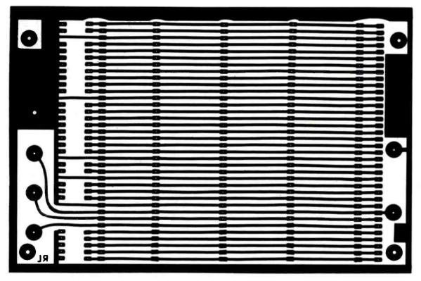
**Figure 3:** Layout of the bus board. When exposing, the "scoops" in the ground perimeter are at the top, and the power supply pads are on the left. Large pads in the corners are for mounting-screw holes. The lead holes in some lower pads have been blocked out; open these with a pin on transparency before exposing.
