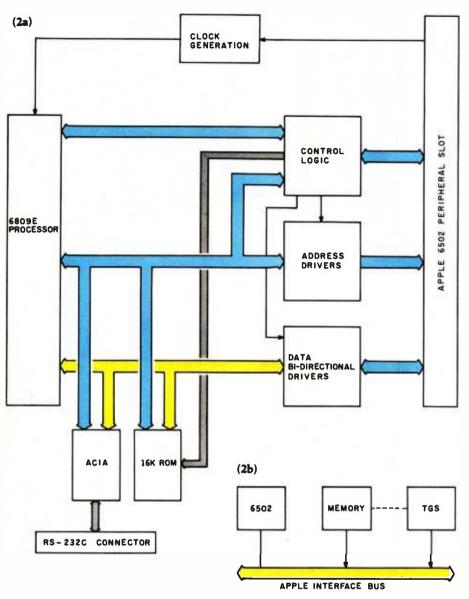
**Figure 2:** Block diagrams of the Telidon Graphic Systems card (figure 2a) and how it interfaces to the Apple II (figure 2b).
