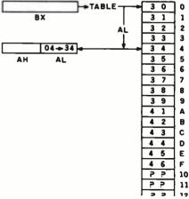
**Figure 5:** This program uses the XLAT instruction to convert a single hexadecimal digit to its ASCII equivalent (e.g., to convert the value 04 into 34 hexadecimal, which is the ASCII code for the character "4"). XLAT uses the contents of the AL register as a displacement into a lookup table pointed to by the BX register. The contents of the location then replace the contents of the AL register. The values in the table are in hexadecimal.
