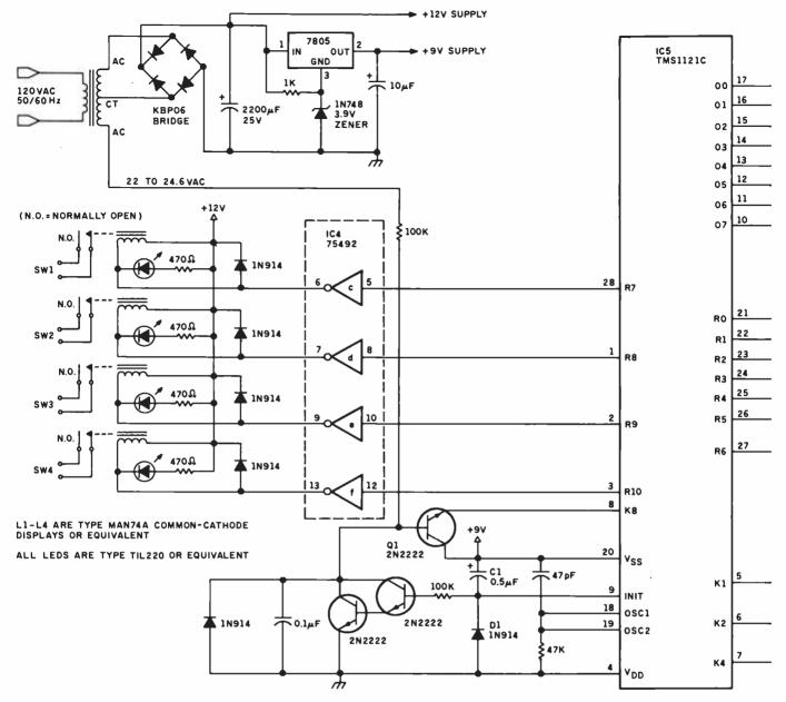
**Figure 3:** Schematic diagram of the RTC-4. A type-MAN74A common-cathode LED display module is specified, a type somewhat different from the junk-box unit used in the prototype (see text box, page 34). Please note the position of the MSD (leftmost digit) and the LSD (rightmost digit) when wiring the unit.
