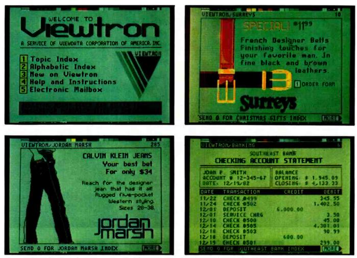
**Photo 4:** Examples of the pictures created on the Viewtron system being run by Knight-Ridder newspapers and AT&T. This system is based on NAPLPS and is capable of some very impressive graphics. (Copyright © 1983 by Viewdata Corporation of America Inc., used by permission.)
