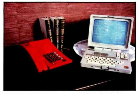
**Photo 3:** A terminal that is used in the French Teletel system for electronic access to phone directories and other services.
