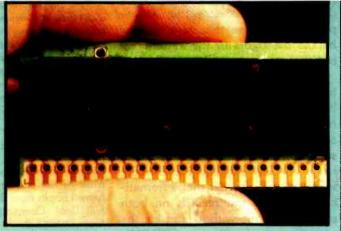
Photo 3b: The LED display with the lens cover removed.
