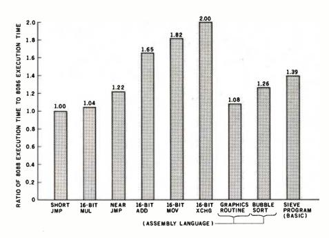
**Figure 2:** Performance ratios for selected pure and real-world benchmarks. The ratios are obtained by dividing the execution time of the 8088 for that benchmark by the execution time of the 8086. The first six bars are derived from the pure benchmarks of table 2; the last three are from the real-world benchmarks of table 1.
