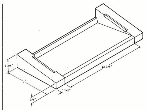
**Figure 2:** Keyboard case frame. Dimensions for the various pieces are provided in inches. Most pieces can probably be cut from scrap lumber.
