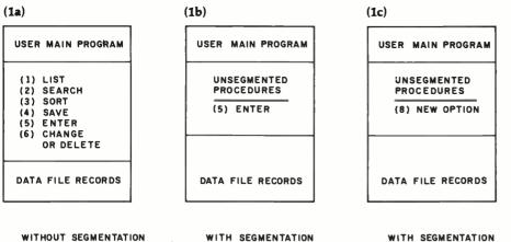
**Figure 1:** With segmentation, not only can more records be included, but the application program can be expanded to include more capabilities.
