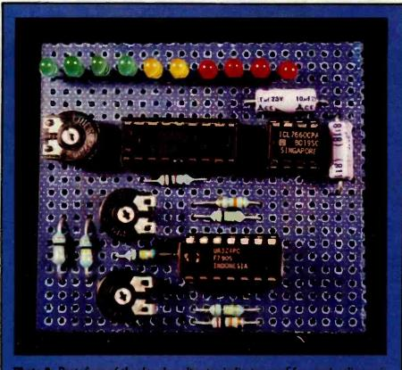
Photo 2: Prototype of the decade-voltmeter indicator used for precise diagnosis of the state of en RS-232C line.
