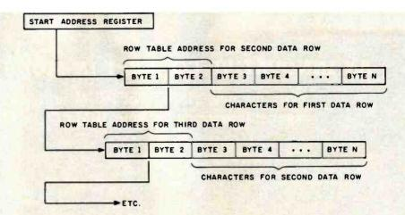
Figure 3: Linked-list row-table format. The start address register points to the address for the second data row. The first 2 bytes of that data row point to the address of the next data row, and so on.
