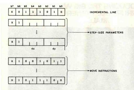
Figure 2: Structure of the Incremental-Line instructions. The first byte indicates that a series of Incremental-Line instructions will follow. The next series of bytes indicates the size of the relative coordinates dx and dy to whatever resolution is desired. The last series of bytes is composed of the actual 2- and 4-bit drawing instructions.
