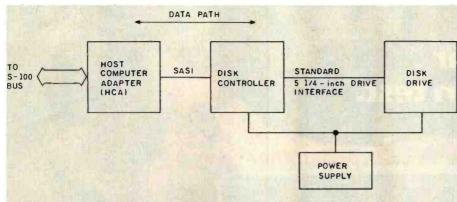
Figure 1: Winchester disk-drive subsystem block diagram.
