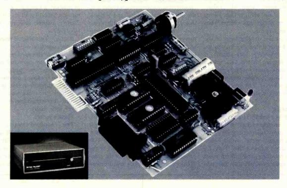
INTEX-TALKER, the new second generation text-to-speech synthesizer with unlimited vocabulary, an advanced text-to-speech algorithm and 64 levels of inflection provides a new high level of speech intelligibility.
