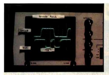
Photo 4a: The Z80 clock runs at 3.58 MHz, and the memory clock at 14.5 MHz. An op-code fetch (a short Read with M1 high) sets two request flags. The first  $\overline{RAS}$  pulse is the actual op code being fetched, and the one on its heels is a "hidden refresh." The time elapsed for each vertical line on the scope face is 200 ns. The horizontal smear on  $\overline{RAS}$  is the 69-ns latency time of the cycle generator.
