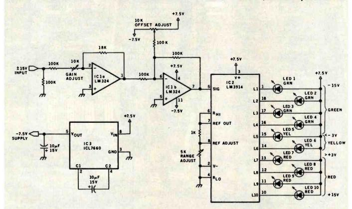
Figure 5: A decade-voltmeter circuit. This more precise indicator may be substituted for the twelfth indicator in the breakout box of figure 4a. It lights up in one of three colors depending on the voltage present on its input.
