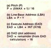
Figure 1: Four equations to locate an individual dot address.
