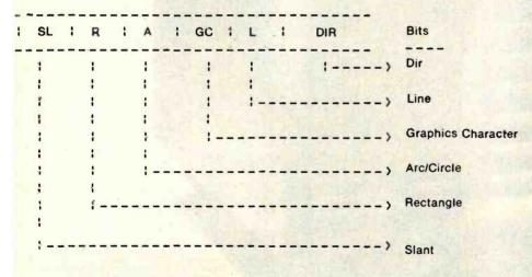
Figure 5: The layout of the FIGS (figure specify) command.
