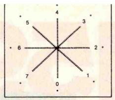
Figure 2: A direction map for controlling pixel-drawing direction.
