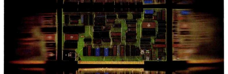
A hard disk and cartridge tape controller together on one board? Magic? Not really. It's Teletek's HD/CTC. The hard disk and cartridge tape drive controller provide the support necessary to interface both rigid-disk drives and a cartridge tape deck to the S-100 bus.
