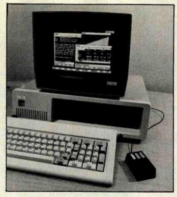
Prototype of Visicorp's Visi On integrated applications environment. Note the multiple video windows and mouse. Since this photo was taken, Visicorp has changed to a two-button mouse.
