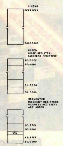
Figure 3: Three methods of addressing memory. The Linear method arranges a contiguous memory area. The Paged method organizes memory into blocks or pages of a prescribed length. The Segmented method gives each user or program a specific area in memory. Both the Paged and the Segmented method give the programmer access to only a small portion of memory.
