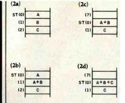
Figure 2: The effects of instructions on the register stack.
