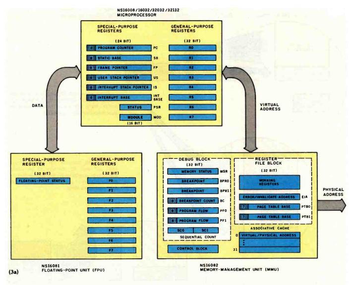
Figure 3: Component interconnection in the NS16000 family. Figure 3a shows the logical interconnection of the microprocessor and its memory-management and floating-point units, while figure 3b gives an overview of the physical interconnections.
