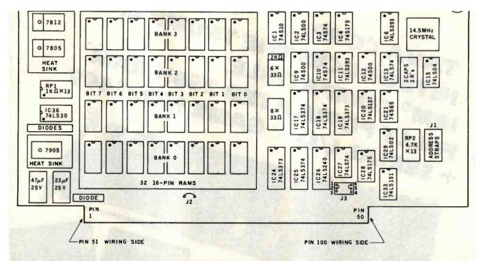
Figure 6: Layout of ICs on wire-wrap circuit card. Note that, in some places, resistors and capacitors are shown in IC-like blocks.
