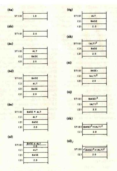
Figure 6: The status of the NPX stack during operation of the program in listing 1.
