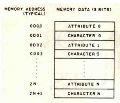
Figure 4: The Attribute Assemble mode lets the programmer create a pseudo 16-bit word that describes both the character and its attributes (see text).
