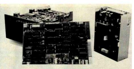
Photo 3: The Winchester disk-drive subsystem components before assembly.
