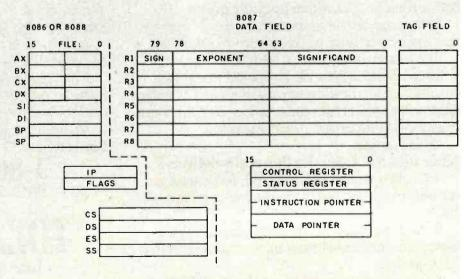
Figure 1: The NDP register set of eight 80-bit registers.
