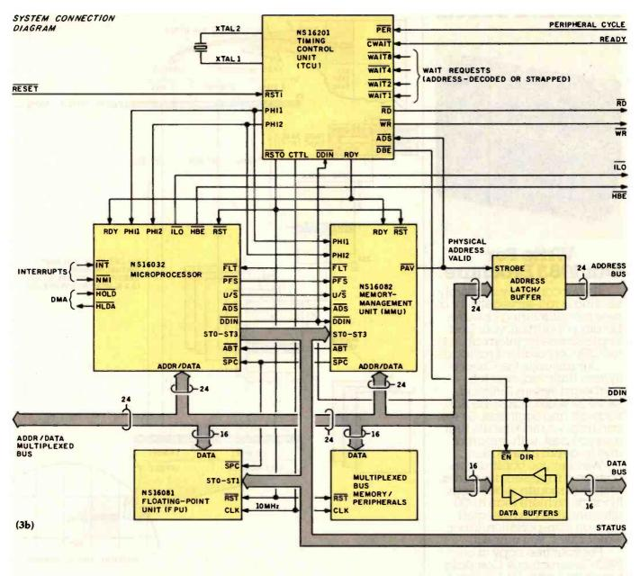
ory-management unit. If the memory-management unit decides that the information resides in main memory, it translates the virtual address to the physical address directly, allowing the microprocessor to operate directly on the memory.
