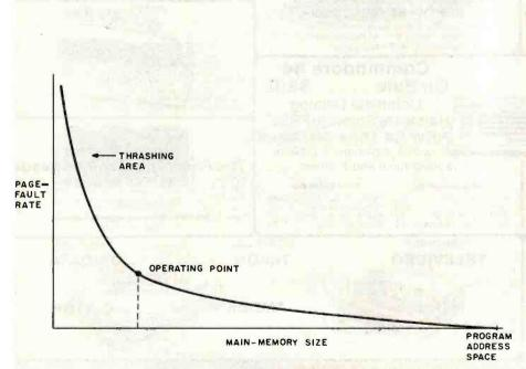
Figure 4: A graph showing how the page-fault rate (i.e., the rate of accesses to pages not present in main memory) is related to the size of main memory. The operating point is the memory size sufficient to hold a program's most frequently accessed routines—its working set. Adding memory past this point has little effect on the page-fault rate. Of course, as the needs of a program change, the operating point will shift.
