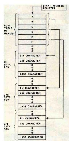
Figure 2: Contiguous row-table format. Each data row (screen line) is stored contiguously within memory. The start address register points to the first row table.
