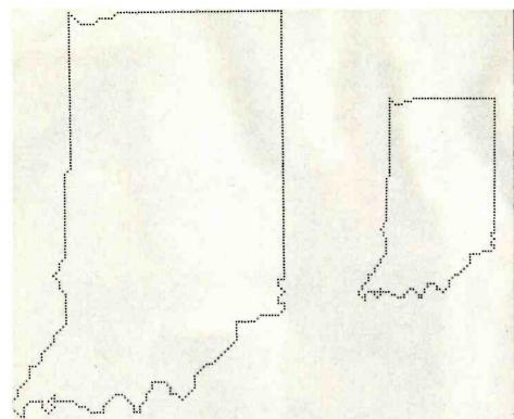
**Figure 1:** An example of an incremental-line drawing. The size can be changed simply by changing the values of the relative coordinates dx and dy. This drawing was done on a Diablo 630.
