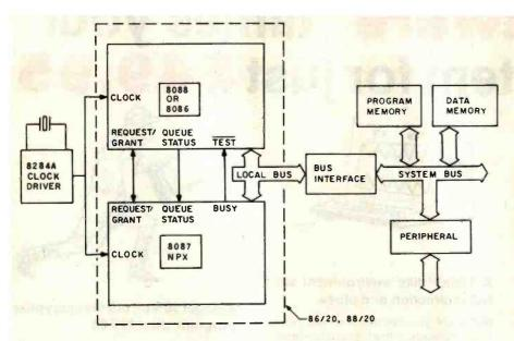
Figure 5: The interface and communication lines.
