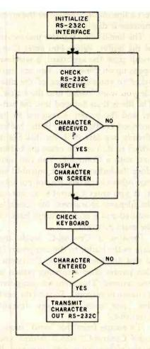
Figure 1: Operation of the main section of the terminal program. The RS-232C board is controlled from the program.
