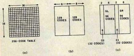
Figure 5: With an 8-bit code, 256 combinations are possible. These can be represented on a 16 by 16 table (a). For convenience, this large table can be divided into two 128-code tables (b). Each of these 128-code tables can then be further subdivided into a 32-code table and a 96-code table (c).
