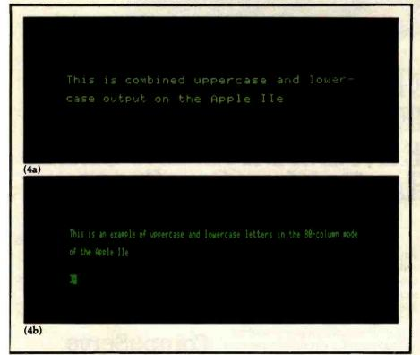
Photo 4: The Apple IIe video display. Photo 4a is an example of the 40-column text display showing both uppercase and lowercase characters available. Photo 4b shows the Apple IIe 80-column display. The plus sign within the cursor shows that you are in Escape mode, which provides expanded editing and cursor-control functions.
