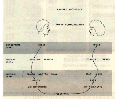
Figure 4: If the conversation in figure 3 were conducted over a telephone, we could interpret this as a change of the physical layer. The advantage of layered protocols is that one layer can be changed without affecting the other layers. Although the physical level here has been changed, the logical level—English—is unaffected.
