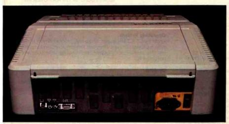
Photo 2: The rear panel of the Apple Ile. Instead of the plastic slots found in the Apple II, the Apple IIe's metal back panel is designed to mount 9-pin, 19-pin, and 25-pin D-type connectors in precut recesses, providing more reliable connections and reduced RF interference. The built-in game-paddle connector has also been changed to a 9-pin D-type; however, the older-style connector is still available inside the case to accommodate existing devices.
