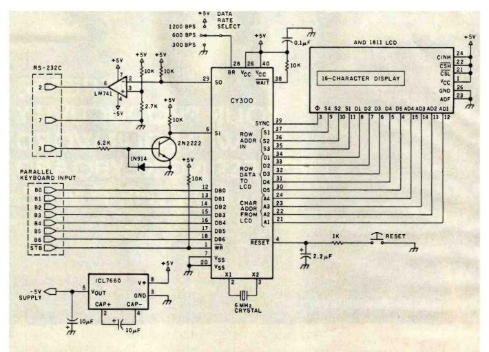
Figure 5: Schematic diagram of a single-line LCD computer terminal built around the CY300 and the AND 1811 display module. This style of RS-232C driver circuit was designed to use minimal  $\pm 5$ -V power, so it's not guaranteed to work through a long cable to the host computer.
