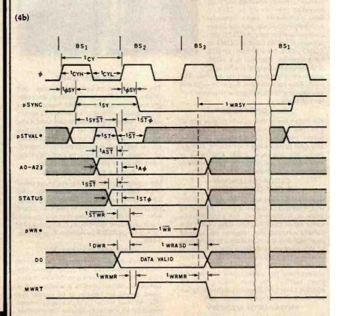
Figure 4: Timing diagrams for basic bus cycles. Figure 4a shows a read cycle; figure 4b shows a write cycle; and figure 4c shows the timing required for the RDY, XRDY, and SIXTN\* signals (when pSYNC is false, RDY and XRDY are tested only when the master is in a wait state).
