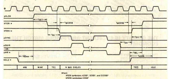
Figure 3: Diagram of the timing relationships for temporary-master access to the bus.
