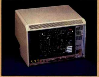
Inside the Lisa computer. Note the three connectors for expansion boards.
