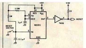
Figure 1: A circuit diagram for the Reset switch, which has been added between pins 1 and 2 of the 555 IC timer.
