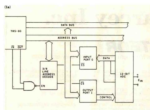
Figure 1: Diagrams of the complete interface circuit. In figure 1a, a block diagram of the circuit shows how the I/O port address is decoded and how the eight data lines are partitioned into an input bus and into an output bus. Figure 1b is a schematic diagram developed from figure 1a. Note that all eight data lines are used when transferring data to the computer and only three lines are used by the computer to control the ADC.
