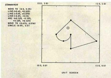
Figure 7: The unit screen of NAPLPS. All coordinates are represented as fractions between 0.0 and 1.0. The figure on the screen was drawn with the commands listed on the left. The advantage of this coordinate scheme is that it can be easily implemented on display screens of various resolutions and sizes.
