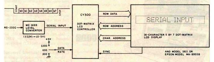
Figure 4: Block diagram of a typical serial-input arrangement used by the CY300.
