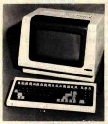
Protected fields, optional 2nd page of memory, visual attributes, tilt-swivel screen (non-glare P31 green), 25th status/user line, time of day, can emulate 912/920, R\$232C printer port, 50 Baud to 19.2KB., 8x10 character resolution, switchable character sets, function keys self test.
