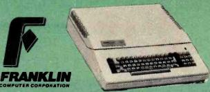
The Franklin ACE 1000 includes 64K RAM, upper/lower case character set (40 columns), hi-res graphics, numeric keypad, 8 peripheral slots, joystick/paddle connectors, and a built-in cooling fan. The Franklin ACE 1000 has full hardware/software compatability with all existing Apple II\* products.
