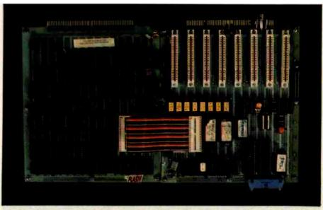
**Photo 7:** The Apple IIe engineering prototype wire-wrap boards. The custom MOS IOU and MMU ICs are emulated with discrete logic on the board to the left, while the Apple IIe main board prototype is on the right.
