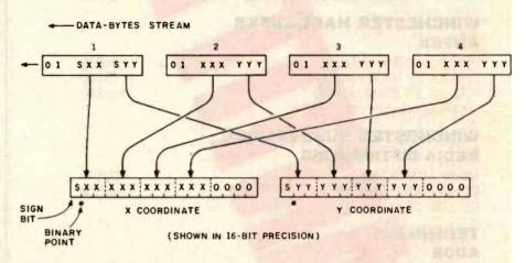
Figure 11: The data bytes shown in figure 10 can be combined to specify coordinates of almost unlimited resolution. Here, 4 data bytes in the two-dimensional mode are combined to form a pair of 12-bit coordinates. This would support a resolution of 2048 by 2048.
