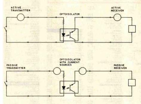
Figure 5: Active-to-active and passive-to-passive converters.
