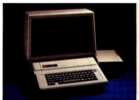
Photo 1: An Apple Ile system made up of the Apple Monitor III, the Apple Ile computer, and a Disk II 51/4-inch floppy-disk drive.
