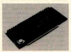
Where it all started: pictured is the popular Multiuser I, Macrotech's first product. This widely used board provides 256 Kbytes of dynamic ram with 4K page memory mapping (called M³), 8/16 bit operation, 24 bit addressing and byte parity checking.
