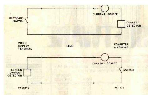
Figure 4: Computer-to-terminal interface using current loops.
