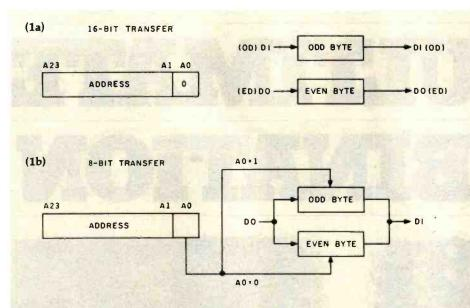
Figure 1: Data transfers as performed according to the IEEE-696 standard. In figure 1a, a 16-bit transfer is shown using all of the available data lines. Data whose least-significant address bit is 0 is considered even, while data whose least-significant address bit is 1 is considered odd. Figure 1b shows how the odd and even bytes are employed during an 8-bit-wide transfer of 16-bit data (called a byte-serial transfer).
