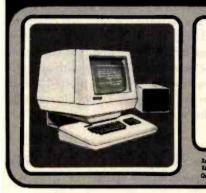
820-II FEATURES: 4MHz. Z80A, CPIM BASED, 64K RAM, 12" HI RES SCREEN (24 x 80), DO DISK CONTROLLER, THIN LINE GRAPHICS, ENHANCED SCREEN FEATURES (HIL INTENSITY, REVERSE VIDEO, FLASHING CHARACTERS), TONE GENERATOR, 2 RS-232 PORTS, ONE PARALLEL PORT, ALSO BOOTS AS INTELLIGENT TERMINAL.
