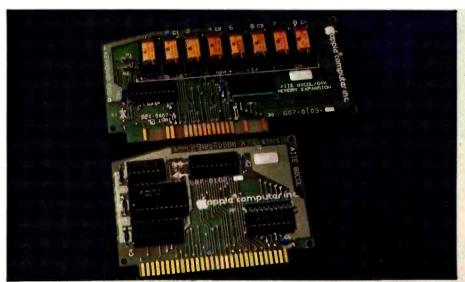
Photo 5: The Apple Ile 80-column text card (bottom) and extended memory 80-column card (top). The 80-column text card provides an additional 1K-byte text/low-resolution graphics display page, while the extended memory 80-column card duplicates the entire Apple Ile 64K-byte address space.
