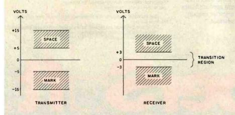
Figure 1: RS-232C signal levels.
