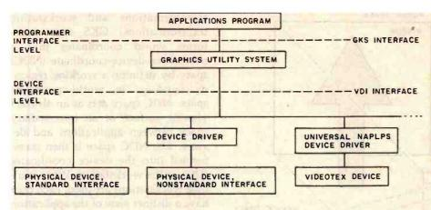
Figure 1: The two main levels of graphics standardization are the programmer and device-interface levels. The Graphical Kernel System (GKS) provides a standard interface between the application program and graphics utility programs. The Virtual Device Interface (VDI) standardizes the interface between graphics utilities and device
