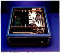
A LMC MC68000 system with 1.5 megabytes of error-correcting RAM.
