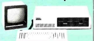
The Columbia MPC features full compatability with all IBM PC hardware and MSDOS. MSBASIC. CP/M 86, FORTRAN, PASCAL, COBOL, CBASIC 86, etc. Comes with 128K RAM, two double-sided drives (320K perdrive), two serial ports. one printer port, and one keyboard port. Eight peripheral slots remain for maximum expansion of the system, including multi-user configurations.
