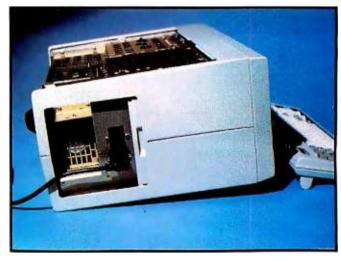
Photo 3: A sliding door conceals a storage compartment, the power switch, and the ventilation fan.
