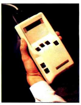
The Microwriter is one of the most interesting devices I saw at the show. A one-handed dataentry unit, it can be hooked up to a printer or a microcomputer, and it even has some limited word-processing features. You enter data by pressing down and releasing certain combinations of the six buttons. At £557.75 (less than \$1000). it's a bit expensive, but its portability and one-handed operation make it desirable to some.
