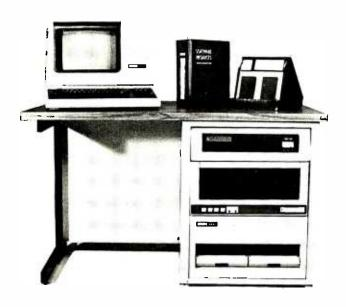
**CI-MWS03-SB** — LSI 11/2 computer workstation. LSI 11/2 CPU, 64KB Memory, power supply, KEV 11, in 16 slot rack mountable chassis. 2 port serial I/O. CRT terminal. 1 mega byte floppy disk system. Desk-
