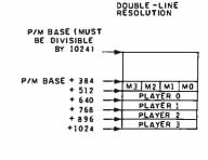
Figure 2: Memory allocation for the player-missile graphics. Definitions for the shape and vertical position of both the players and missiles are kept in this area of memory.
