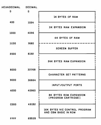
Figure 1: The VIC-20 memory map shows the organization of the VIC's memory with starting addresses in both decimal and hexadecimal for each block.
