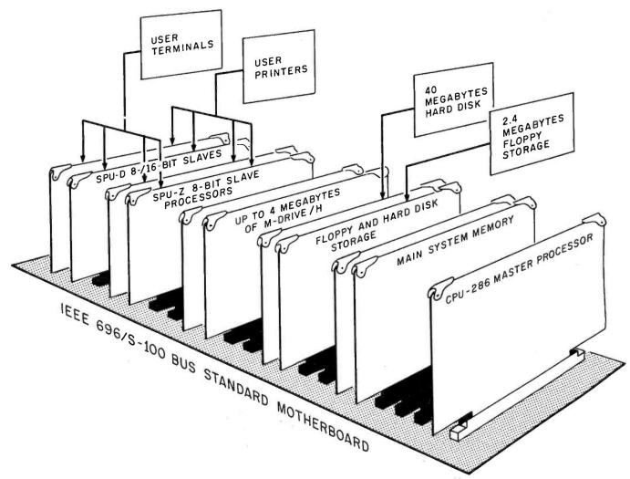
Figure 1: A typical system configuration with a CPU 286 master processor (based on Intel's iAPX 286) with its main system memory and floppy- and hard-disk storage. Up to 4 megabytes of M-Drive/H solid-state disk is supported by the system for ultrafast access times. Any mix of up to sixteen 8-bit or 8-/16-bit slave processors may be plugged into the system. (Figure provided courtesy of Compupro Systems.)
