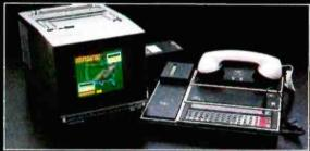
The Quasar mainframe has a complete range of intelligent peripherals including a new 40-Character Printer, Telephone Modem/Cassette Interface, RS232 Interface, Color TV Adaptor, I/O Adaptor that works with up to 6 peripherals.
