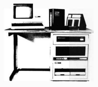
**CI-MWS23-MB** — LSI 11/23 computer workstation. LSI 11/23 CPU, MMU, 256KB Memory, power supply, in 16 slot rack mountable chassis. CRT terminal. 10 mega byte cartridge disk system. 4 port serial I/O. Desktop workstation .....**\$10,995.00**
