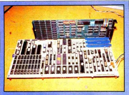
**Photo 3:** Prototype of the MPX-16 being tested for compatibility with the I/Oexpansion bus of the IBM Personal Computer. A Quadram Quadboard (an expansion card for the IBM PC that contains 256K bytes of memory, a serial port, a parallel port, and a real-time clock) is inserted in one of the MPX-16's slots. It works!
