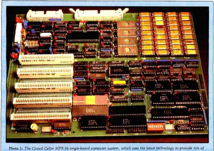
**Photo 1:** The Circuit Cellar MPX-16 single-board computer system, which uses the latest technology to provide lots of low-cost computing power. The five-layer printed-circuit board contains 120 integrated circuits including most common peripheral-device interfaces; furthermore, any peripheral-device card intended for use with the IBM Personal Computer can be plugged into one of the I/O-expansion slots. There are nine slot positions, but only five sockets are installed initially.
