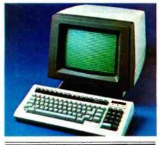
VIDEO DISPLAY TERMINAL FROM SHINLEE CORP -- Shinlee's T88 terminals is microprocessor-based, teletype-compatible model with detachable keyboard capable of displaying the complete ASCII set. The 12inch screen will accomodate 2,000 characters in an 80 x 25 matrix. The T88 is compatible with most currently-available terminals. Size: 345mm (H) x 370mm (W) x 295mm (D). The Shinlee Corp, 2/F, 372 Lin Sen North Road, Taipei, Taiwan, ROC. TLX: 11154 SHINLEE
