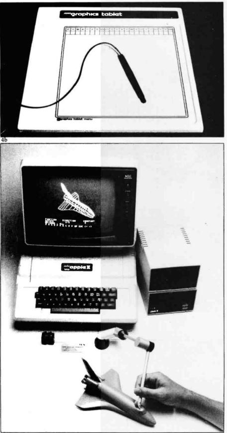
**Photo 4:** Digitizers. Pictured are the electromagnetic Apple Graphics Tablet (photo 4a, courtesy of Apple Computer Inc.) and the mechanical three-dimensional digitizer from Micro Control Systems (photo 4b, courtesy of MCS). Manufacturer addresses can be found in the vendor text box.
