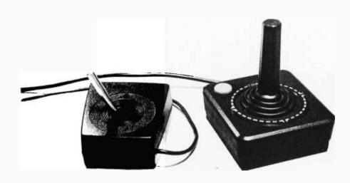
**Photo 3:** Joysticks. At the left is the Radio Shack Color Computer joystick (resistive); at right is the Atari joystick (switch type).
