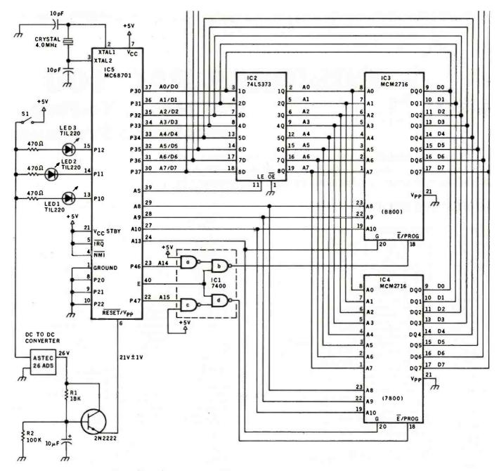
**Figure 2:** Programmer for the MC68701. The simplicity of this inexpensive circuit means easy construction and use. In combination with the software provided in listing 1, LEDs in the programmer can indicate that the EPROM is initially erased and that the newly stored data pass or fail a verification test.
