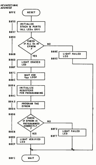
**Figure 4:** Flowchart of the programmer software called MINPRG. The program is shown in listing 1.
