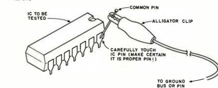
Figure 11: After building the GPIO, the 24 lines may be tested easily by a LED/resistor tester for outputs and by grounding inputs.
