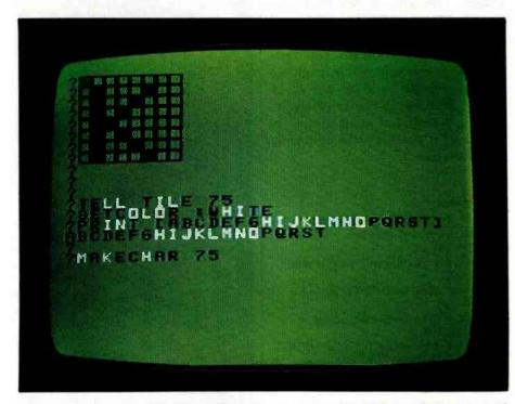
**Photo 4:** Tile recoloration and redefinition. As this photo illustrates, both the shape and color of a tile (character) can be changed. Notice that changing the color of a single tile also changes the color of the other seven tiles in the same group.
