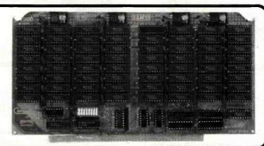
The days of "Out of Memory" are gone at last! CompuPro has introduced the largest static S-100 IEEE/696 RAM board ever to be produced. The RAM 21 is arranged either as a 128K x 8 bit wide or 64K x 16 bit wide board, using a high speed, ultra low low power proprietary static RAM. CompuPro has also included 24 bit addressing for up to 16 megabyte capability and power consumption so low your mainframe will never know it's there!
