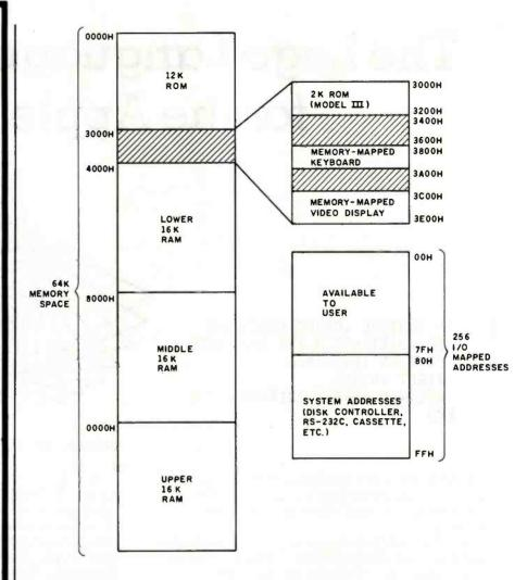
**Figure 2:** The Models I and III have 64K bytes of addressing space. Some system devices are memory-mapped and use dedicated addresses within the 64K bytes. Other system devices use the I/O-mapped addresses hexadecimal 0 through FF.
