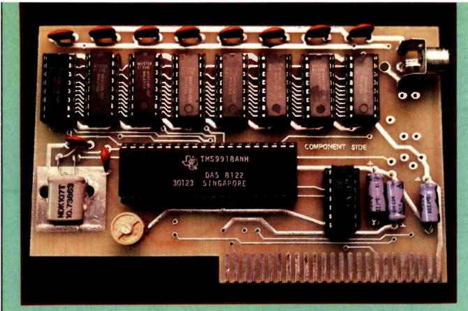
Photo 4: The Circuit Cellar E-Z Color Graphics Interface; a prototype printed-circuit board is shown. This typical TMS9918A color graphics interface is interfaced to the Apple II microcomputer bus with a minimum of components.
