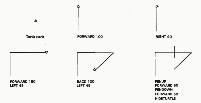
Figure 1: Moving the turtle with a simple sequence of Logo commands. FORWARD moves the turtle in the direction it is facing. RIGHT and LEFT rotate the turtle. PENUP and PENDOWN raise and lower the pen—the turtle leaves a trace when it moves with the pen down.
