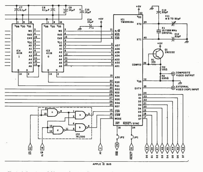
The circuit shown is intended for use with an Apple II computer, with the circuit board plugged into a slot on the motherboard (usually slot 4), but other versions of the circuit for S-100-bus computers and the IBM Personal Computer are under development. The E-Z Color Graphics Interface may also be adapted for use with other computers.
