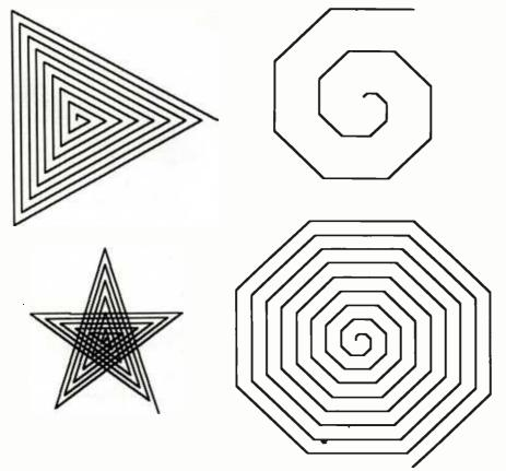
Figure 3: Figures created using POLYSPI. A variant of POLY (see figure 2), the program takes advantage of recursion to increase the turtle's FORWARD step each time the procedure calls itself. The result is a polygonal spiral. As with POLY, varying the ANGLE input changes the symmetry of the pattern.
