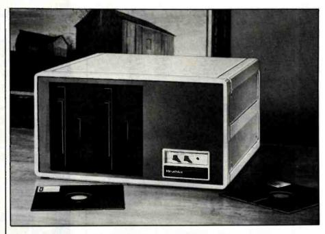
Photo 1: Front view of the Heath/Zenith 47 dual floppy-disk system.
