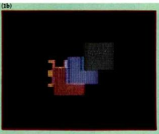
Photo 1: A step-by-step illustration of the use of sprites and the concept of plane priority. The yellow turtle (sprite 3) is programmed to pass from left to right past the green box (sprite 0), the blue box (sprite 1), and the red box (sprite 2). The transparent pattern plane and backdrop cause the background to be black.
