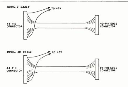
Figure 9: The cable for the Model I is different from the Model III version. The Model I version uses a 40-pin edge connector, while the Model III version uses a 50-pin edge connector. Both versions use a 44-pin connector for the prototype board.
