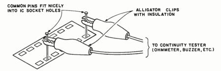
Figure 7: After GPIO board fabrication, the wiring connections should be checked out. Two common pins and a continuity tester or ohmmeter facilitate checkout.
