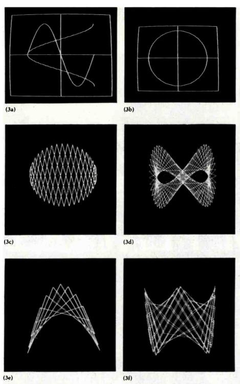
Photos 3a-3f: Six more designs from the PLOTTING microworld. The author regards designs made from sine and cosine functions as neat phenomena; i.e., phenomena inherently interesting to observe or interact with. In each design, a procedure calculates a screen location with x as a sine function of an angle value, and y as a cosine function of the same angle. The turtle draws a line by moving from one calculated location to the next.
