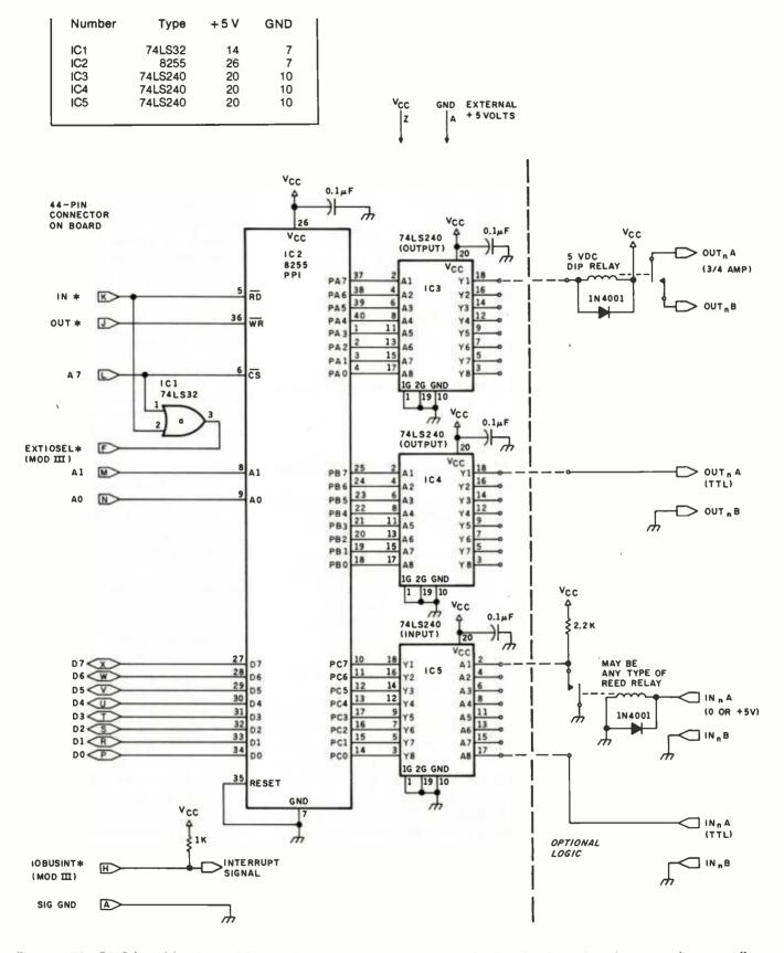
**Figure 5:** The GPIO board for the Model I and III uses an Intel 8255 Programmable Peripheral Interface chip as a 24-line controller. Sixteen of the lines are outputs and control 74LS240 drivers. Eight of the lines are inputs.
