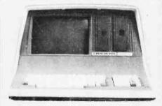
64K Double or Quad Density units available. Uses two Z-80 CPU's. Commercial-type terminal with 12" monitor. Dual double density minifloppies. Over 350 kilobytes of storage (twice that with quad density drives). Two serial RS232 ports, I/O ports standard. Comes with CP/MTM 2.2 operating system. MiniMicroMart can supply a wide range of CP/M development and application software.
