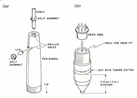
**Figure 2:** Modifications made to Schaefer No Nonsense pen barrel. With contents removed, the pen becomes a home for the HEDS-1000 sensor. The cable and indicator LED are affixed to the pen barrel (2a), while the sensor is mounted to the pen tip (2b).
