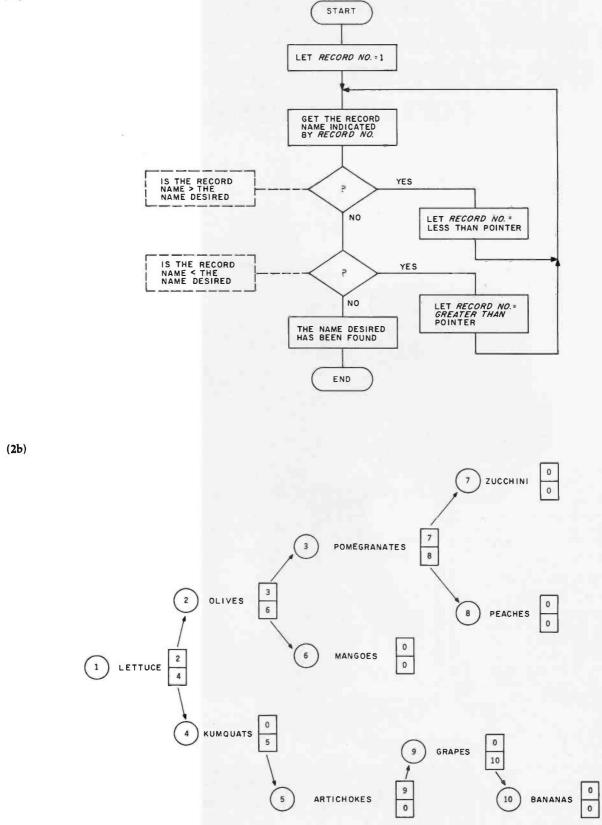
Figure 2: Traversing the PDQ tree. Figure 2a is the flowchart for a method of searching a tree. Note its simplicity when compared to the binary-search method of figure 1a; searching the tree requires fewer steps and calculations. A sample PDQ tree (of the same data used in figure 1b) is shown in figure 2b.
