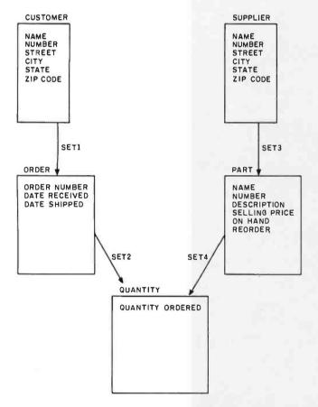
Figure 1: A data structure representing the information needed to handle the data-processing tasks of the Nibble Computer Store. The boxes represent record types. The names within boxes correspond to the data items that make up the records. The lines between boxes represent set-types—ordered groupings of related records. SET3, for example, associates parts with their suppliers.
