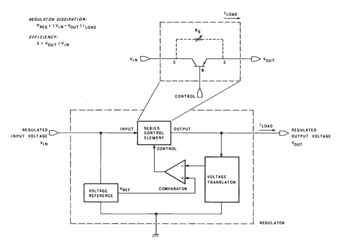
**Figure 1:** Block diagram of a typical linear series voltage regulator, such as the LM317, LM340 or 7805. The series regulator acts as a varying resistance, dissipating excess power as heat to maintain a constant output voltage.
