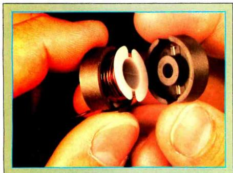
Photo 3: Winding the inductor for the switching supply of figure 6a. The turns of wire are neatly wound around a plastic bobbin, evenly distributed.
