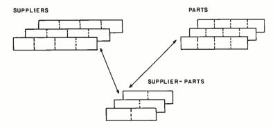
**Figure 1:** A visual representation of files in a network data-base management system. The user can move through the network of files. For example, a user positioned at part number 124 in the Parts file can find out all the suppliers of that part by moving through the Supplier-Parts file to the Suppliers file.
