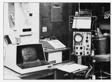
**Photo 1:** View of the laboratory microcomputer, showing the Soroc video console, Horizon II computer, interface box, and oscilloscope and strip-chart recorder used for graphic display of data. Plant growth transducers and other instruments located in a controlled-temperature room behind the computer are plugged into the interface box on top of the Horizon.
