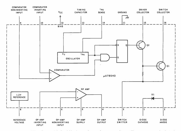
Figure 3: Functional block diagram of the Fairchild 78540 switching-regulator integrated circuit. This component may be obtained from the supplier listed on page 45.
