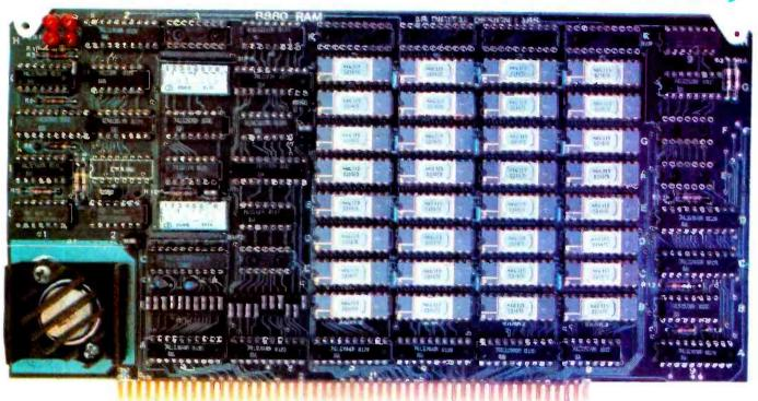
**FEATURES •** Byte or Word Width Operation • Extended Addressing or Port Select • 100 ns Access and Cycle Time (Maximum) • Low Power Consumption • IEEE 696 Standard • Four Layer Board • Byte Parity Option
