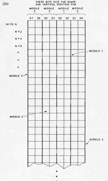
Figure 2: The player-missile area. Information on the shape and vertical position of the players and missiles is kept in a block of memory. The allocation for single-line and double-line player-missile areas is shown in figure 2a. Figure 2b shows how one area can store the shape and position of four missiles.
