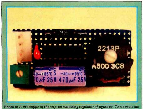
Photo 6: A prototype of the step-up switching regulator of figure 6a. This circuit can be adjusted to produce voltages between +8 and +28 volts.
