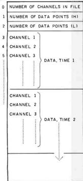
Figure 6: Map of the structure of the data file used by the author's programs. Three file-information bytes precede the actual data in the file.
