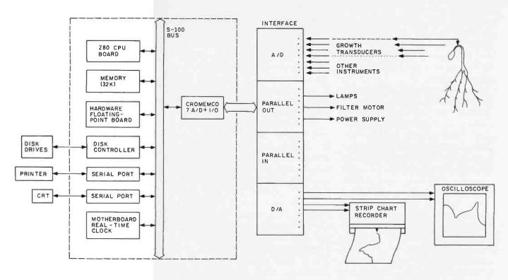
Figure 2: Block diagram of the hardware and peripherals used in the author's data-acquisition system.
