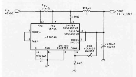
Figure 6a: A step-up regulator that converts +5 volts to +25 volts, possibly for use in an EPROM programmer. The output voltage may be adjusted within the range of +8 to +28 volts. Current capacity depends on fine points of construction and on the voltage desired.
