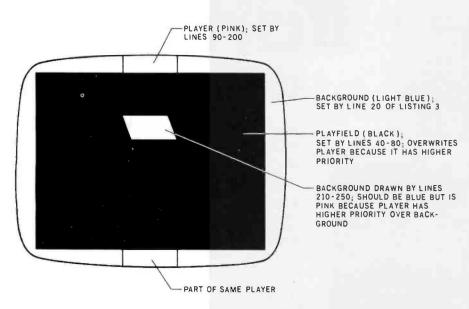
**Figure 3:** Playing tricks with the video display to achieve higher player resolution. This technique works by manipulating the relative priorities of the playfield, players, and background. See the text and listing 3 for details.
