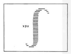
Figure 4: Use of a player as a special symbol. This can be done because players and missiles are superimposed over whatever text or graphics are in effect.
