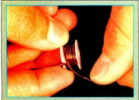
**Photo 4:** Having been wound, the wire bobbin is placed between the two halves of the pot core, which are screwed together to form the finished coil.
