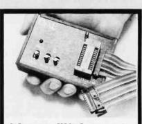
OAE's PP-Series EPROM Programmers plug directly into any vacant EPROM socket and allow you to transfer data directly from RAM to EPROMs. No additional power supplies are required. All timing & control sequences are handled by the programmer. Each unit includes internal DC to DC switching regulator, ZIF socket and 4 ft. ribbon cable terminated with a 24 pln plug. Programmers are available for all EPROMs from 2708's thru 2532's.
