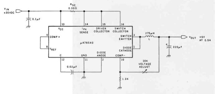
Figure 4: Schematic diagram of a 5-volt, ½-amp step-down switching voltage regulator. For low currents, the 78540's internal switching transistor and diode may be used.
