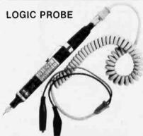
Compatible with all logic families using a 4 to 15V power supply. Thresholds automatically programmed. Visual indication of logic levels to show high, low, bad level or open circuit logic puises.
