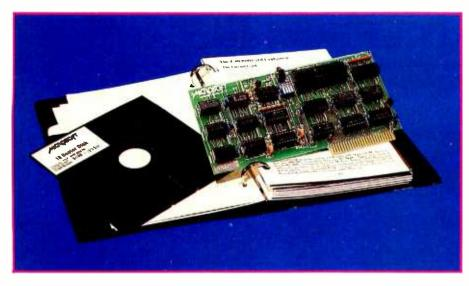
**Photo 1:** Microsoft's Softcard package. Included are the card itself, software for the Apple II, and a two-volume set of manuals (with installation instructions, information on using CP/M, hardware details, Microsoft BASIC reference, and documentation on other utilities.
