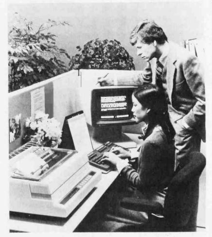
There are two HP 125 modules from which to choose: the Model 10 and the Model 20. The Model 10 uses dual 5-inch floppy-disk drives with 500 K bytes of storage. The Model 20 offers 2.4 megabytes of memory on 8-inch disks. Both models can be expanded with additional drives.
