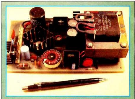
Photo 2: A commercially sold switching power supply that combines both linear-regulator and switching-regulator technology to provide outputs of  $\pm 12$  volts and  $\pm 5$  volts. Note the use of the toroidal inductor and the relatively small heat sinks. This unit was made by Conver Corporation, 10631 Bandley Dr, Cupertino CA 95014, (408) 255-0151.
