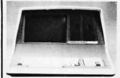
64K Double or Quad Densily units available. Uses two Z-80 CPU's. Commercial-type terminal with 12" monitor. Dual double density minifloppies. Over 350 kilobytes of storage (twice that with quad density drives). Two serial RS232 ports, I/O ports standard. Expandable with optional S-100 Interface. Comes with CP/MTM 2.2 operating system. MiniMicroMart can supply a wide range of CP/M development and application software.
