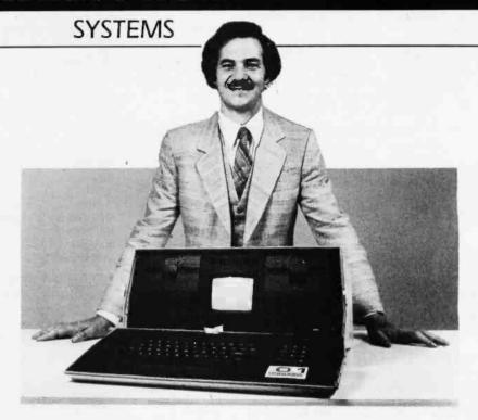
battery pack providing three to five hours of operation, modem electronics, and an acoustic coupler.
