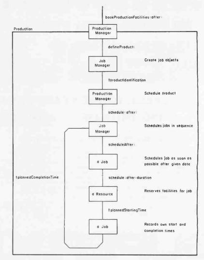
Figure 4: A simple planning algorithm implemented in a Smalltalk system.
