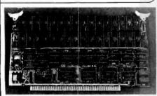
The **32K x 8 bit/16K x 16 bit** STATIC RAM BOARD uses low power and its fast device access time of 200 nsec (max.) allows for operation @ 4 MHz without any wait cycles.
