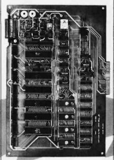
JBE's 7 ¾" x 11 ¾" 6502 base Microcomputer has the capacity for 16K of EPROM, 4K of RAM, 8 Parallel Ports and 1 Serial Port. Monitor and Tiny Basic are also available. The fully populated version includes:
