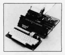
ASCII characters, graphics character font, and uses a separate microprocessor. The display module uses a vacuum fluorescent 40-character display. Assembler and other language packages are available.
