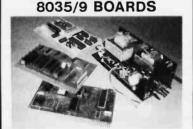
CPU 1K RAM, 40 I/O lines Parallel I/O 2 8255s, 70 mil line drivers Serial I/O 3 8251s, RS 232C interface A/D-D/A 8/1 channel All boards 4x7, 86 pin edge connector Assembled - \$125 Bare - \$20 Hardware & Software Tools available
