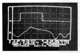
The APPLESCOPE system combines two high speed analog to digital converters and a digital control board with the high resolution graphics capabilities of the Apple II computer to create a digital storage oscilloscope. Signal trace parameters are entered through the keyboard to operational software provided in PROM on the DI control board.
