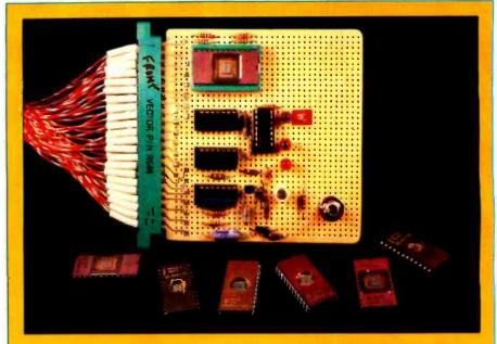
Photo 3: Type-2716 EPROM programmer, adapted from "Program Your Next EROM in BASIC" (March 1978 BYTE, page 84). The circuit, which is driven through parallel ports, programs a 2716 in about 2½ minutes and is controlled by a BASIC program.
