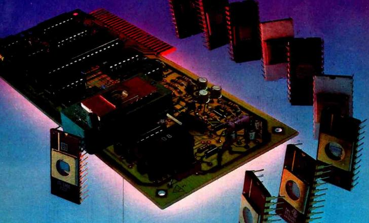
Apparat announces the most versatile EPROM burner available today for your TRS-80 model I and III or Apple computer . . . the Apparat PROM Blasting system (A.P.B.). Most EPROM burners will program only one type of EPROM. The A.P.B. system will program all commonly used 24 pin EPROMs by using special personality modules that adapt the unit to the EPROM. The following EPROMs are programmable: 2704, 2708, 2716, (3-volt) & (5-volt), 2732, 2508, 2516 and 2532.
