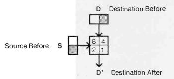
Figure 5: A BitBlt combination diagram. This diagram, when filled in, specifies the effects of a given combination (or "rule") on all combinations of dark and light source and destination cells. Each combination is given a number equal to the sum of the cells that are darkened. See figure 6 for examples.
