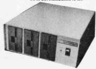
S-100 MAINFRAME WITH 12 SLOT MOTHERBOARD AND CUTOUTS FOR 3 51/4" FLOPPY DISK DRIVES
