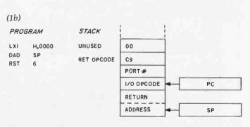
Figure 1: Stages in the assembly and execution of an indirect I/O subroutine. The C register is assumed to contain the I/O port address. Figure 1a shows how the code is assembled in the registers and pushed onto the stack. In figure 1b, the start address for the code on the stack is loaded into the HL register pair and an indirect subroutine call is performed.
