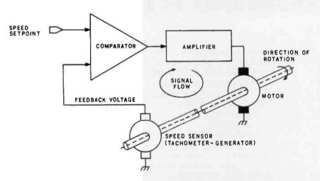
**Figure 10b:** Block diagram of a closed-loop controller. The speed sensor detects too-fast or too-slow motion and keeps the motor running without variation in speed over wide variations in load.
