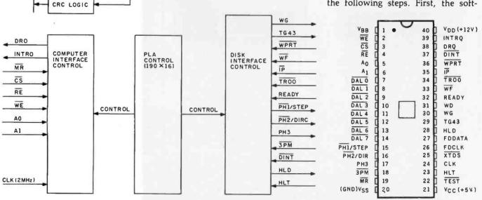
**Figure 3:** Internal architecture and pinout diagram of the Western Digital FD1771 floppy-disk controller. The four programmable registers and eleven commands of the 1771 allow any microprocessor to control a disk subsystem using high-level instructions, thus removing a significant burden from the disk-driving software. See table 1 for a summary of the commands.
