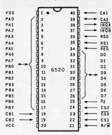
Figure 5: Pin description of the MOS Technology 6520 PIA. Use of this particular device allows easy interfacing of a disk controller to a 6502-based computer. One I/O port handles control signals; the other is used to transfer parallel bytes of data.
