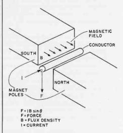
Figure 1: Simplified diagram of the basic electromagnetic principles behind the DC motor. When a current-carrying conductor is placed in a magnetic field, the conductor feels a mechanical force, F, in the indicated direction, perpendicular to the current and the magnetic field. The force is greatest when the current is flowing perpendicular to the lines of flux  $(\theta=90^{\circ})$ , as shown here. The force is zero if current flows parallel to the lines of flux  $(\theta=0^{\circ})$ .
