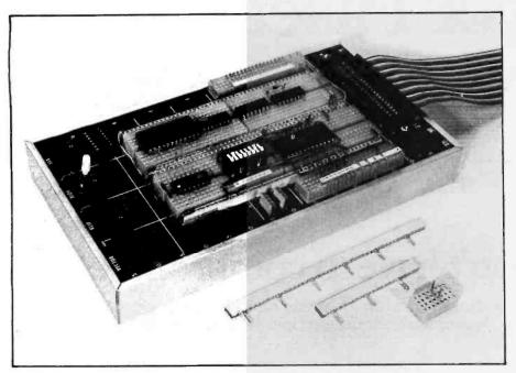
**Photo 3:** A DIP (dual in-line package) patchboard or breadboard, such as the Vector 51X patchboard, is indispensable to circuit development. This patchboard is top and bottom wirable and can be easily linked to a computer with an IDC ribbon cable.
