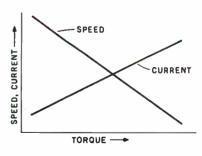
**Figure 3:** Different types of DC motors are distinguished by the type of stator field. Three types use an electromagnet to produce the stator field; the fourth uses a permanent magnet. Different methods of connecting windings in the stator electromagnet produce different speed/torque and current/torque function curves.
