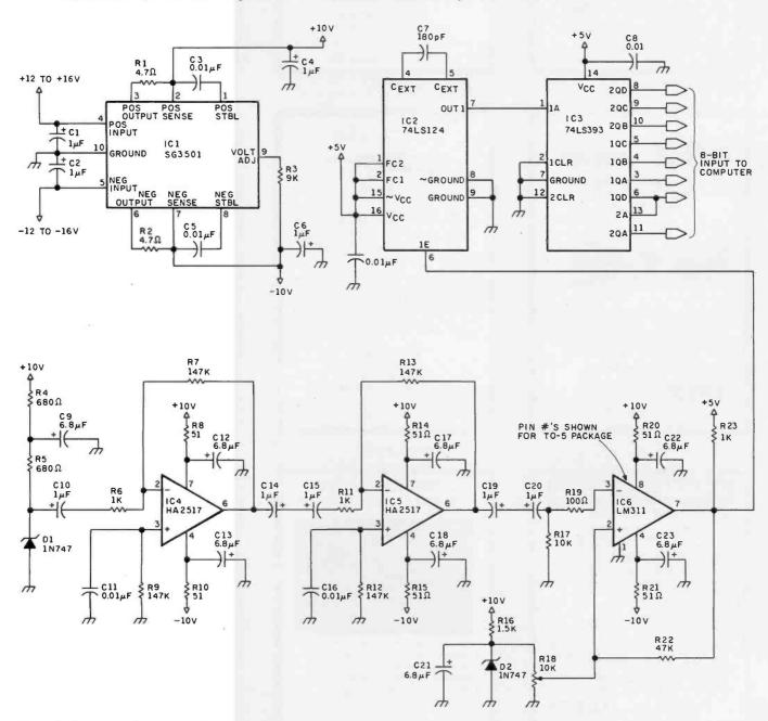
**Figure 2:** Schematic diagram of the random number generator described in this article. The noise of D1 is amplified by IC4 and IC5. The amplified noise from IC5 is compared with the DC wiper voltage of R18 at the comparator input of IC6. The level generated at the comparator input gates IC2 (running at about 3 MHz). The oscillator is clocked by IC3 (a cascaded 4-bit binary counter). The circuit should be shielded. Pin numbers shown for IC1 (Silicon General 3501) are those for a TO-5 package.
