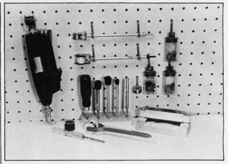
**Photo 1:** Available wire-wrapping tools include the Vector P180 Slit-N-Wrap, installed in a P160-4R cordless driver unit (left), the P160-2A-1 Dual-Way Wrap-N-Strap (top center), and the P184-Tefzel Slit-N-Wrap (below). The stand (center) displays five different pin-insertion tools. In the foreground (left to right) are the P160-1A Dual-Way unwrapping tool, P178-1 wiring pencil, and the P187 IDC fixture for assembling IDC ribbon cables.
