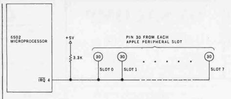
Figure 3: The  $6502\ \overline{IRQ}$  signal and the Apple II peripheral slots. The  $\overline{IRQ}$  signal is connected to pin 30 of each of the slots and is held high by the pull-up resistor shown. A maskable interrupt is generated if the peripheral card in any of the slots presents a low impedance to ground to its pin 30.
