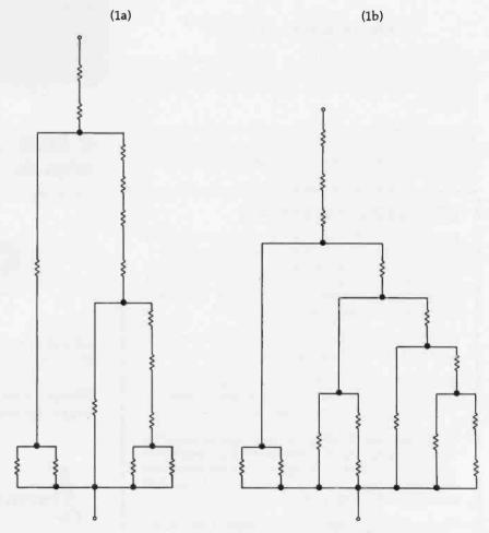
Figure 1: Two 15-unit networks with  $Z = \frac{35}{11}$
