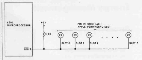
Figure 1: The  $6502 \ \overline{NMI}$  signal and the Apple II peripheral slots. The  $\overline{NMI}$  signal is connected to pin 29 of each of the slots and is held high by the pull-up resistor shown. An interrupt is generated if the peripheral card in any of the slots presents a low impedance to ground to its pin 29.
