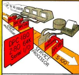
The ACE DISCOVERY MULTIPROCESSOR dedicates a complete 64K Z-80 Distributed Processing single board Computer, the dpc-180" to each user. An expanded DPC coordinates all of the system activities.
