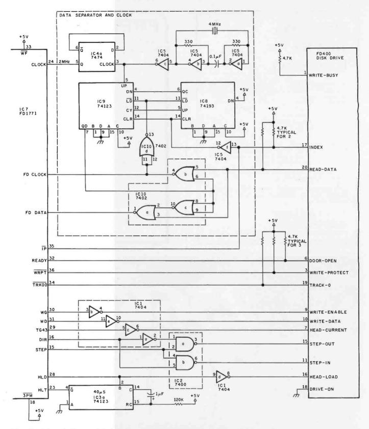
**Figure 4b:** Schematic diagram of the drive-interface side of the floppy-disk controller. Clock signals and minor control functions are provided for by the additional circuitry, as well as the separation of recorded data from recorded synchronization pulses.
