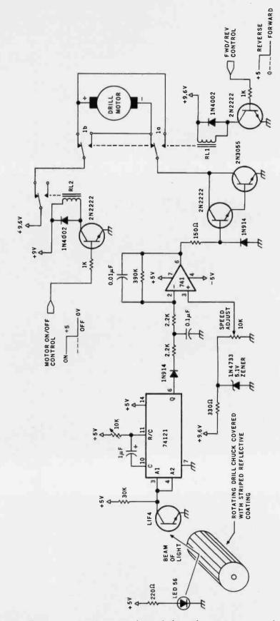
Figure 14: The motor-control system of the platform, featuring incremental-motion control and reversing capability. Two such circuits were used, one for each motor. Values of the components were experimentally chosen for use with the motor from a Black & Decker Model 9001 portable drill. The 2N3055 transistor must be mounted on a heat sink. The L1F4 phototransistor is made by General Electric.
