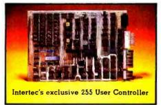
The secret behind our CompuStar DSS is its unique controller/multiplexor. It allows many terminals to "share" the resources of a single disk. So, not only can you use the DSS with your Super-Brain, you can configure multiple user stations using our new series of CompuStar<sup>TM</sup> terminals, called Video Processing Units or VPU's<sup>TM</sup>.
