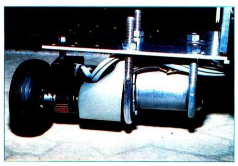
Photo 4: Close-up of a drive motor on the platform. The motor is from a 4.8 V Black & Decker battery-operated %-inch drill. The drill's case and battery pack have been removed. It is secured to the aluminum T-frame with two U bolts. A %2-inch brass rod that serves as an axle is inserted into each drill chuck. The tires are air-filled 3%-inch diameter rubber tires used on model airplanes.
