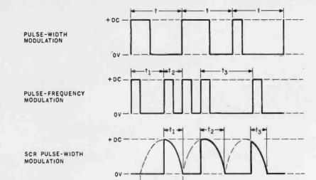
Figure 5: Comparison of three basic switching-amplifier control-circuit output waveforms. The controlling semiconductors are saturated; the average amount of electrical current transferred to the motor is limited by rapidly cutting the current off and
