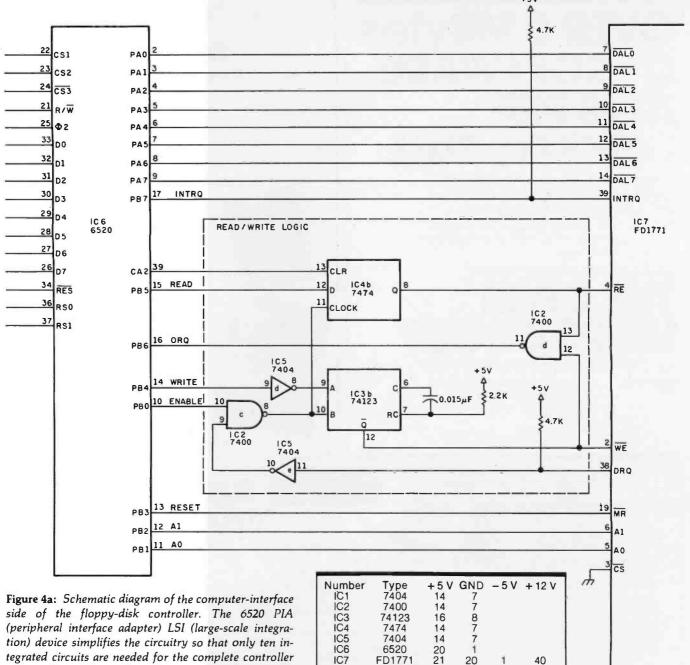
system. The additional logic devices are used to provide the read and write signals expected by the 1771. See figure 4b on page 372 for the rest of the diagram.
