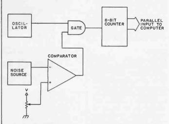
Figure 1: Block diagram of a generator that produces true random numbers. Through pulses created by the random-noise source, the free-running oscillator is gated to the 8-bit binary counter. Since the instantaneous amplitude of the voltage from the noise source is unpredictable, the width and arrival of the gate pulse generated by the comparator are also random. Therefore, the 8 bits available from the counter are truly random.
