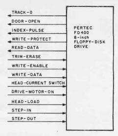
**Figure 1:** Input and output lines available for controlling a Pertec FD400 8-inch floppy-disk drive. These signals are the same as those found on any Shugart-compatible drive, so nearly any drive may be substituted for the FD400.
