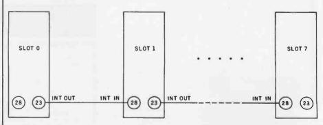
Figure 2: Using daisy chaining to create a priority system of interrupts. The INT OUT (pin 23 of each slot) and INT IN (pin 28 of each slot) signals are connected to each other to create a daisy chain that is broken by an interrupting slot. A peripheral device is not allowed to generate an interrupt unless it has highest priority or "permission" from higher-priority devices. Peripherals in lower slots have a higher interrupt priority than peripherals in higher slots. See the text for details.
