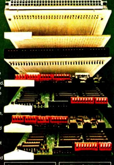
Single Board Computer Module R6502 CPU, 2K bytes static RAM, 16K bytes PROM/ROM capacity, an R6522 VIA and support circuitry on a single RM 65 modulé. module.
