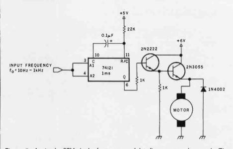
Figure 7: A simple PFM (pulse-frequency-modulated) motor-speed control. The number of constant-duration pulses supplied to the driving transistors over a given interval controls the speed.
