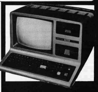
New low cost internal disk kit available to expand your storage capability. With this kit, now, you may expand your Model III computer up to four MTI 40 track disk drives, giving 175,000 bytes of storage per drive for a total of 700K.
