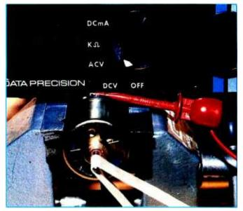
Photo 1: A PM (permanent-magnet) DC motor can also be used as a generator-type tachometer, or tachometer-generator. When the shaft is turned, a DC current proportional to the speed is produced. In the case shown, a small PM DC motor is secured in a vise, and the shaft is slowly turned (by the belt attached to the shaft and extending to the lower right). The digital voltmeter above the motor indicates the actual generator output voltage. In this case, the shaft is turning at about 150 rpm.
