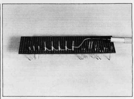
**Photo 2:** Rapid assembly of circuit boards demands insulated-wire strapping or chaining techniques, as demonstrated with the P184 Tefzel Slit-N-Wrap tool. The wide variety of board pins shown can handle any wiring situation.
