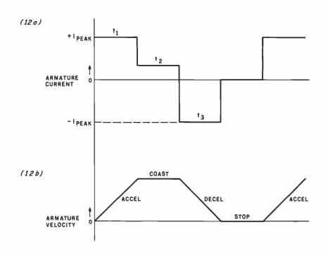
Figure 12: Precise control can be achieved using incremental-motion controllers. During predetermined periods of time, variable-amplitude voltage pulses are applied to the motor's coils. With the system initially at rest, a high positive step voltage,  $t_1$ , is applied to the motor. After motion has begun, the voltage is reduced to a lower continuing value,  $t_2$ . When the motor is to be stopped, a negative braking voltage,  $t_3$ , is applied.
