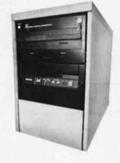
Data Storage Power with 0.5 to 96 Megabytes available. The S100 Bus and SMD disk controller access a variety of hard disk systems:
