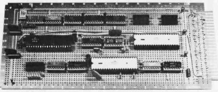
Photo 1: The authors' wire-wrapped floppy-disk controller board.
