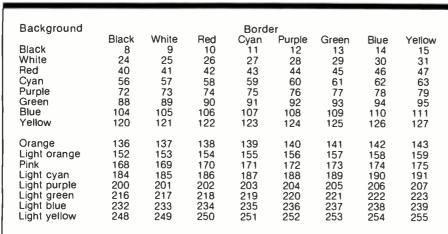
**Table 1:** Background and border color combinations in the VIC 20 microcomputer. Poking decimal location 36,879 with the values given in this table gives a video display with the colors shown.
