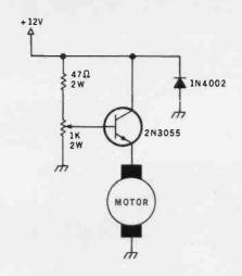
Figure 4: A simple open-loop linear motor-speed control. Operating the controlling transistor in the linear region of its characteristic curve leads to loss of energy
