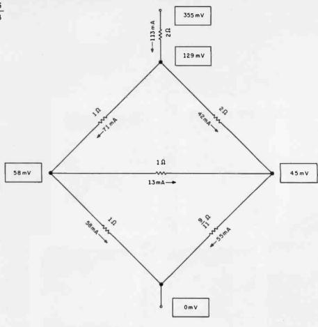
Figure 3: Voltages and currents in the 14-unit network with 355 mV across it.
