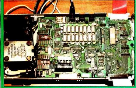
**Photo 1:** External data separator circuitry as installed in the Radio Shack TRS-80 Expansion Interface. Most of the integrated circuits can occupy the space intended for the RS-232 interface (photo 1a). Irreversible changes can be avoided by bending a few pins on the FD1771 to obtain the necessary signals (see the wires leading from the FD1771, under the red cable, in photo 1b).
