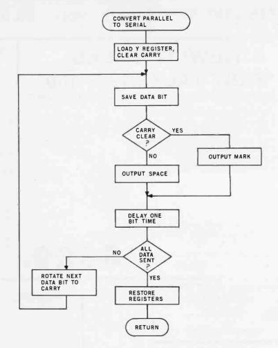
Figure 2: Flowchart for machine-language software UART in listing 1.
