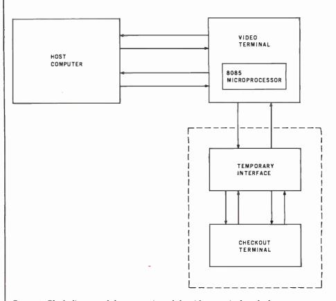
Figure 4: Block diagram of the connection of the video terminal to the host computer. Also shown are the temporary connections to the checkout terminal, used for debugging the project.
