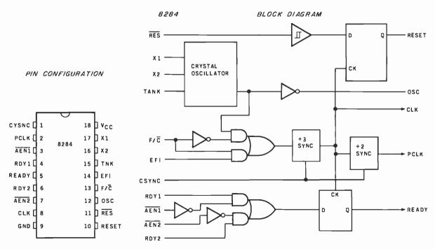
Figure 6: The 8284 clock generator. This device provides an optimum clock signal and serves to buffer and condition some of the basic processor signals. Figure 6a shows the pin labeling for the device, while figure 6b shows a block diagram of its internal structure.
