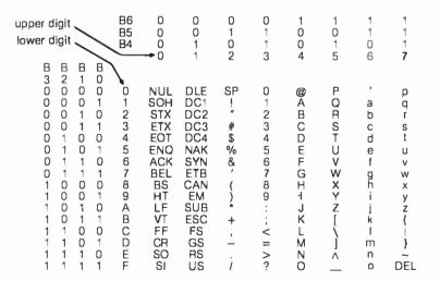
Figure 2: ASCII code table. When converting from lowercase to uppercase, by either hardware or software, only hexadecimal codes 61 thru 7A should be changed. The change to uppercase is made by setting bit B5 to 0 or, equivalently, by subtracting hexadecimal 20 from the code. All other codes should be left intact.
