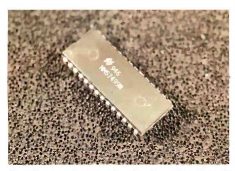
Photo 4: This twenty-eight-pin integrated circuit keeps things simple by performing the keyboard encoding and transmitting resulting data serially. It also takes care of display functions, with the addition, in figure 2a, of a single shift register.
