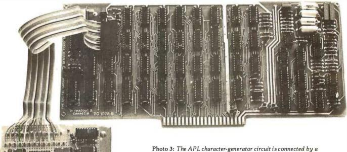
Photo 3: The APL character-generator circuit is connected by a ribbon cable to the socket formerly occupied by the MCM6571 part on the video display board. Use of sockets enables you to unplug the APL character-generator circuit and plug the MCM6571 back into the video display board if you need to reactivate the Greek characters.
