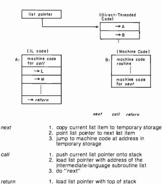
Figure 2: Diagram of direct-threaded code (DTC). Here, "temporary storage" refers to a memory location that is used to hold the address of the machine-code routine associated with the current unit of code.
