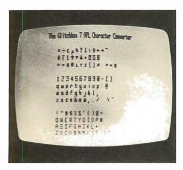
Photo 1: Video screen display of the character set produced by the APL character-generator circuit described in this article.
