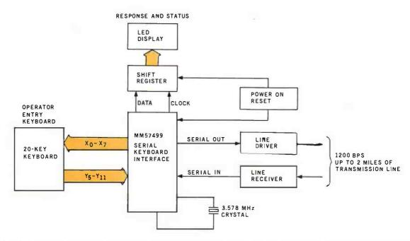
Figure 1: Block diagram of a minimal-component remote-entry panel, capable of serial communication with most host computers.
