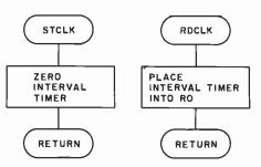
Figure 2: Flowcharts of routines to operate interval timer.
