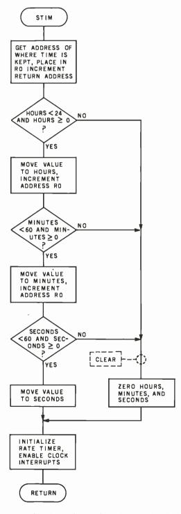
Figure 3: Flowchart of procedure that sets the clock.
