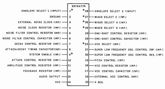
Figure 3: Pin assignments for the SN76477N complex-sound generator. It is suspected that this well-known device is marked TMC0271NL in the Speak & Spell. The pins marked with asterisks are in a logical low state unless they are pulled up by an external voltage.
