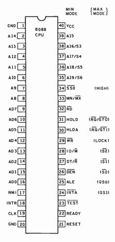
Figure 3: The pinouts assigned to the 8088 microprocessor package. Notice that many pinsserve dual functions depending on the mode selected (either minimum or maximum). Maximum mode is designed to facilitate concurrent processing, using the I/O processor and arithmetic processor also available in the 8088 family.
