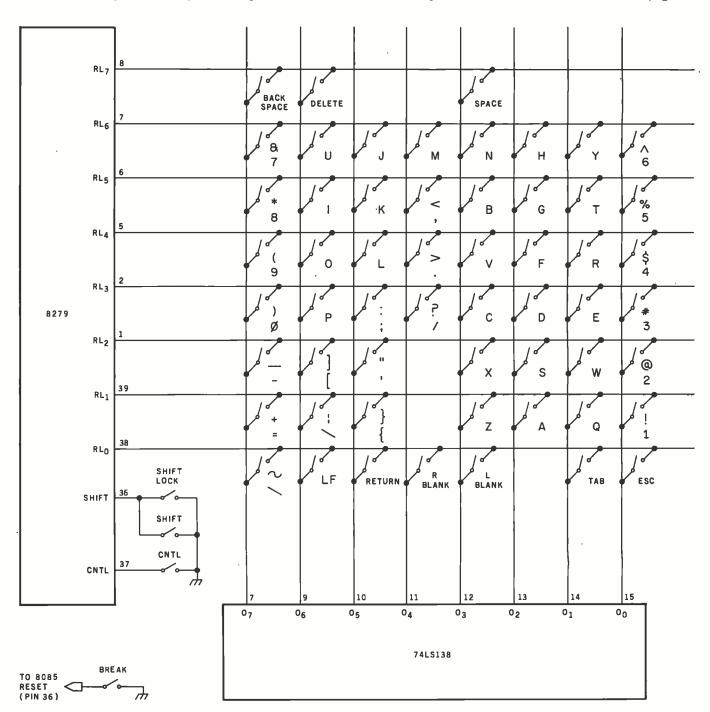
Figure 5: Schematic diagram showing detail of the keyboard matrix. A sixty-three-key unencoded keyboard from Jameco Electronics was used. The BREAK key is connected to the  $\overline{RESET\ IN}$  line of the 8085 processor.
