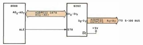
Figure 4: The ALE signal from the 8088 microprocessor is used to latch address information into an 8282 buffer. The buffer output is demultiplexed address information which has been separated from data that appears on the same pins.
