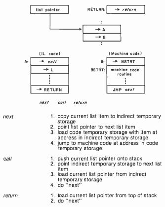
Figure 3: Diagram of indirect-threaded code (ITC). Here, "indirect temporary storage" and "code temporary storage" store the indirect and direct pointers to the machine code routine associated with the current unit of code.
