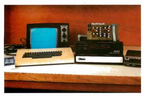
Photo 1: A wolf in sheep's clothing. The panel may say "8080," but the processor card in this system is based on Intel's high-performance 8088.
