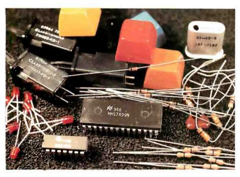
**Photo 3:** It is amazing what can be done with so few parts. Most of the components shown here are quite common and easily available. The use of such materials as a color-burst crystal and a standard hexadecimal keypad make this project reliable and nearly bullet proof.
