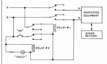
Figure 1: Steven Schafer's power-line protection circuit. The line marked H is the hot side of the power line; the line marked N is the neutral side of the power line. The resistor in series with the neon lamp should have a value of 100 k ohms.
