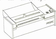
MAURO PLOTTER — Uses 11° by 8-1/2° or any length paper. Resolution is 200 steps per inch. 0.005° tracking error. Mauro X-Y vector software with pen control is available for 8080/280, 6502, & 6800 micro-processors. Requires 5 bits of a paralial output part. APPLE, TRS-80, and RS232 interfaces are available as I/O Options.
