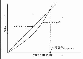
Figure 1: Area occupied by the side of a given length of tape as tape thickness is changed. The X-axis value at the nonzero intersection of area calculated by two different methods must be the actual tape thickness.
