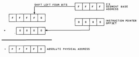
Figure 5: Calculation of the reset address on the 8088. The 8088 reset address is derived from the code-segment register, which is set to hexadecimal OFFFF, and the value in the instruction pointer, which is reset to 0.
