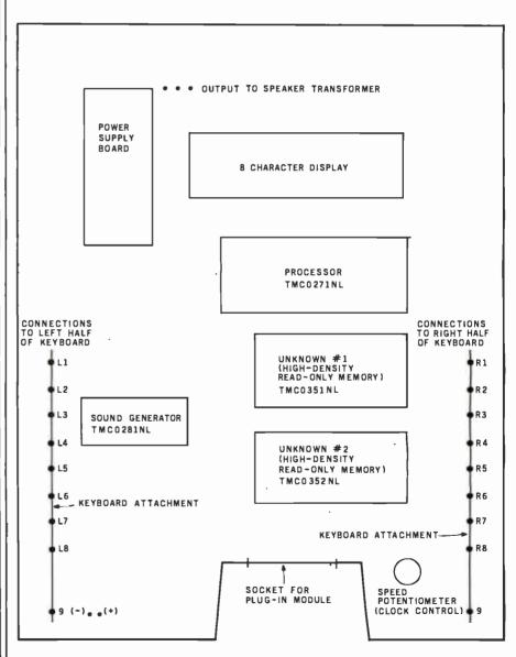
Figure 2: Layout of the Speak & Spell main circuit board, viewed from the front of the tov.
