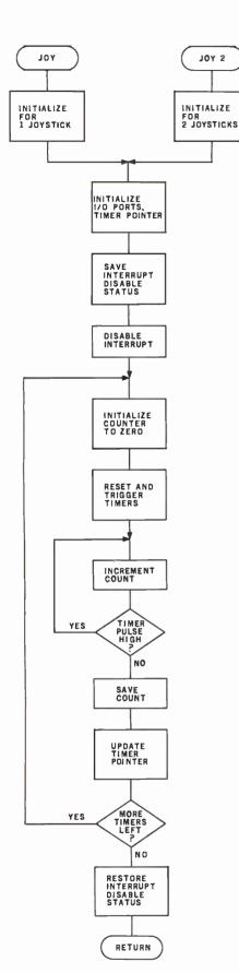
Figure 2: The joystick-driving software consists mainly of a counting loop; this determines the stick position by timing the output pulse interval. High resolution can be attained by using a fast counting loop.
