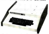
The Challenger 4P. A 4-slot computer with one open slot. Highly sophisticated 16 color video interface. 32 rows x 64 columns, upper and lower case. BK BASIC-in-ROM, BK RAM. 200-20KHz programmable tone generator. AC remote interface. Expandable to 32K RAM and two mini-floppy drives. \$750.
