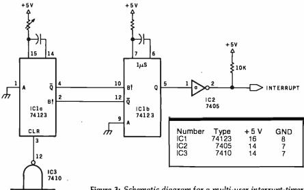
Figure 3: Schematic diagram for a multi-user interrupt-timer circuit. IC1 and IC2 are monostable multivibrators set to work in a one-shot mode. Together they generate a 1 µs negative-going pulse used to interrupt the system at a rate equal to the time allotted to each user. If control is to be passed early to the next user, the current user can write a 1 to a given memory-mapped location. This causes the SEL pin to go high and the interrupt to be generated early.
