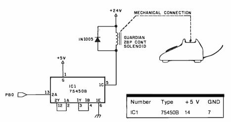
Figure 1: Schematic diagram for solenoid interface to the computer. In this method, the computer interrupts the phone line by pressing and releasing the cradle switch button on the body of the telephone set. IC1 is a TTL-compatible peripheral driver capable of switching up to 300 mA at 30 V. A logical 0 at the output bit PB0 leaves the push-type solenoid unenergized, and a logical 1 energizes the solenoid, pushing the cradle switch button down and interrupting the telephone line.
