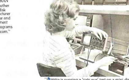
"Connie is running a 'cats eye' test on a mini-disk drive to check radial track alignment. Drive motorspeed timing and sensor alignment tests have already been performed. Disk formatting and format
