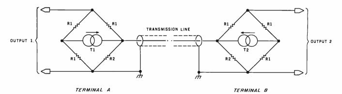
**Figure 1:** The fundamental transmission scheme. T1 and T2 are current sources (ie: transmitters) which may be either on or off. Proper termination of the transmission line is accomplished by the selection of bridge impedances to fit the equation:
