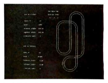
Photo 2: Display on Digital Equipment Corporation VT11 vector graphics unit showing the layout of the racetrack and the position of the one car that is racing. The display resolution is 1024 pixels by 1024 pixels.
