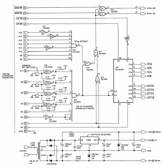
Figure 3c: Section of COMM-80 interface circuit, including power supply and address-selection circuitry. Power to the interface should not be cut off while the TRS-80 is in operation, lest programs be lost. Both units should be powered up and down simultaneously.
