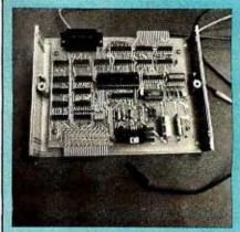
The COMM-80 is available assembled and tested in an attractive 20.95 by 15.24 by 6.35 cm (8.25 by 6 by 2.5 inch) enclosure, including expansion-bus connector and cable, an auxiliary 40-pin expansion-port edge connector, a 34-pin Centronics parallel printer port, RS-232C serial port with DB-25S connector, user's manual, power supply, and terminal software.
