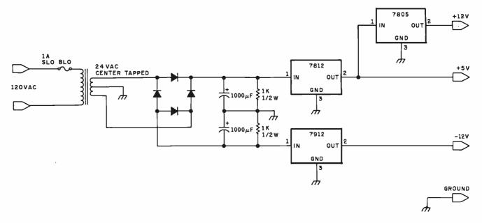
Figure 2: Schematic diagram of the optional power supply. This regulated power supply can be eliminated if the required voltages are available from a nearby computer or terminal.
