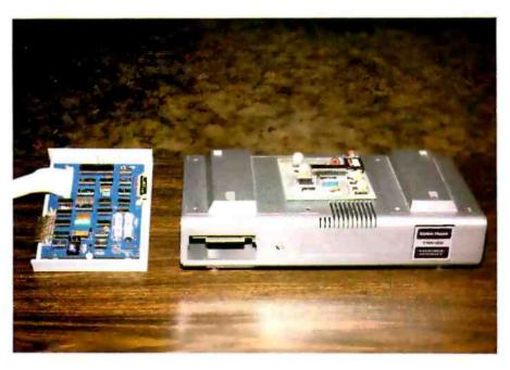
**Photo 2:** Here are two ways of adding RS-232 communication capability to the Radio Shack TRS-80. The COMM-80 unit is shown on the left; the combination of the Radio Shack expansion interface and serial-interface board is shown on the right.
