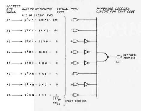
**Figure 3a:** Various methods can be employed to decode the address signals that appear on the address bus during I/O operations. Here, various inverters and an eight-input NAND gate are hardwired in a configuration that will produce a logic 0 output for one of 256 possible I/O port addresses. The logic 0 output can be used to activate the interface for the peripheral device. Here the circuit decodes the address hexadecimal C5, or decimal 197.
