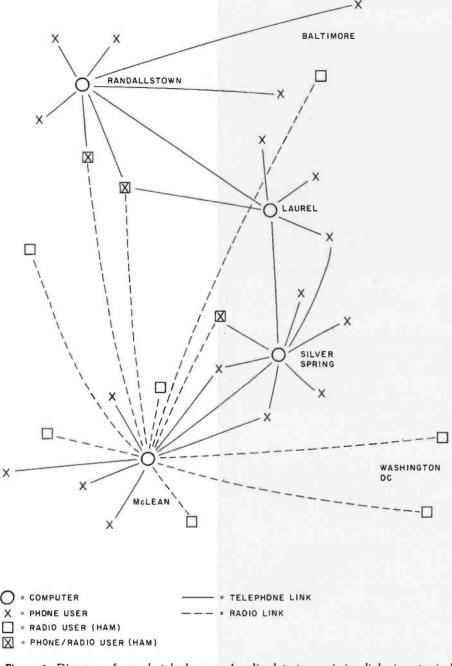
Figure 1: Diagram of sample telephone and radio-data transmission links in a typical club computer network. Several computers form nodes in the network. Solid lines indicate telephone links; dotted lines indicate links through a 2-meter band amateur radio repeater system (at the same location as one of the computers). Communities identified are located in northern Virginia and in Maryland (except for Washington DC).
