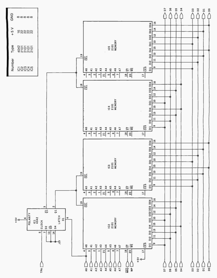
Figure 1: Schematic diagram of a two-page programmable-memory system that can easily be added to a COSMAC ELF microcomputer. Pins 17 and 22 of the memory parts should not be connected together. Instead of 2101 memory devices, it is possible to substitute CMOS 5101, 74C920, or CDP1822CD parts. Use of complementary metal-oxide semiconductor memories enables the use of batteries to retain data in memory even when the main power supply is shut off.
