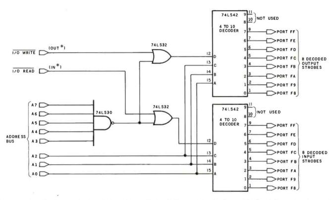
Figure 4c: Schematic diagram of a circuit that produces eight decoded input-strobe signals and eight decoded output-strobe signals. The port addresses produced are hexadecimal F8 thru FF.
