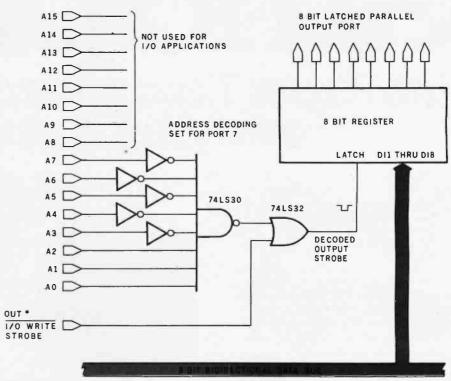
**Figure 4a:** Block diagram of a typical parallel output port. The logic that decodes the 8-bit port address was shown in three forms in figure 3. The signal from the address-decoding circuit is logically combined with one of the control signals from figure 2 (I/O WRITE) to produce an output strobe signal that activates the 8-bit output latch register.
