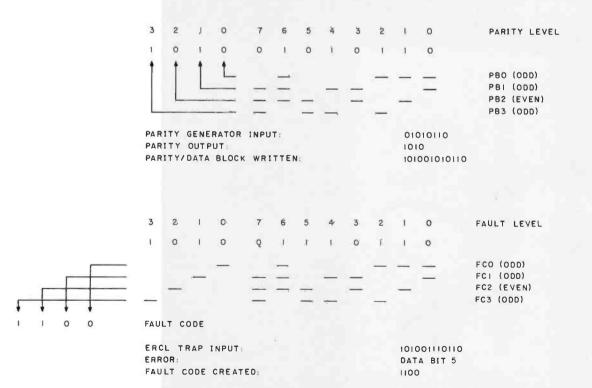
**Figure 5:** Encoding and decoding for data consisting of an 8-bit byte. Four bits are used for error checking; the possible fault codes are given in table 6.
