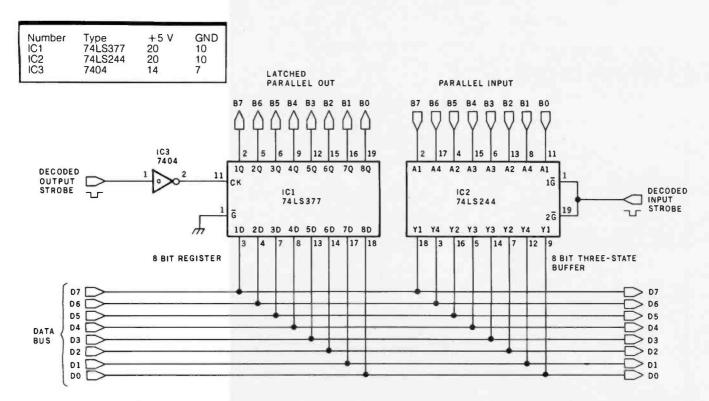
Figure 6: Data connections in input and output ports. Once the proper port address has been decoded and combined with the read-or write-control signal to form an I/O strobe signal, the actual process of accessing the data bus for data transfer is relatively easy. For input to the accumulator (the most common pathway for I/O), a three-state buffer is used in conjunction with the decoded input-strobe signal that controls the enable line of the buffer.
