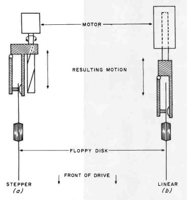
Figure 2: Two methods of moving the read/write head from track to track across the disk. A stepper motor is shown as (a); a linear or "voice-coil" motor is shown as (b). The rotary motion of the stepper motor must be converted into linear motion by a gear arrangement.
