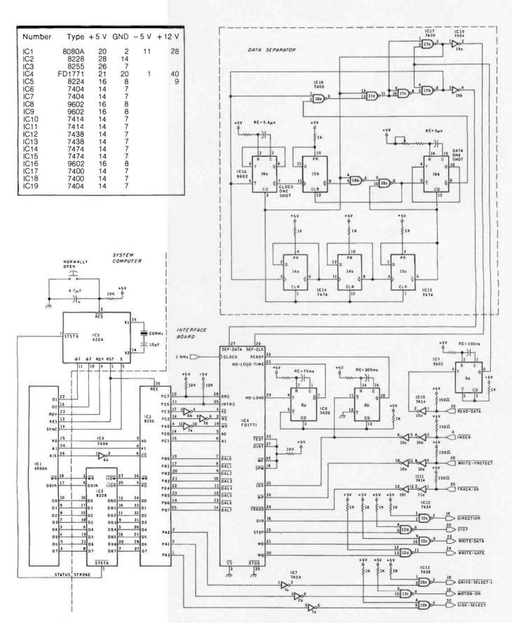
Figure 2: Disk-controller board. The circuit to the left of the dotted line is part of the computer being interfaced; the part to the right is the interface to the floppy-disk drive. The area in the dotted box is a data separator made from 7400-series TTL devices. It separates the clock bits from the data bits as they come from the disk drive.
