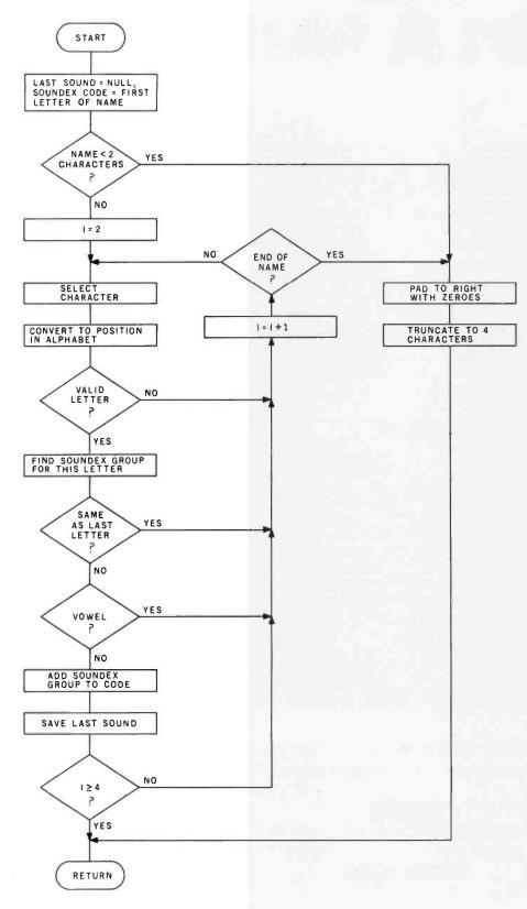
Figure 1: Flowchart of the Soundex algorithm subroutine.
