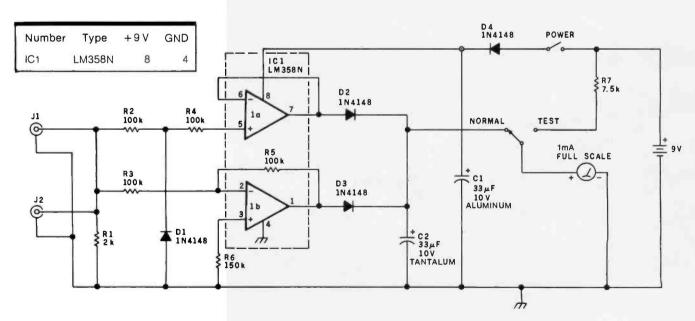
Figure 1: Schematic diagram of peak-signal-strength meter. This meter enables the user to present the cassette interface with a signal of known peak intensity—usually, about 2 V. The circuit is designed to be sensitive to voltage changes around the 2 V area.
