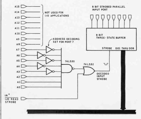
Figure 4b: Block diagram of a typical parallel input port. Note the resemblance to the output port of figure 4a.
