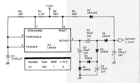
Figure 1: Schematic for the DC-to-DC converter. The 555 timer produces a rectangular wave at about 20 kHz, which is inverted by the diode-capacitor voltage-doubler arrangement. A feedback signal reaching the reset pin of the 555 regulates the magnitude of the output, which is  $-12\ V$  at  $25\ mA$ .
