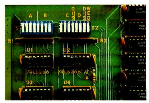
Photo 2: A more expensive and more easily changed addressing scheme employs dualin-line-pin (DIP) switches and exclusive-NOR gates. The schematic diagram for this is shown in figure 3b.
