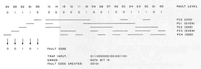
Figure 6b: Decoding and checking the 16-bit data, 5-bit parity-check word from figure 6a. Bit 14 has been transmitted erroneously; therefore a fault code of 00101 (reading from check bit 04 to bit 00) is generated. A complete list of possible fault codes is given in table 8 (in reverse order, reading from check bit 00 to bit 04).
