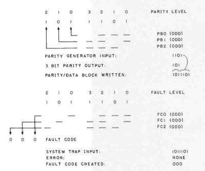
Figure 3: Sixteen different logical states may be represented in a 7-bit code with a Hamming distance of 3. Single-bit errors may be detected and corrected. Encoding in 7 bits is accomplished by performing three distinct parity checks on 4 data bits. Table 4 shows the possible fault codes. The fault code of 000 indicates that no error was detected in decoding.
