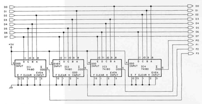
**Figure 7a:** Schematic diagram of electronic logic that encodes 8-bit data. Unused input pins on the 74180 parity-generator and tester devices are connected to ground.
