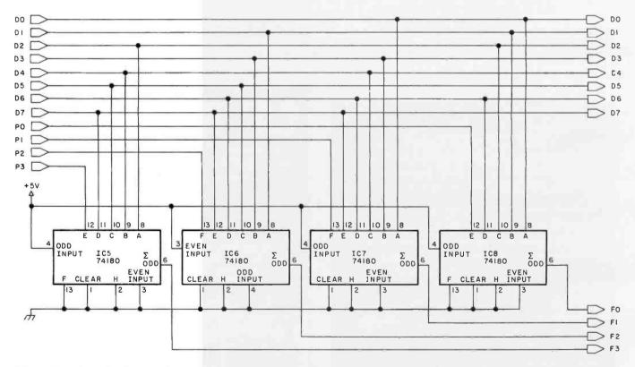
**Figure 7b:** Schematic diagram of circuit for trapping errors in the 8-bit data encoded by the circuit in figure 7a. The 12-bit word received from the peripheral device is separated into 8 bits of meaningful data and 4 bits of parity-checking data. Unused inputs on the 74180s are grounded.
