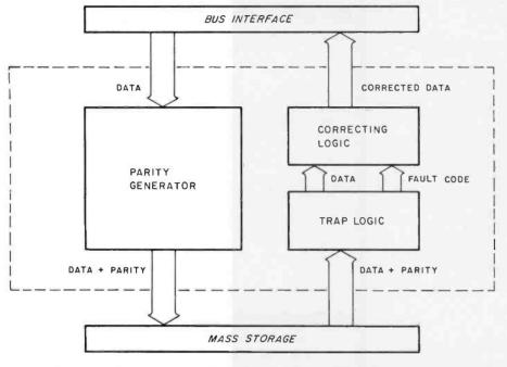
**Figure 9:** Block diagram of data flow through the error-checking and correcting system. The extra parity bits are never seen by the processor, and make the system transparent from the point of view of the system bus.
