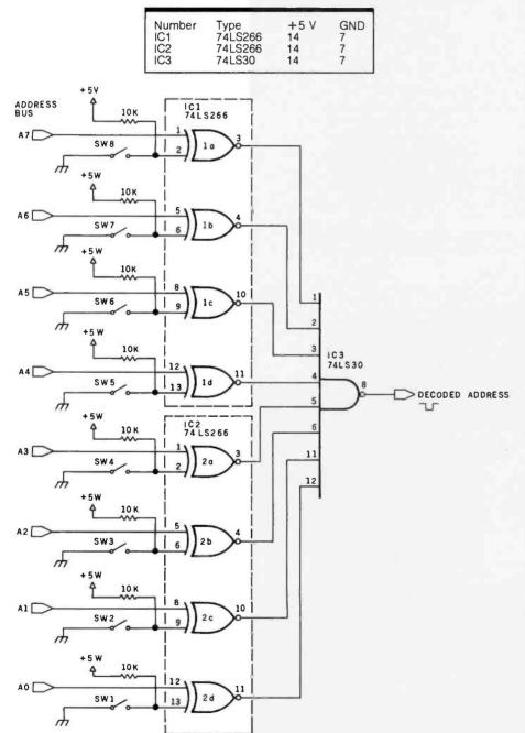
Figure 3c: Another method of decoding an 8-bit address, using exclusive-NOR gates and an eight-input NAND gate. As in figure 3b, the desired port address is set up on switches SW8 thru SW1.
