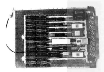
**Photo 3:** Component side of the processor board. The video signal is brought off the board by the miniature 75-ohm coaxial cable.
