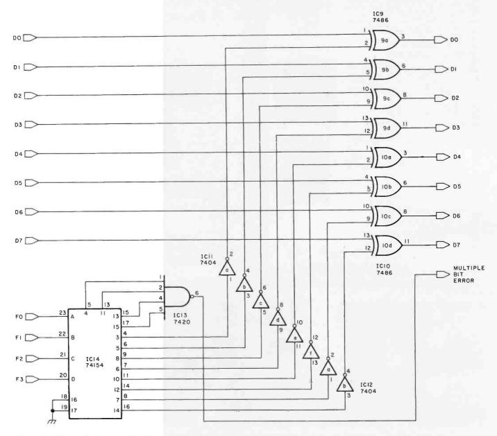
**Figure 7c:** Schematic diagram of the circuit which corrects single-bit errors trapped by the circuit of figure 7b. Multiple-bit errors are made known to the processor, but cannot be corrected using this scheme.
