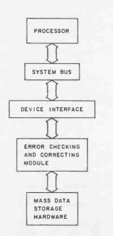
Figure 1: Block diagram showing interconnection of error-checking and correcting system with the computer.
