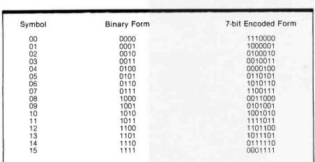
**Table 2:** Sixteen different logical entities or symbols can normally be represented by a 4-bit code. Use of a unique 7-bit encoding increases the Hamming distance to 3 and allows a single-bit error correction.
