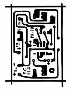
**Figure 2:** Full-sized, printed-circuit-board pattern for the peak-signal-strength meter circuit of figure 1.
