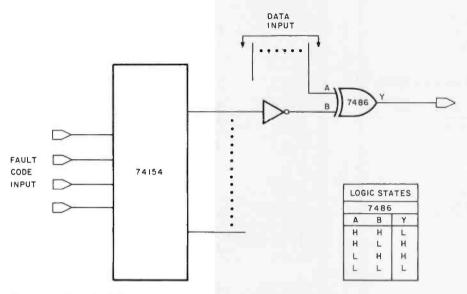
Figure 10: Detail of the error-correcting logic. Error correction is achieved by loading a binary pointer into a 4-to-16 line demultiplexer that flags the proper bit line and corrects the fault with an exclusive-OR inversion. Eight-bit systems may load the fault code directly into the demultiplexer and avoid the use of a read-only memory.
