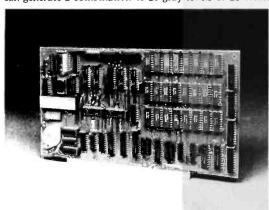
character field is 9 by 16 (or 144) pixels with a raster scan of 621 pixels. The entire character field can be changed at one time for fast animation. Adjoining character fields of any shape can be combined to create large continuous characters. The VG100 is configured in 12 K bytes of programmable memory and is selectable in three 4 K-byte blocks. The price is \$645. For details, contact IPDI, 1708 Stierlin Rd, Mountain View CA 94043
