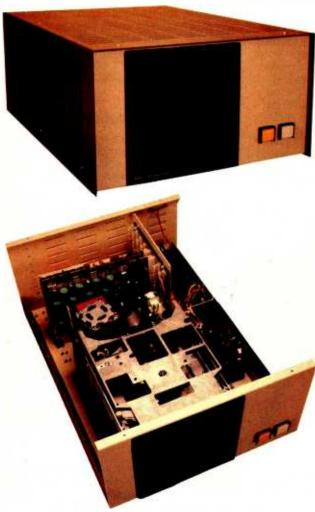
The C2-OEM with cover off showing the placement of floppy drives, UL recognized power supplies and 8-slot OSI 48 BUS backplane.
