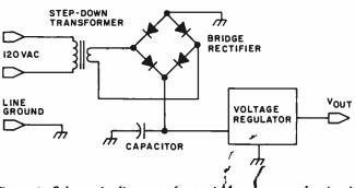
Figure 1: Schematic diagram of a typical power supply circuit containing a step-down transformer, a full-wave bridge rectifier, a filter capacitor, and an integrated circuit voltage regulator.
