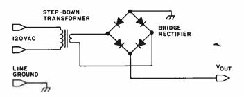
Figure 2: Schematic diagram of the power supply without capacitor or regulator. This circuit produces the output voltage waveform shown in figure 3.
