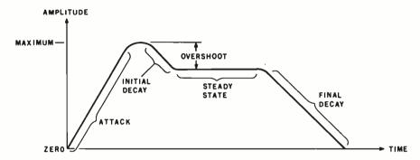
Figure 6: Amplitude envelope for a typical musical sound. This exhibits in graphic form how fast a given tone builds up, continues to sound, and then dies away. Terms for various parts of the envelope are shown.
