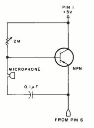
Figure 2: A microphone and simple amplifier can be added to the Apple paddle connector and used to input audio information. The program in listing 2 is used with this circuit.
