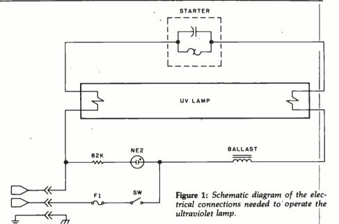
F6T5/BLB 89G435 (General Electric) 6 watt ultraviolet lamp 4,6,8 watt ballast
