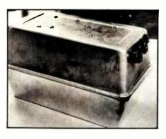
Photo 1: The case for the EPROM eraser is made of two bread-baking tins hinged together with flexible material. Power supply components are mounted in one end of the upper tin.
