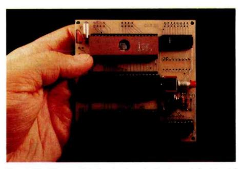
**Photo 1:** This 8088 system fits in the palm of your hand and uses only five integrated circuits. It contains enough read-only and programmable memory, and sufficient peripheral interfaces, to support two 300 bps terminals, running a Tiny BASIC interpreter on each.
