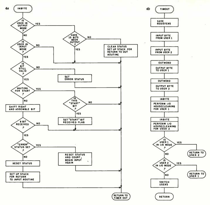
Figure 4: Flowchart of the multitasking routine of listing 1, which divides the resources of the 8088 system between the two users. (4a) Routine to receive input from one of the users. (4b) Routine to handle timing out of the time-arbitration counter.
