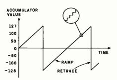
Figure 1: Generation of a sawtooth waveform by software. Coordinate points along the waveform are generated by continuously adding a constant value, FREQ, to the accumulator (register A). The point values (samples) are sent to the D/A converter. A close-up circle demonstrates the inevitable stair-step quality of the curve reproduced from discrete samples. The 6502 assembler code to produce the sawtooth is shown in listing 1.
