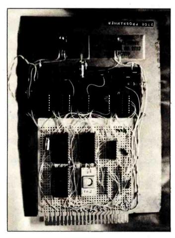
**Photo 1:** Front side of the EPROM programming circuit board. Components may be identified from diagram of figure 4. A Radio Shack 44-pin card forms the base of the board, which has had other sections added to it. TO-220 packages at top are voltage regulators.
