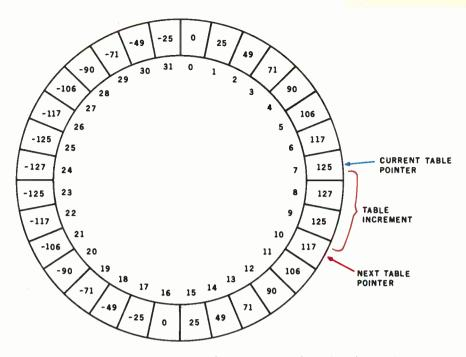
Figure 4: Conceptual diagram of a waveform-scanning table. The table, in this case containing thirty-two waveform samples, is scanned in such a manner that the end of the table seems to be contiguous with the beginning. The table pointer indicates the value that is currently being sent to the D/A converter. During each sample period, a table-increment value is added to the table-pointer value, yielding a new pointer position further around the table.
