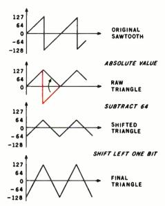
Figure 2: Method for transforming samples of a sawtooth waveform into samples of a triangular waveform. First the absolute value of the contents of the accumulator is determined. A constant value, 64, is subtracted from the accumulator. The remaining value is multiplied by 2; the multiplication is performed by the simple method of shifting the binary value one bit to the left.
