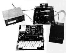
A complete disk system for the Rockwell Aim 65. Uses the Rockwell Expansion Motherboard. Base price of \$850 (U.S.) includes controller with software in Eprom, disk power supply and one packaged Shugart SA400 Drive.
