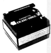
Two battery-powered machines offer longer life for cassettes and reduced wear on standard cassette players. The Erase-Sure passes the cassette through a rotating magnetic field that erases the tape and leaves an extremely low residual noise level. The user slides the cassette through the unit once. This
