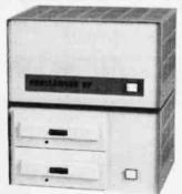
Challenger 8P. Ohio Scientific's mainframeclass. Personal computer. 8 slots with 6 open. Cassette based with 8K BASIC-in-ROM. 8K static RAM, expandable to 32K RAM, and dual B-inch floppy disk drive. \$895.
