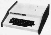
**The Challenger 4P.** A 4-slot computer with one open slot. Highly sophisticated 16 color video display. 32 rows x 64 columns, upper and lower case. BK BASIC-in-ROM BK RAM. 200-20KHz programmable tone generator. AC remote interface. Expandable to 32K RAM and two mini-floppy drives. \$698.
