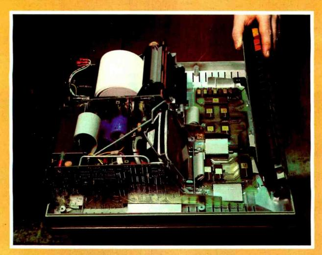
**Photo 3:** Internal view of the HP-85, showing the processor board under the hinged keyboard. The 8-bit processor is a custom Hewlett-Packard design, as are most of the integrated circuits in the computer.
