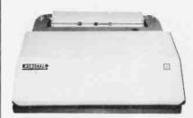
The Robotype Model 2100 is capable of interfacing with a Centronics-compatible parallel interface, RS-232C
