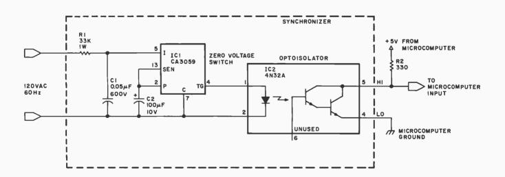
Figure 5: Synchronizer necessary to provide correct timing reference. IC1 is a zero voltage switch that produces a current pulse (from pin 4) at the beginning of each AC half cycle. This current pulse is optically coupled through IC2 to pull a current pulse through R2, thus generating a momentary logic 0 at the synchronizer's output. For convenience and electrical safety, the circuit shown inside the dotted line should be built into a protected, insulated enclosure.
