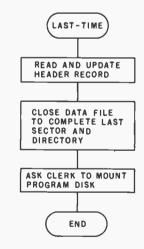
**Figure 4:** Flowchart of the routine that terminates execution of the Tickler system in an orderly manner.
