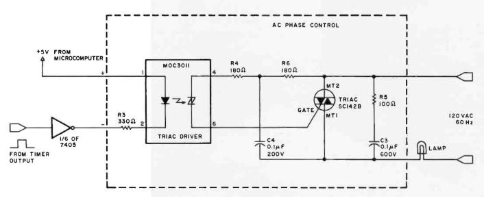
Figure 9: Circuit for connecting one timer output to the AC circuit it controls. The AC phase-control circuit contained within the dotted lines should be built into a metal box, and the triac's isolated mounting tab securely fastened to the inside wall of the box. (Substitution of a different triac without the isolated mounting feature will require the use of special mounting hardware to electrically isolate the triac from the wall of the enclosure.)
