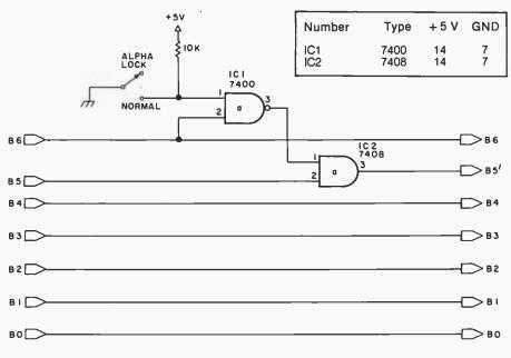
**Figure 1:** A simple circuit to provide alphabetic uppercase lock. It causes the undesired shift of 6 punctuation and control codes in addition to the alphabetic characters.
