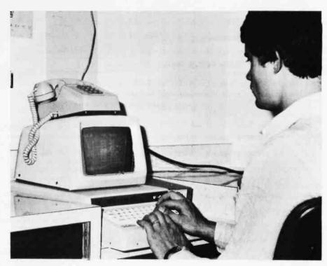
**Photo 1:** Dialing the telephone is done by selecting from a menu displayed by the computer on the screen of the video terminal.
