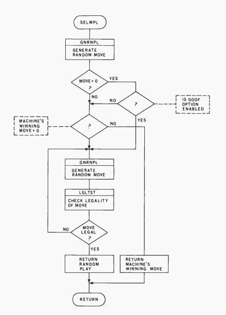
Figure 7: Flowchart of the subroutine that determines the machine's play (SELMPL). If the goof option is selected, the odds are one in eight that the computer will make a random legal play, instead of playing the apparent winning play discovered while revising the win table. If no winning play is found, a random play is made.
