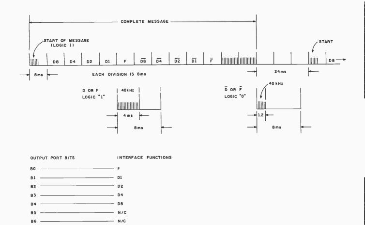
Figure 3: Description of coded message sent from the cordless controller to the command console via ultrasonic communication. The necessary codes are shown in table 1.
