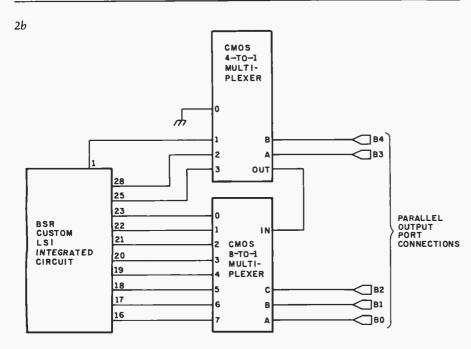
Figure 2: The keyboard in the BSR X-10 command console and remote control unit is connected to a custom LSI integrated circuit. Figure 2a shows the keyboard in relation to lines coming from the BSR custom integrated circuit. The functional schematic in figure 2b could be used to replace the keyboard with an I/O port.
