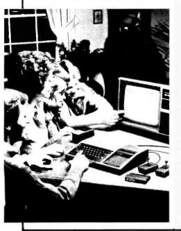
and education. Designated the Model TI-99/4, the system consists of a console with 16 K bytes of programmable memory, a wide range of sound effects, sixteen colors for graphic display, a powerful extended BASIC programming language, and a 13-inch color video monitor.
