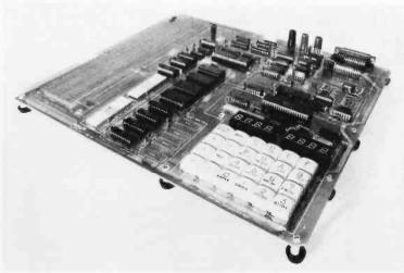
The 2 K bytes of 2142-type programmable memory can be doubled by implementing additional devices in the positions provided. There is room for 8 K bytes of program instructions using either or both of the keyboard and terminal software monitors included in the kit. There is a fully buffered system bus. Programs and data may be entered three ways: from the built-in keyboard; through a built-in serial communications interface; or via cable (SDK-C86) from
