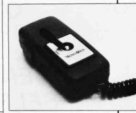
ISC Inc. 2224-C Old Middlefield Way, Mountain View CA 94043, has introduced the Model VS20/APL Videostick X/Y controller for the Apple II. The unit features a large push (firing) button and a linear joystick designed specifically for applications such as plotting graphics or playing games. The controller plugs directly into the Apple II and can be hand-held or table positioned.
