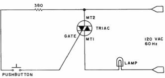
Figure 2: Basic switching arrangement for proportional AC phase control using a triac.
