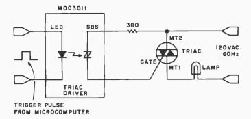
Figure 4: Electrical isolation between the computer and the triac is achieved with a device containing an LED and a silicon bilateral switch (SBS).
