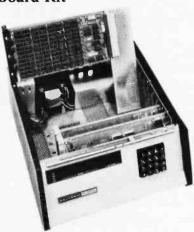
The H8 Extender Board allows Heathkit owners to troubleshoot their machine easily because each board is up above the computer for access to all circuits and components. Jumper links in power lines make power measurement simple. The links can be replaced with fine copper wire, which protects the traces or the motherboard from damage due to excessive current during testing.
