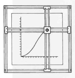
Figure 1: A sketch of the complete plotter: mechanism.
