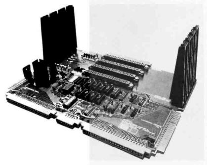
The Little Buffered Mother mother-board incorporates 4 K bytes of programmable memory on the motherboard itself, which, when used with either the SYM-1 or AIM-65, gives the user a total of 8 K bytes of contiguous programmable memory (5 K contiguous on the KIM-1). The motherboard also has regulators for the on-board logic and has the power required for all three microprocessor boards, except the +24 V for the AIM printer.
