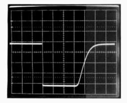
Photo 1: Output of the synchronizer. The waveform was recorded with a vertical scale factor of 1V per division and a horizontal time base of  $100\mu s$  per division. Its zero is at the bottom line of the screen.
