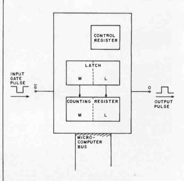
Figure 6: Model of the programmable timer, showing gate input  $\overline{G}$  , output O, the connection to the microcomputer bus, and the addressable registers. The arrows pointing from the latch to the counting register indicate the data transfer that takes place at the beginning of each count.
