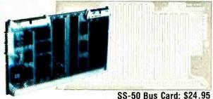
conductors · contacts for power regulators and distributed capacitance bypassing use wire wrap, wiring pencil or solder wiring • tin-lead plating over 2-oz copper conductors wets quickly, solders easily FR4-G10 epoxy-glass substrate.
