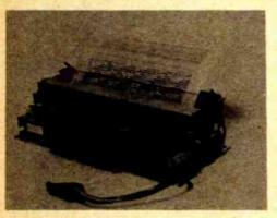
Featuring a 100,000,000 character dot head, this 80 column Model 3110 dot matrix printer mechanism is being introduced by Epson America Inc, 23844 Hawthorne Blvd, Torrance CA 90505.
