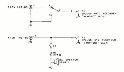
Figure 1: Cassette interface switching box for the TRS-80. The circuit enables the user to manually control the cassette recorder without having to unplug the recorder's remote jack, and allows audio monitoring of the tape while it is being loaded into the computer.
