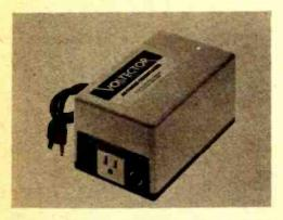
The new Voltector Series 5 AC power conditioner protects microcomputers and other sensitive electronic equipment from power line noise and high energy transients, saving the cost of a dedicated line. The Series 5 provides both common and transverse mode protection against RF (radio frequency) noise and against the destructive surges, spikes and transients that enter a building on the primary power line servicing it.
