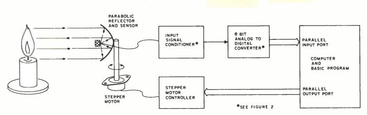
Figure 1: Block diagram of closed loop optical scanning system. The three main sections are the optics, consisting of a parabolic reflector and visible and infrared detector, the signal conditioner and input interface, and the stepper motor.
