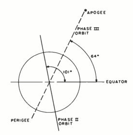
Figure 9: Typical orbit of the Phase III satellite. The greater the altitude of the spacecraft, the more ground it sees and thus the greater the communications range. The Phase II orbit at 1440 km allows communication ranges of up to 2400 km. The Phase III orbit, with a much higher altitude, will provide communications over the entire northern hemisphere and much of the southern hemisphere.
