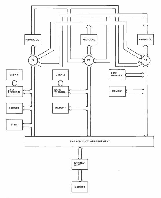
Figure 1: Loosely coupled network using protocol and shared slot modules.
