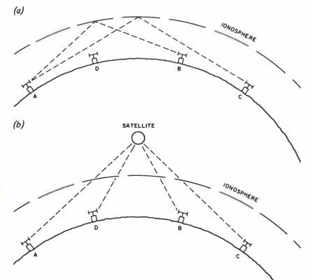
Figure 7: Propagation considerations. When two radio stations are communicating via shortwave propagation by bouncing signals off the ionosphere, it may be difficult to tell exactly which station you are communicating with since the ionosphere is a dynamic medium. Introducing a satellite as in figure 7b will alleviate this difficulty by not using the ionosphere for propagation.
