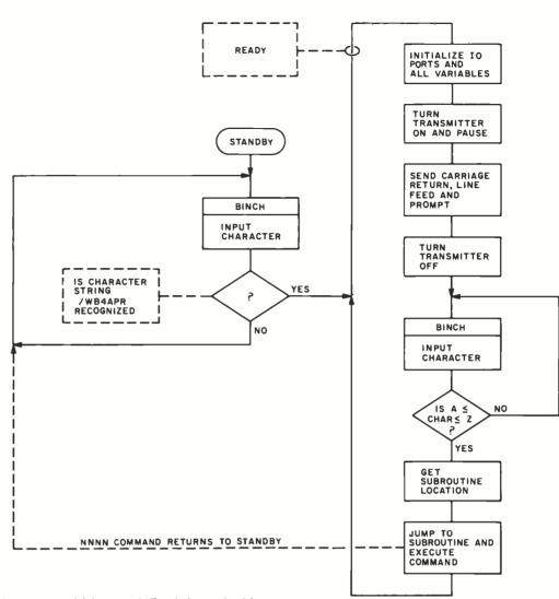
Figure 4: Flowchart of the system monitor showing the standby and ready states.
