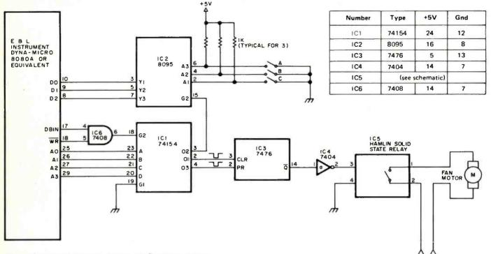
Figure 4: Control circuitry for the air flow experiment.
