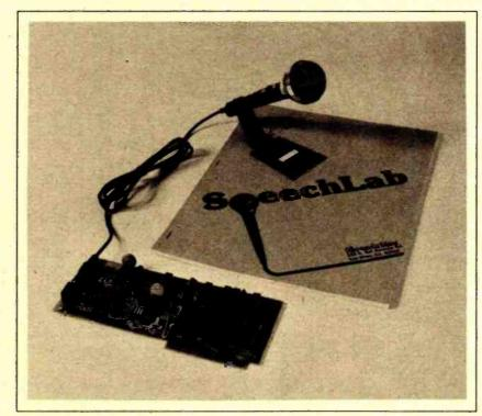
A new voice data input unit for the Apple II computer has been announced by Heuristics Inc, 900 N San Antonio Rd, Los Altos CA 94022. Known as Speechlab Model 20A, it features a 32 word vocabulary, fast real time response and the capability of multiple training samples for high accuracy.
