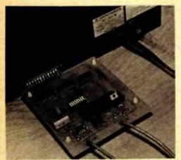
The 32 K byte Bytesaver holds up to 16 of the Intel 2716 memories or equivalent. Switches are provided to: protect and unprotect programmable read only memories individually or in groups for programming; shadow read only memory socket pairs, thus allowing external programmable memory to overlap portions of read only memory address space, select card address, and control the Bank-Select and direct memory access input and output features.
