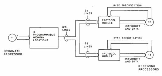
Figure 3: Protocol modules are controlled by the receiving processors within the local network.
