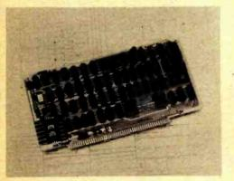
Requiring +8 VDC at 1.2 A, the Flashwriter generates a video display of 1024 characters arranged as 16 lines of 64 characters each and uses a 7 by 9 dot matrix to produce a high quality, high resolution display image. The board also has an 8 bit parallel port with latched strobe that may be used as a keyboard port.
