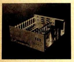
A starter set for the construction of an S-100 cardframe and power supply has been announced by Objective Design Inc, POB 20325, Tallahassee FL 32304. The kit allows the beginner
