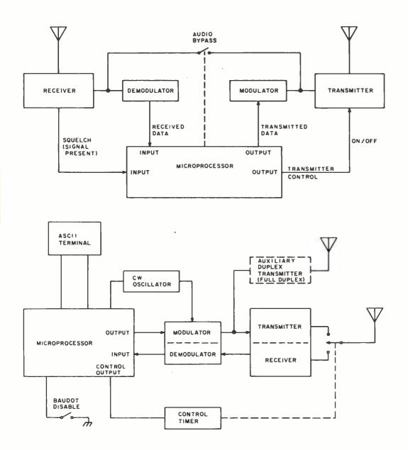
Figure 2: Having the microcomputer at the repeater site has the advantage of full duplex operation if user stations overcome the complexity of full duplex operation at their own stations.
