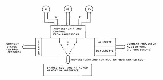
Figure 2: The existing processor bus can be extended by adding a shared slot arrangement. The actual switching mechanism is software controlled.
