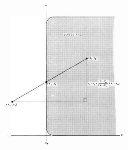
Figure 12a: Clipping. One way of calculating the cutoff point for a line is to use the traditional method of similar triangles. A disadvantage of this method is that it requires multiplication, a relatively time consuming operation on a computer.
