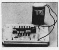
The Continental Specialties Corp carries a line of Experimenter socket solderless breadboards. The smallest of these is 3.6 inches by 2.1 inches by .3 inches, about the size of an audio cassette. No soldering, drilling or tooling is required. Parts simply plug right into the breadboard and interconnections are accomplished by pushing short lengths of hookup wire into adjacent holes. Prices range from \$4 to \$10.95. Contact Continental Specialties Corp, 70 Fulton Ter, New Haven CT 06509.
