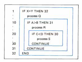
Listing 1: A BASIC-like program equivalent for the flowchart of figure 7. The lines in the picture emphasize the structured programming formalism.
