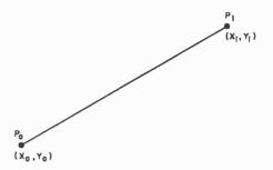
Figure 2: The straight line, a basic element in many displays. If two points are to be connected by a line segment, in a raster graphic display it is necessary to calculate every point on the connecting line. In the case of a vector display, only the endpoints of the vector need be computed.
