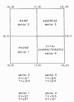
Figure 1: Physical arrangement of sectors on the screen as used by program in listing 4.
