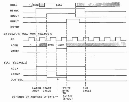
Figure 4: Timing diagram of an LSI-11 memory write (8 bit byte) cycle as it is interpreted by the S2L and passed on to the Altair (S-100) bus.
