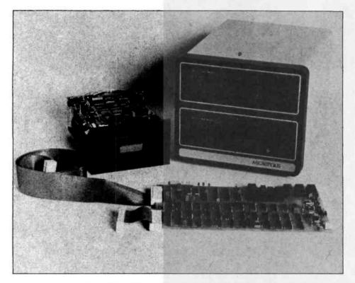
Double sided floppy disk drives are now available on two of Micropolis Corp's OEM series. The company's Mega-Floppy series, Models 1015 and 1055, features an intelligent controller that facilitates interconnection of four subsystems to a common host interface for a total on line storage capacity of more than 15 M bytes.
