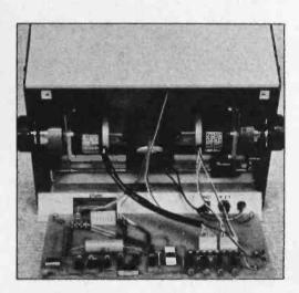
Photo 3: Inside the Hi Plot plotter, we find this pair of stepper motors which drive the mechanism through cable linkages.
