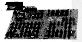
The C/D-40 interface board allows the 300 line per minute Teletype Model 40 printer to connect to a host computer or terminal that offers a Centronics or Dataproducts interface. Complete hardware and software transparency is provided so that plug to plug compatibility exists without making system modifica-
