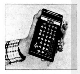
An alternative to the Teletype has been developed by Gleichmann & Co, Wormser Str 9, D 6710 Frankenthal WEST GERMANY. The pocket-sized terminal has the same electrical interface but according to the company costs about one tenth as much as the conventional solution.
