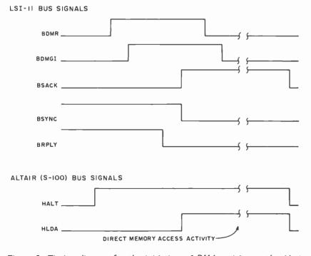
Figure 5: Timing diagram for the initiation of DMA activity on the Altair (S-100) bus between memory segments on that bus and peripherals on that bus. (DMA from an Altair (S-100) bus peripheral to peripherals or memory on the LSI-11 "Q" bus is not supported in this design.)
