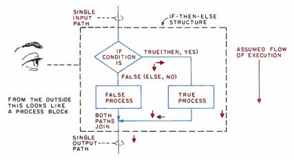
Figure 4: The if-then-else structure is composed of a decision block and two process blocks. The process blocks may themselves be viewed as any form of structure with a single input and a single output path; and thus might in fact be sequence structures, if-then-else structures, etc.
