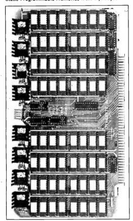
Two fully static programmable memory modules for the Altair (S-100) bus are now available from Dynabyte Inc with access times of either 450 or 250 ns. The 250 ns mode is compatible with 4 MHz Z-80 processors.
