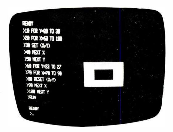
Photo 4: An illustration of the use of the TRS-80's graphics capabilities. The BASIC program shown on the screen created the square and cutout by using the SET and RESET statements to turn points on and off. This illustrates the arbitrary way in which text and graphics can be interspersed on the display.
