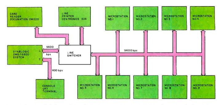
Figure 1 The system block diagram of the multiple microprocessor laboratory. This design allows each student team to have a separate dedicated computer with a shared set of peripherals controlled by the main system. The use of a common mass storage, printing and card input facility avoids the expense of having equivalent facilities at each student station. The "microstations" are small computers with limited (but still interactive) resources.
