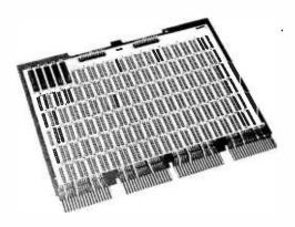
The CIP4 and CIP4/11 universal wire wrapping boards plug into the Digital Equipment Corp standard "Omnibus" and "Q-Bus" backplanes, and provide 32 columns of 60 low profile socket terminals per column with alternate rows of ground and power terminals. The boards will accommodate up to 110 16 pin sockets or an equivalent in other sizes and are priced from \$1.50 to \$2 per chip position, from Garry Manufacturing Co, 1010 Jersey Av, New Brunswick NJ 08902, (201) 545-2424.
