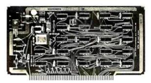
88-SPM CLOCK MODULE: The 88-SPM provides a time of day clock and an independent realtime clock on one S100 compatible module. Provisions are included for battlery backup so the 88-SPM can maintain the time during power-off conditions. \$96.00 kit
