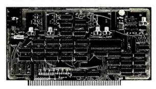
88-UFC UNIVERSAL FREQUENCY COUNTER: The 88-UFC is an \$100 compatible frequency and period measurement module. The 88-UFC has four software selected inputs. Frequency measurement to above 600MHz and period measurement to 1/10th microsecond are standard. The counter provides nine digits of readout and is priced at \$179.00 in kit form.
