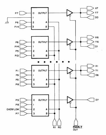
Figure 9: Output decoding. Four MSI devices, 74153 dual 4 to 1 data selectors, are used to decode outputs PS, P1, ..., P14 of the MPY-8AJ as well as the OVERFLOW signal generated (on the condition in figure 8). Two three state 74125 quad buffers decouple the low impedance totem pole 74153 outputs from data bus D0, D1, ..., D7. Since the X and Y inputs of the multiplier are high impedance, X1-X7 and Y1-Y7 are coupled directly to data bus bits D6 to D0. ENABLE OUT signal comes from figure 7.
