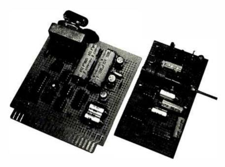
Photo 2: Prototype boards of transmitter (at left) and one receiver board. Receiver unit is described next month.
