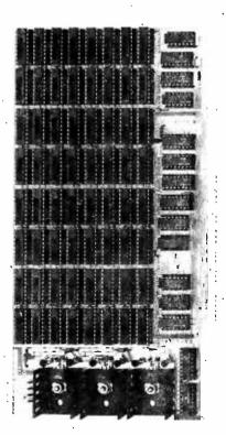
Artec Electronics Inc has introduced a 32 K byte static programmable memory board in modular form designed for the Altair (S-100) bus.
