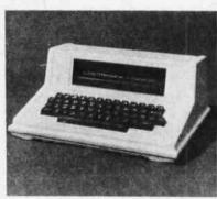
The Transactor I data terminal consists of a single line 32 character gas discharge display with a 5 by 7 dot matrix for easy reading, and a 53 key Teletype style keyboard. It can be attached to almost any computer, with an RS232 or 20 mA current loop interface. Switches allow the user to select the operating mode including 110 to 9600 bps data rate, full or half duplex, even, odd or no parity, five to eight data bits, and one or two stop bits.
