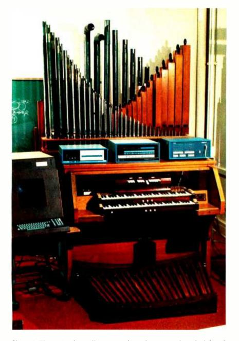
Photo 1: The authors' overall system with graphics terminal on the left and the disk drive and two computers on top of the organ console. The wooden pipes at top right are the flute rank; the metal pipes are a viola rank. The stop tablets for selecting ranks and harmonics can be seen just above the top keyboard.
