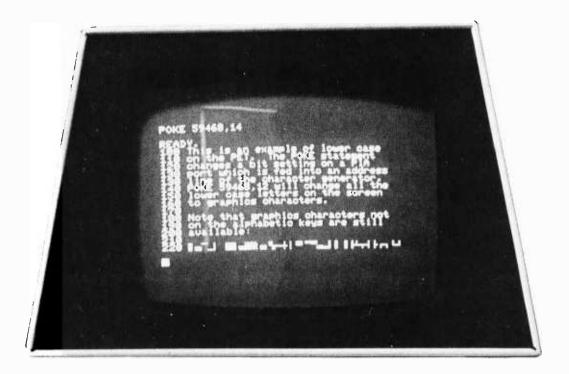
Photo 4: An illustration of upper and lower case letters on the PET. 26 of the 64 graphics characters can be exchanged for lower case letters by altering an address line on the character generator read only memory.
