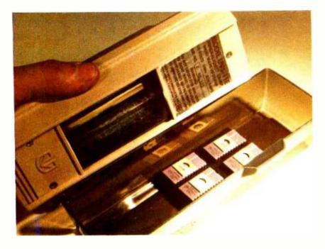
Photo 3: An Ultra Violet Products UVS-IIE ultraviolet eraser for 2708s and similar erasable read only memories. This unit can hold four circuits at a time on conductive foam inside the tray.
