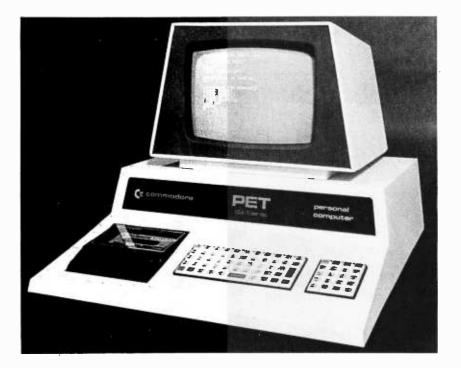
Photo 1: A view of the Commodore PET, Model 2001. This personal computer sells for \$595 and includes a keyboard, video display, cassette drive, 4 K bytes of programmable memory, and a BASIC interpreter and operating system in 14 K bytes of read only memory.
