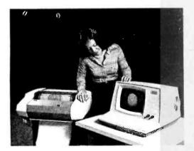
A video graphic display and matching printer with plotting capabilities are now available for the Wang 2200 series computers. The 2282 Graphics CRT has a 12 inch (30.5 cm) diagonal screen with 800 by 512 addressable dots. Vectors are generated by turning on a series of dots approximating a line. The 2231W-3 printer provides an accurate hard copy of a graphics image by printing strips of
