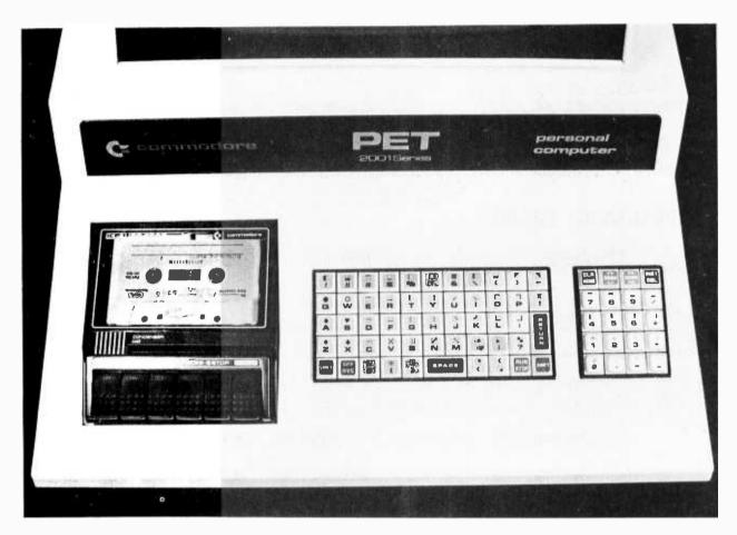
Photo 2: A close-up of the PET keyboard and cassette drive. The keyboard is a flat, calculator style unit with 73 keys. The upper case shift positions on 64 of the keys are occupied by graphic characters. At the right are the cursor control and insert/delete keys and a numeric keypad.
