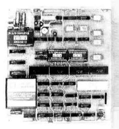
Signal Laboratories Inc, 202 N State College Blvd, Orange CA 92668, is making available a new analog IO card. With this board, intended for use with the Zilog Z-80 development systems, the engineer or scientist can monitor up to 16 analog channels in real time.
