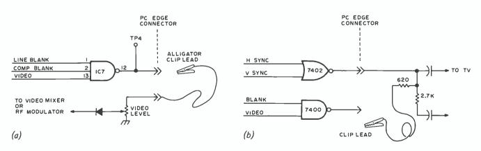
Figure 2: (a) A modification of the Gantt televison display circuit, of page 18, June 1976 BYTE, to use this test instrument technique. The line from IC7 pin 12 to the video level potentiometer is broken so that input to the video mixer, and thus to the TV, is taken from some arbitrary point under test rather than the usual source. (b) The author's video output circuitry, with a similar clip lead jumper normally in place for display purposes, but free to be moved around for testing purposes.
