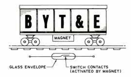
Figure 6: This is a magnetic reed switch which can be used as a marker along the track. The switch consists of two contacts that are enclosed within a glass envelope The two metal contact are activated magnetically when a car with a magnet attached passes over.
