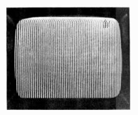
Photo 4: Looking at a single dot position. When the alligator clip is moved to point 3 on figure 1, this pattern is produced. Each character has seven horizontal dot positions, of which two are inactive spacing positions, and five are used for character generation.
