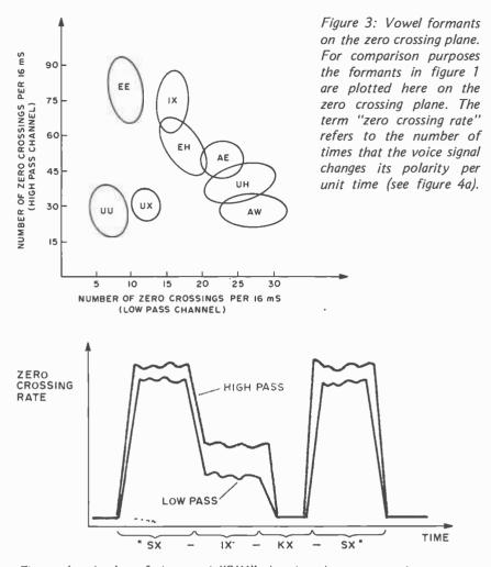
Figure 4a: A plot of the word "SIX" showing the zero crossing rate as a function of time. The word is shown split into its four phonemes. In this case, the signal is first processed through two bandpass filters. The number of zero crossings is then determined by the computer. Results for both filters are shown. As the graph indicates, there is a very short period of silence during the pronunciation of the KX phoneme which can be verified by slowly pronouncing the word "six."
