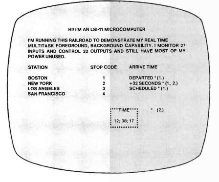
Figure 3: A typeset example of the type of display generated by the authors<sup>\*</sup> terminal. Such pertinent train information as arrival times and estimated delays is available to the operator. "Arrival Time" messages vary between "ARRIVED," "DEPARTED," "+XX SECONDS," "DELAYED," "NEXT STOP," and "SCHEDULED."
