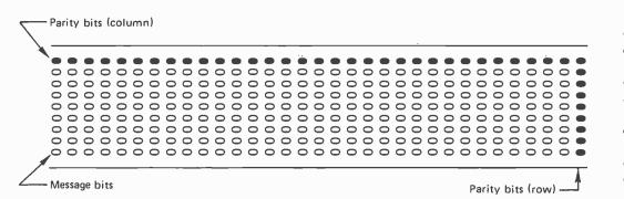
wrong one. If we could tell that, then we could correct the error, because if a bit is "one," and it is wrong, then it must really be "zero," and vice versa. Knowing which bit is wrong is what enables us to do error correction.
