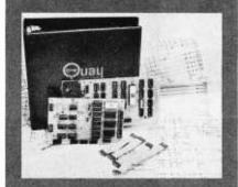
This dynamite new microcomputer system in a kit moves data like nothing else on the market. Run it alone or plug it into an \$100 bus Altair/IMSAI. For sola performance, all you need is an unregulated power supply and an I/O device. Plugged in, Quay 80AI is a CPU, ROM, SIO, and RAM board—run any \$100 compatible device. BUT MORE THAN THAT. Quay 80AI's Z-80 CPU opens challenging new areas of personal computing.
