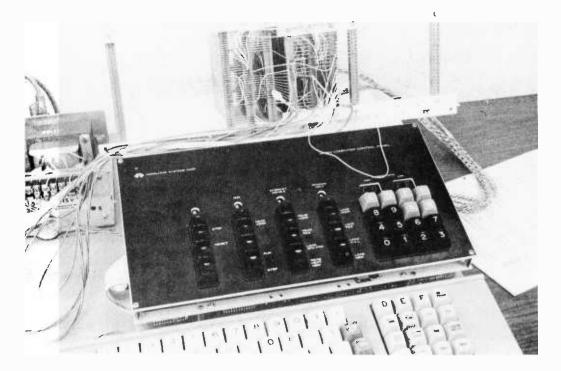
Photo 7: Physical layout of the equipment. The author's display is shown here as it was built on prototyping cards with a bus wired backplane between connectors. The clip lead is shown here attached to memory address bit 7, as used to generate photo 3. The computer and keyboard are in the foreground. correspond correctly, and that data is written correctly. (Of course, we could just as well have put some message on the display, too.)
