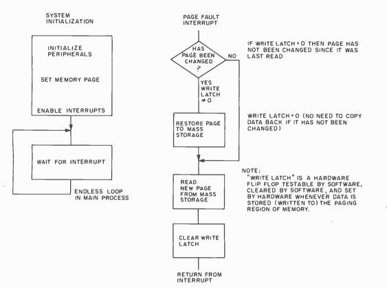
Figure 3: What to do when a page fault occurs. This is a simplified flow diagram of a virtual memory system control process, including initialization and response to a page fault interrupt. It is assumed to be running in a microprocessor dedicated to memory management.
