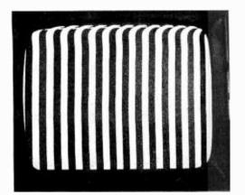
Photo 2: Exploring the circuit with the probing alligator clip produces various interesting signals. Here the clip looks at address bit 1, point 1 on figure 1. This signal changes state every other character position, giving vertical bars two character widths wide. Note the distortion at the top of the image, not normally seen due to blanking of the display.
