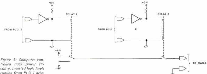
trolled track power circuitry. Inverted logic levels coming from PLU 1 drive two types of relays. The first type (represented by relay 1 in this illustration) chooses the polarity of the voltage going to the track, while the second type (relay 2 here) applies power to the track. Only certain strategic areas of the track require polarity switching.
