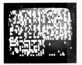
Photo 6: A map of the preferred states of one memory chip. By tapping into just one of the memory data lines with the display probe, it is possible to generate a map of the data. This data is identical to that of photo 5, but we are now looking directly at one bit, instead of generating characters from 8 bit byte groupings of several chips. This same technique of looking at one bit can be done with normal programmed displays, too, rather than the turn on pattern used here.
