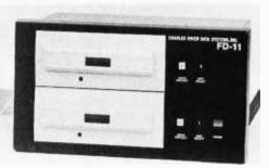
software and media compatible with the DEC RX11 products. It includes write protect switches, unit select switches, up to four drives with one unit load on the DEC Unibus, PROM self-diagnostic programs and bootstrap loader. Track to track access time is 6 ms. Single quantity price of the drive and DEC compatible controller is \$2750.=
