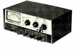
b. A laboratory bench power supply. Once built, this instrument is used to simultaneously power logic (+5 V) and provide variable metered analog levels from  $\pm 0$  to  $\pm 20~V$ .
