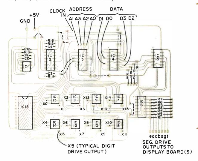
easily be used to replace the binary lights on a computer as an octal display. This display board is also a handy readout for any number of homebrewed instruments.
