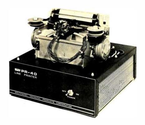
Photo 1: The PR-40 dot matrix printer as assembled from the kit distributed by Southwest Technical Products. The printer is not enclosed in a case but is mounted on a black anodized aluminum chassis with overall dimensions of 9.63 by 10.50 by 8.75 inches (24.45 cm by 26.67 cm by 22.23 cm).
