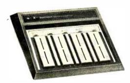
a. A prototyping breadboard. In computer applications, such a breadboard can be used to temporarily try out a circuit before committing it to permanent form using wires, sockets, Vectorboard and solder or wire wrap. Power supplies at standard logic  $(\pm 5\ V)$  and typical analog  $(\pm 12\ V)$  levels aid prototyping with this unit.
