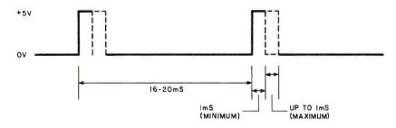
Figure 1: Timing diagram of the waveform that is needed to drive the servomechanism. The pulses are from 16 to 20 ms apart in time, and have a pulse width of 1 to 2 ms. This type of timing can be accomplished using your computer's internal clock as a reference in timing loops, or through a programmable real time clock.
