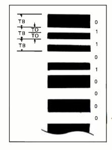
If we assume, in each of these formats, that the short spaces and bars are half the width of the long spaces and bars, and that 50 bits per inch is a reasonable density for format 2, we can calculate the corresponding densities for the other formats:
