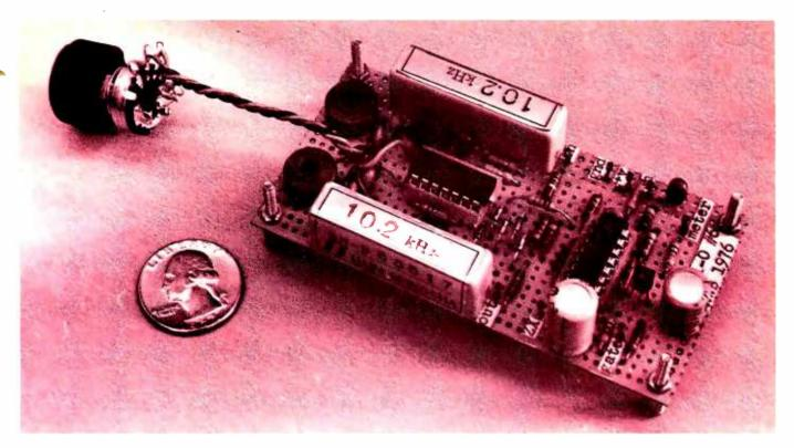
Photo 3: Mechanical filter front end board. This picture details the construction of the mechanical filter front end for the Mini-O receiver, described by the circuit diagram of figure 2. The potentiometer hanging loose at the left is the 1 k RF gain potentiometer, R1 in figure 2. The board shown here also includes the zero crossing detector of figure 3, at the right.
