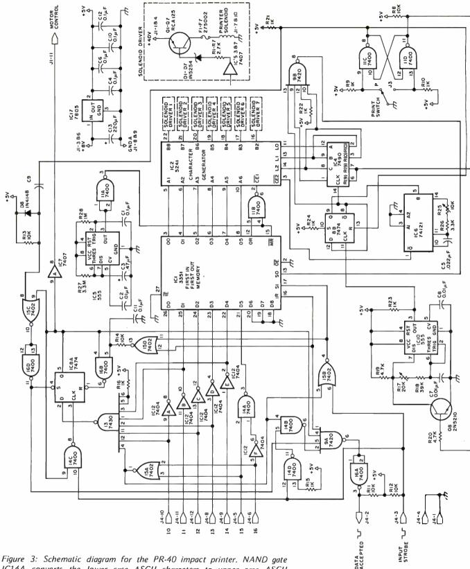
Figure 3: Schematic diagram for the PR-40 impact printer. NAND gate IC14A converts the lower case ASCII characters to upper case ASCII characters. The printer outputs a line of data at a time. The data is output when a carriage return is received or 40 characters have been entered into the memory buffer. All ASCII control characters, except carriage return, are ignored since they are not printed anyway. All resistors in this circuit are measured in ohms and are 0.25 W.
