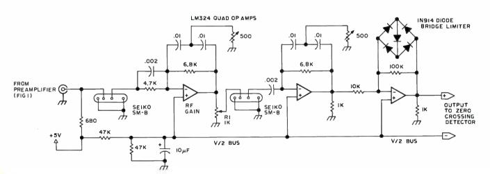
Figure 2: Mini-O mechanical filter front end amplifiers. This active circuit uses two mechanical filters manufactured by Seiko to provide a narrow bandwidth of 14 Hz at the -3 dB points and a gain of 40 to 60 dB. The output passes through a diode bridge limiter implemented with an operational amplifier section, prior to reaching the zero crossing detector of figure 3. The physical construction of this circuit is shown in photo 3.
