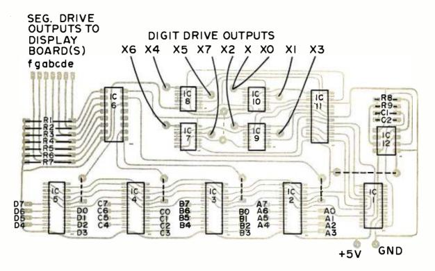
the counter will be disabled and the address on the counter inputs will appear at the outputs addressing the memory. IC2 provides a 60 ns delay, then a 60 ns pulse which writes the data at the memory data inputs into the memory location addressed. When the clock line returns to the high state, the counter will resume counting. The counter sequentially addresses the BCD data stored in the memory while it selects and enables the appropriate digit in the display.
