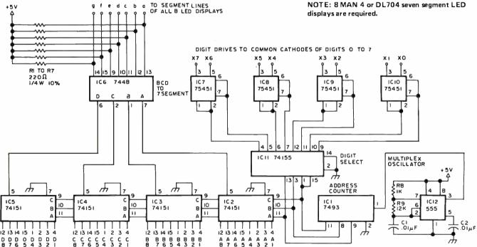
power configuration uses one 7 segment driver for each 7 segment LED in the display. Constant power is supplied to all digits. The multiplexed configuration uses only one 7 segment driver for several digits. Power is supplied to only one digit at a time, but is switched at a high rate so all digits appear to be on constantly. Since only one digit is powered at any given time, a certain amount of power is saved. This principle is widely used in electronic calculators.
