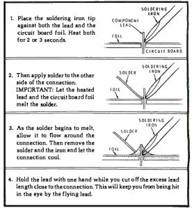
Be sure the solder made a good electrical connection. When both the lead <u>and</u> the circuit board foil are heated at the same time, the solder will flow onto the lead and the foil evenly. See Illustration A. The solder will then make a good electrical connection between the lead and the foil.
