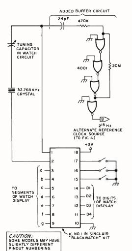
Figure 6: Use of the Sinclair "Blackwatch" wristwatch kit as a source of the 2<sup>15</sup> Hz reference signal (32.768 kHz). This circuit was used by the author to provide both chronometer functions and Omega reference timing by mounting it in a plastic case so that the LEDs could be seen (see photo 2).
