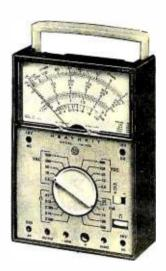
c. A multimeter. This all around useful test instrument can be built from a kit and later used to measure miscellaneous voltages, current and resistance when diagnosing or using the hardware of a computer and its interfaces.
