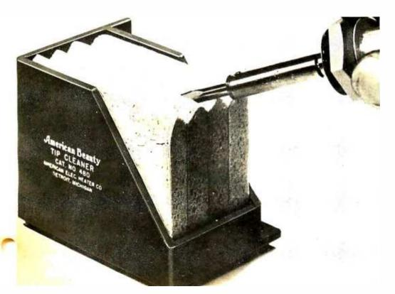
Key 2: One key to good soldering is a clean soldering itp. There are several different brands of wet sponges like this one, which can be used to clean the tip during use. Many of these products are treated with special chemicals to help improve the cleaning properties.
