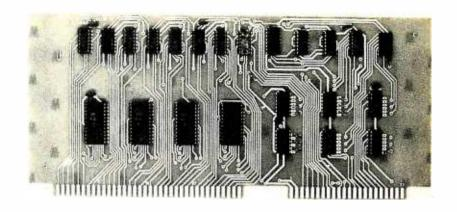
Photo 4: The author's Digital Group System IO card. This card interfaces to the system's bus, providing four parallel output ports and four input ports. These ports are routed to the backplane where they communicate to the video display, keyboard and cassette interfaces.
