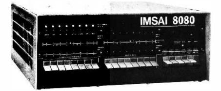
memory and IO interface devices. The heavy duty lucite front panel has an extra 8 program controlled LEDs as well as rugged commercial grade paddle switches backed up by reliable debouncing circuits. The IMSAI 8080 power supply has a steady state 20 Amp current capacity, enough to power a full system.
