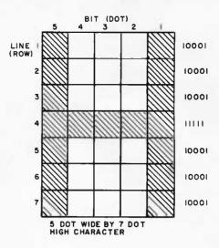
Figure 3: An example of a dot matrix pattern generated by the television display.
