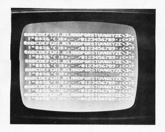
Photo 1: This is a test display pattern generated by connecting the low order outputs of the character and line counters to the character generator ROM's 6 input bits. The result presents every combination of the character set, so every character pattern is visible on the screen.
