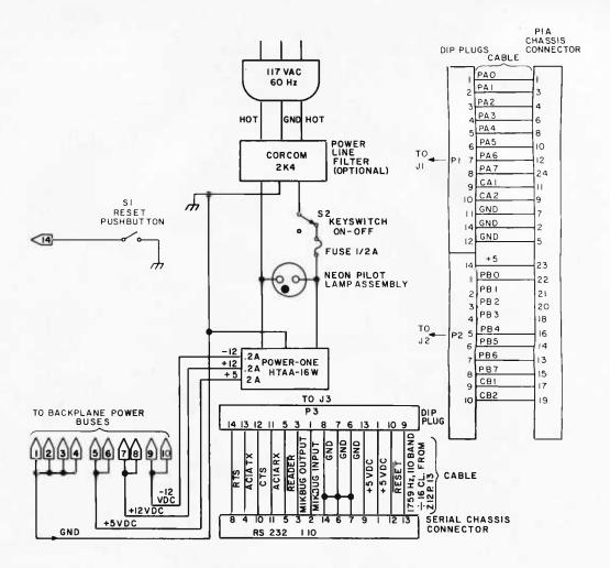
Figure 4: Power Supply, Interconnection Cables and Reset Switch.
