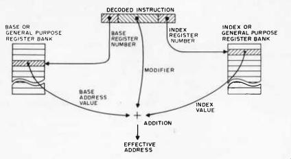
Figure 5: Combining Two Index Registers. A more general address calculation uses one register as a base register, a second register as an index register, and a modifier. The effective address is then the sum of the values found in the two registers and the value of the modifier. The order of calculation and detailed significance of the registers depends upon the processor design which uses this type of address calculation.
