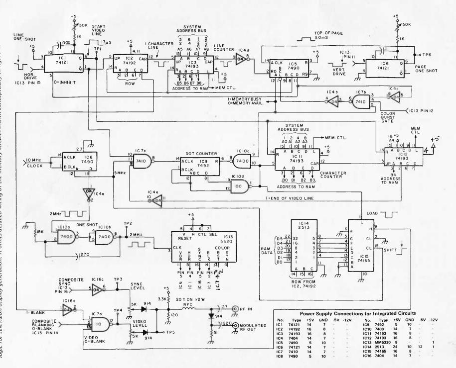
that the TVD generates two identical interlaced frames to make a complete picture. The result is that each character is actually 14 lines high.
