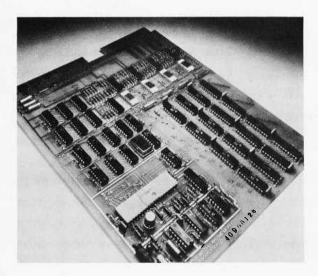
A new option in the high performance 16 bit microcomputer field has now arrived on the scene. This is the Data General micro-NOVA, introduced early in March as BYTE's June issue went to the press. Here is another instance of a widely available minicomputer architecture being made available in the form of a relatively inexpensive microcomputer.
