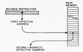
Figure 8: Indirect Addressing. In this form of addressing, the first effective address developed is used to address memory to find a pointer which will become the final effective address used for the instruction.
