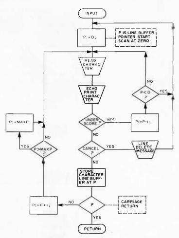
Figure 4: The Input Subroutine Specified as a Flow Chart. The main purpose of INPUT is to read one line of input, terminated by a carriage return. INPUT implements the line editing functions of character delete and line delete. When the carriage return code is detected, the line buffer LB is filled from position 0 to position P.
